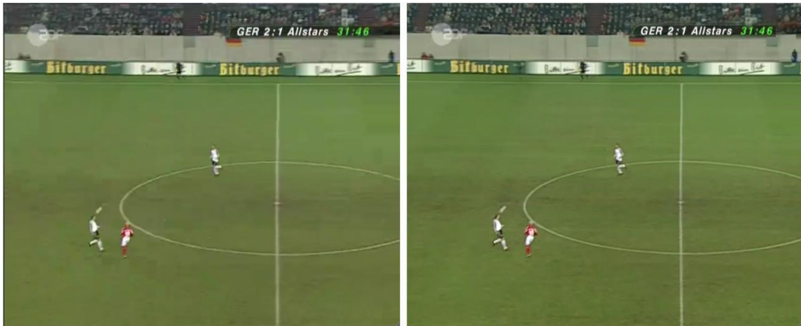
(a) Frame 24, (H.264/AVC, PSNR = 36.01 dB, SSIM = 0.93) (b) Frame 24, (OBVC, PSNR = 34.54 dB, SSIM = 0.94)
