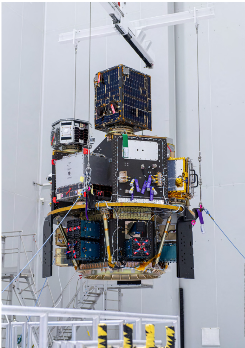
Figure 2.1: Small satellites mounted on Vega's Small Spacecraft Mission Service (SSMS). At the lower end one can see several 12 U CubeSat dispensers mounted to the adapter, while the larger satellites on the upper deck make use of traditional separation systems (Image credit: ESA/CNES/Arianespace/Optique Video du CSG - JM Guillon).
