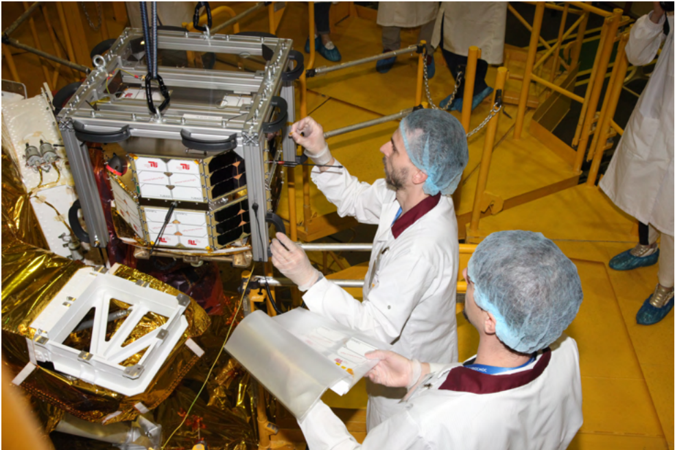
Figure 4.2: Integration of the TechnoSat spacecraft onto the upper stage of the Soyuz launcher one week before launch [244] (Image credit: Roscosmos).
