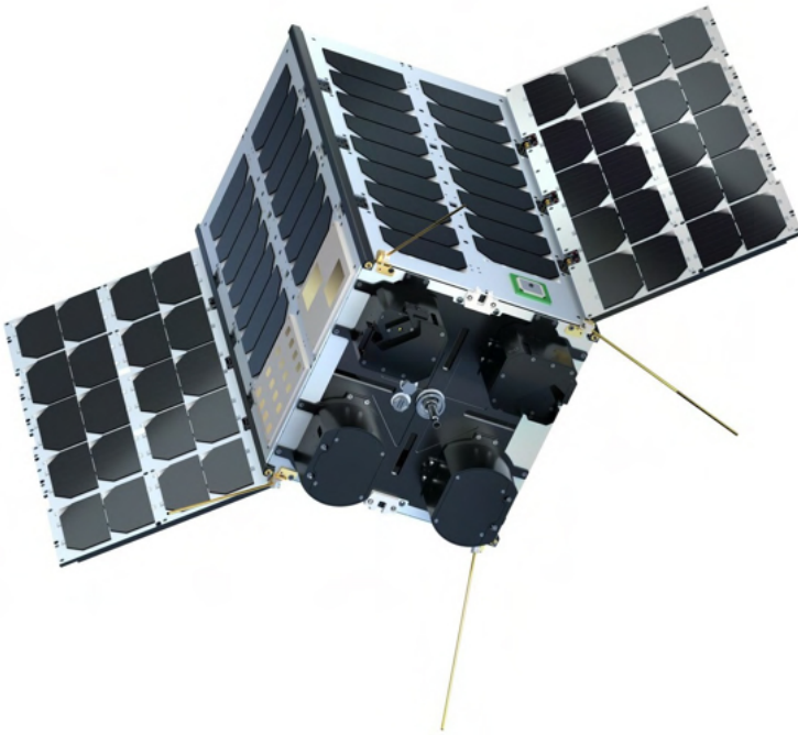
Figure 2.6: M16P 16 U microsatellite platform developed by NanoAvionics in flight configuration (Image credit: NanoAvionics).
