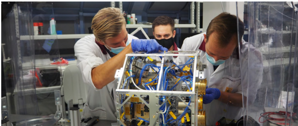
Figure 4.33: Integration of the engineering qualification model of TUBIN in a laminar flow box in the small satellite integration laboratory of Technische Universität Berlin. At this point only the solar panels on the sides of the spacecraft are missing for concluding the integration (Image credit: Philipp Werner).
