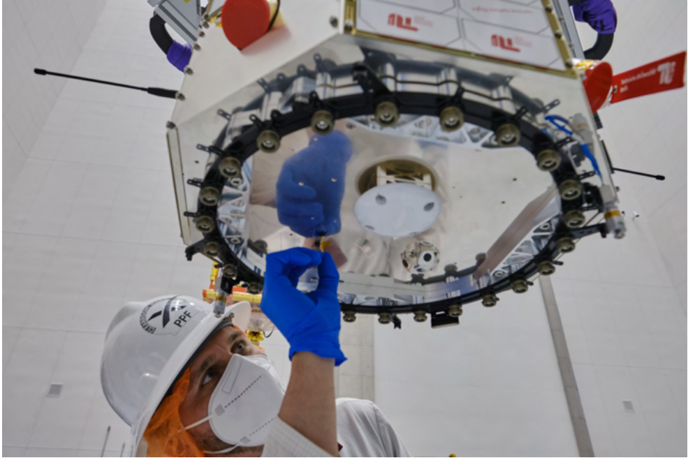
Figure 4.34: Removal of the RBF items in the bottom of the spacecraft right before it is mounted to the adapter to the ESPA ring of the Falcon 9 launcher at Cape Canaveral (Image credit: Mario Starke).
