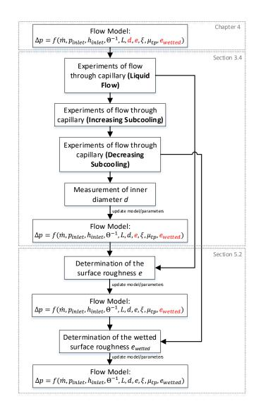
**Fig. 5.10:** Systematic approach for the generation of an experimental database on the refrigerant flow in a capillary and the parametrization of the according flow model based on previous investigations and a partly parametrized flow model of the same refrigerant in a different capillary tube with the same geometry specifications.
