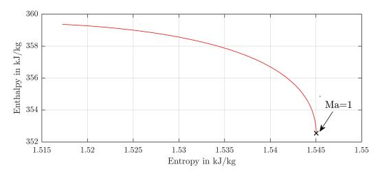
Fig. 2.3: Exemplary Fanno line for an exemplary two-phase refrigerant flow subject to friction.
