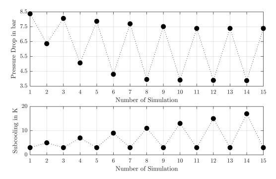
*Fig.* 5.14: Simulated hysteresis effect on the pressure drop evoked by the alternation of the subcooling at a constant inlet pressure of 16 bar and mass flow of 15 kg/h using the flow model in chapter 4 and the parametrization in Tab. 5.4. The horizontal axis displays the number of simulation, i.e. indicates a new flow condition (change of the subcooling).
