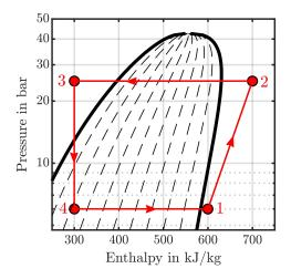
*Fig. 2.2: Exemplary simplified and idealized heat pump process in the p,h-diagram of propane.*
