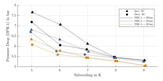
**Fig. 3.6:** Experimental results of the measurement series including the increasing (Incr.) and decreasing (Decr.) subcooling path at a constant mass flow (FIRC-1) of 16.5 kg/h and different inlet pressures (PRC-1) in the copper capillary tube depicting the resulting pressure drop (DPR-1) over the change of the subcooling at the capillary inlet (mean values of the redundant measurements).
