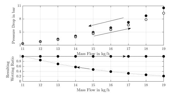
*Fig.* 5.15: Simulated hysteresis on the pressure drop evoked by the change of the mass flow from high mass flow to low mass flow to high mass flow at a constant inlet pressure of 25 bar and constant subcooling of 5 K using the flow model in chapter 4 and the parametrization in Tab. 5.4.
