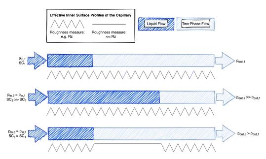
*Fig. 4.1:* Effective roughness of the inner surface of the capillary depending on the wetting ratio of the capillary tube (source: (Gabrisch and Repke, 2021)).
