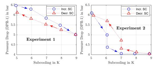
*Fig.* 3.11: *Left*: Performing increasing (Incr.) and decreasing (Decr.) subcooling paths *without flushing*; *Right*: Performing increasing and decreasing subcooling paths *with flushing*. Both at 15 bar inlet pressure (PRC-1) and a mass flow (FIRC-1) of 16 kg/h in the copper capillary depicting the resulting pressure drop (DPR-1) over the change of the subcooling at the capillary inlet (source: (Gabrisch and Repke, 2021)).
