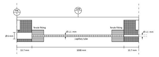
*Fig. 3.3:* Dimensions of the capillary tube and distances of pressure taps to inlet and outlet of the capillary tube.
