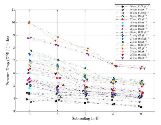
**Fig. A.1:** Diagram of all experimentally gathered increasing subcooling paths in Tab. A.2 in the copper capillary. The legend shows the different investigated inlet pressures (PRC-1) and the mass flows (FIRC-1). The diagram shows the resulting pressure drop (DPR-1) over the change of the subcooling at the capillary inlet, source: (Gabrisch and Repke, 2020).
