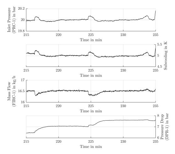
*Fig. 3.8:* Extracted time-resolved measurement of the measurement series at a constant inlet pressure (PRC-1) of 20 bar and a mass flow (FIRC-1) of 16.5 kg/h in the copper capillary tube further displaying the subcooling at the capillary inlet and the pressure drop (DPR-1) showing a collapse of a metastable flow (increase in pressure drop).
