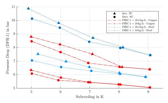
*Fig.* 3.16: Comparison of the characteristics of the hysteresis curves including the increasing (Incr.) and decreasing (Decr.) subcooling path at different mass flows (FIRC-1) for an inlet pressure (PRC-1) of 25 bar referring to the experiments in the copper and steel capillary. The diagram shows the resulting pressure drop (DPR-1) over the change of the subcooling at the capillary inlet.
