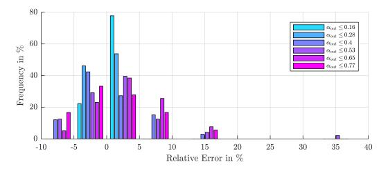
**Fig. D.3:** Histogram of the deviation of the predicted pressure drops from the measured pressure drops (DPR-1) for the decreasing subcooling paths applying the modified B&W viscosity correlation and the parametrization:  $e = Rz_{Copper} = 1.285e-6 m$ ,  $\xi_{Rz} = 2.3475$ ,  $\psi_{Rz} = 6.1714$  and  $e_{wetted,Rz,Copper} = 3.5906e-10 m$  (classified by the predicted void fraction  $\alpha_{out}$  at the outlet of the capillary).
