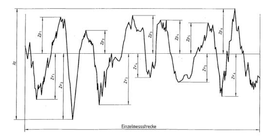
Fig. 3.14: Illustration of the average roughness depth Rz (source: DIN EN ISO 4287).
