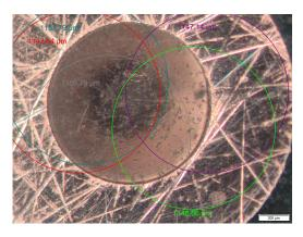
*Fig. B.1:* Exemplary measurements of the inner diameter of a test sample (D-1) under the light microscope.
