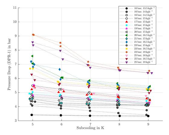
*Fig. A.2:* Diagram of all experimentally gathered decreasing subcooling paths in Tab. A.3 in the copper capillary. The legend shows the different investigated inlet pressures (PRC-1) and the mass flows (FIRC-1). The diagram shows the resulting pressure drop (DPR-1) over the change of the subcooling at the capillary inlet, source: (Gabrisch and Repke, 2021).
