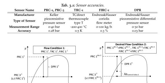
Fig. 3.2: Limit of the mass flow control in the experimental apparatus.
