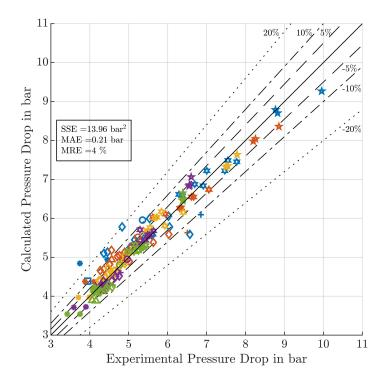
*Fig.* 5.6: Comparison between the experimental pressure drops (DPR-1) of the increasing subcooling paths and the predicted pressure drops in the copper capillary using the modified B&W viscosity correlation in Eq. (5.6) and the parametrization:  $e=Rz_{Copper}=1.285e-6 m$ ,  $\xi_{Rz}=2.3475$  and the estimated  $\psi_{Rz}=6.1714$  (source: (Gabrisch and Repke, 2020)).
