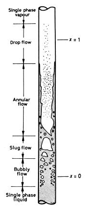
Fig. 2.6: Flow patterns in a vertical evaporator tube (Source: (Collier and Thome, 1994a)).
