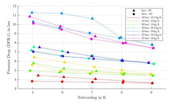
**Fig. 3.15:** Experimental results of the measurements series in Tab. 3.6 in the steel capillary tube comprising all increasing (Incr.) and decreasing (Decr.) subcooling paths. The legend displays the measurements at different inlet pressures (PRC-1) and different mass flows (FIRC-1). The diagram shows the resulting pressure drop (DPR-1) over the change of the subcooling at the capillary inlet (mean values of the redundant measurements).
