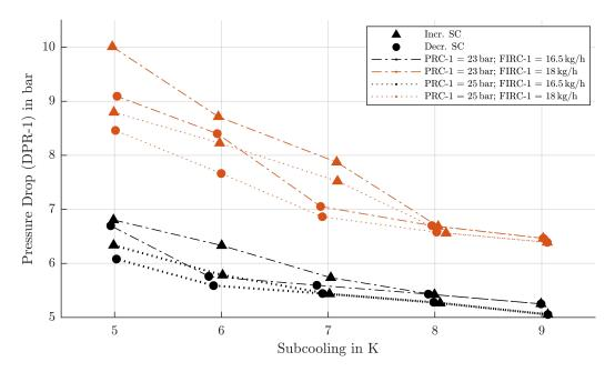
**Fig. 3.9:** Comparison of the characteristics of the hysteresis curves including the increasing (Incr.) and decreasing (Decr.) subcooling path at mass flows (FIRC-1) of 16.5 and 18 kg/h and inlet pressures (PRC-1) of 23 and 25 bar in the copper capillary depicting the resulting pressure drop (DPR-1) over the change of the subcooling at the capillary inlet (mean values of the redundant measurements).
