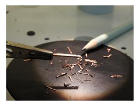
*Fig. B.2:* Preparation of half-pipes of the capillary test samples for the investigation of the roughness of the inner surface.
