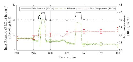
**Fig. 3.10:** Representative extract from the time-resolved recordings of the propane flow conditions at the inlet of the copper capillary - flushing the capillary by increasing the inlet pressure (PRC-1). Showing the inlet pressure (PRC-1), the subcooling and the temperature (TRC-1) at the capillary inlet (source: (Gabrisch and Repke, 2021)).
