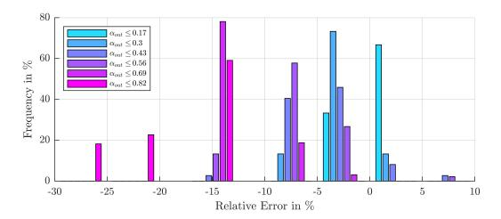
**Fig. D.1:** Histogram of the deviation of the predicted pressure drops from the measured pressure drops (DPR-1) in the copper capillary for the increasing subcooling paths applying the viscosity correlation of Beattie and Whalley (1982) and the parametrization:  $e=Rz_{Copper}=1.285e-6m$ ,  $\xi_{Rz}=2.3475$  and  $\psi_{Rz}=6.1714$ .
