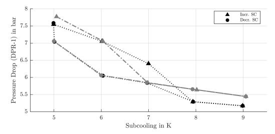
*Fig.* 3.7: Experimental results of two redundant measurement series including the increasing (Incr.) and decreasing (Decr.) subcooling path at the constant inlet pressure (PRC-1) of 20 bar and mass flow (FIRC-1) of 16.5 kg/h in the copper capillary tube depicting the resulting pressure drop (DPR-1) over the change of the subcooling at the capillary inlet.
