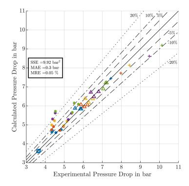
*Fig.* **5.13**: Comparison between the experimental pressure drops (DPR-1) of the decreasing subcooling paths and the predicted pressure drops in the steel capillary using the modified B&W viscosity correlation with the parameters in Tab. 5.7.
