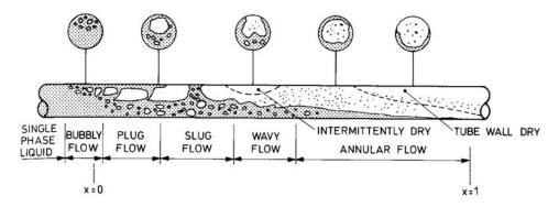
*Fig.* 2.5: *Two-phase flow patterns in horizontal tubes (evaporation) (Source: (Collier and Thome, 1994a)).*
