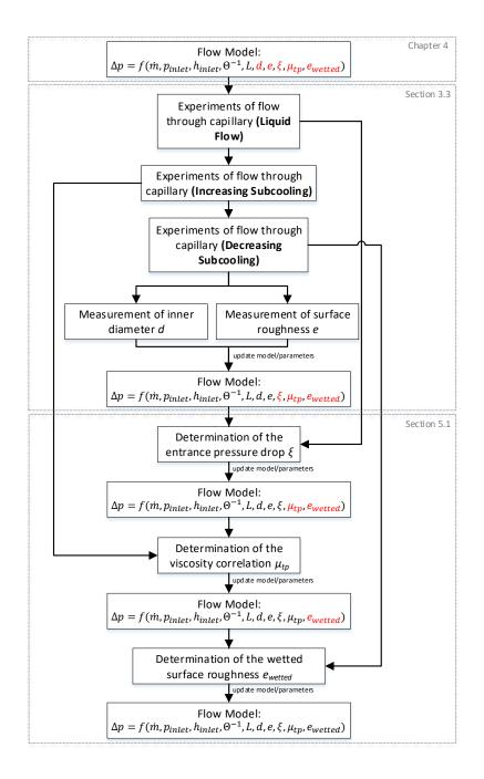
*Fig.* 5.1: Systematic approach for the generation of an experimental database on the refrigerant flow in a capillary and the parametrization of the according flow model.
