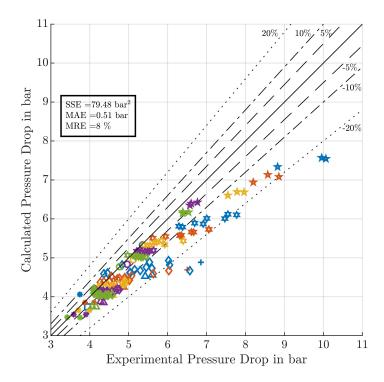
*Fig.* 5.3: Comparison between the experimental pressure drops (DPR-1) of the increasing subcooling paths and the predicted pressure drops in the copper capillary using the viscosity correlation provided by Beattie and Whalley (1982) and the parametrization:  $e=Rz_{Copper}$  = 1.285e-6 m and  $\xi_{Rz}$  = 2.3475 (source: (Gabrisch and Repke, 2020)).
