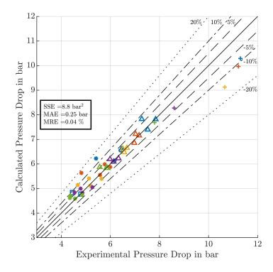
*Fig.* 5.12: Comparison between the experimental pressure drops (DPR-1) of the increasing subcooling paths and the predicted pressure drops in the steel capillary using the modified B&W viscosity correlation in Eq. (5.6) with the parameters in Tab. 5.7 and  $e_{wetted,Steel}=Rz_{Steel}$  = 2.239e-6 m.
