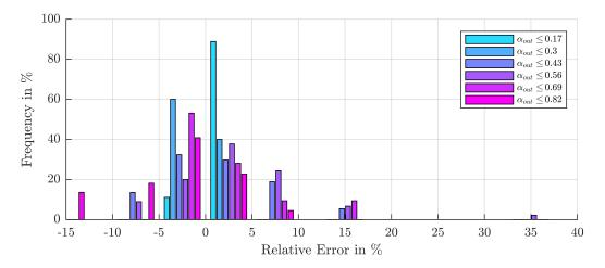
**Fig. D.2:** Histogram of the deviation of the predicted pressure drops from the measured pressure drops (DPR-1) in the copper capillary for the increasing subcooling paths applying the modified B&W viscosity correlation and the parametrization:  $e=Rz_{Copper}=1.285e-6 m$ ,  $\xi_{Rz}=2.3475$  and  $\psi_{Rz}=6.1714$ .
