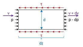
*Fig. 2.4:* Schematic flow through a discretized length of a tube  $\Delta L$ .
