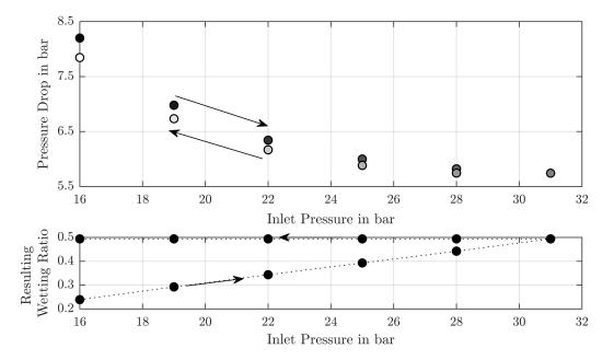
*Fig.* **5.16**: Simulated hysteresis on the pressure drop evoked by the change of the inlet pressure from low inlet pressure to high inlet pressure to low inlet pressure at a constant mass flow of 16 kg/h and constant subcooling of 5 K using the flow model in chapter 4 and the parametrization in Tab. 5.4.
