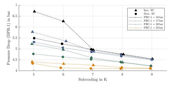
**Fig. 3.5:** Experimental results of the measurement series including the increasing (Incr.) and decreasing (Decr.) subcooling path at a constant mass (FIRC-1) flow of 15 kg/h and different inlet pressures (PRC-1) in the copper capillary tube depicting the resulting pressure drop (DPR-1) over the change of the subcooling at the capillary inlet (mean values of the redundant measurements).
