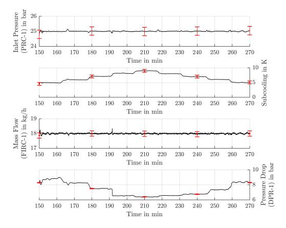
**Fig. 3.4:** Exemplary time-resolved measurement series at a constant inlet pressure (PRC-1) of 25 bar and a mass flow (FIRC-1) of 18 kg/h further displaying the change of subcooling at the capillary inlet and the resulting pressure drop (DPR-1).
