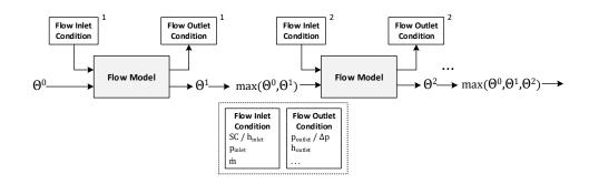
*Fig. 4.2:* Calculation scheme of a transient simulation of the flow model for a series of flow conditions.
