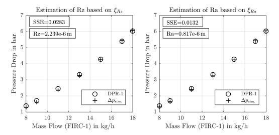
**Fig. 5.11:** Estimation of the average roughness depth Rz and the average roughness value Ra of the steel capillary given the entrance pressure drop coefficients  $\xi_{Rz}$  and  $\xi_{Ra}$ . The diagram shows the resulting experimental pressure drop (DPR-1) vs. the simulated pressure drop ( $\Delta p_{sim.}$ ) over the different measured mass flows (FIRC-1), see data in Tab. A.4. It further shows the resulting sum of square errors (SSE) and the resulting roughness measures Rz and Ra.
