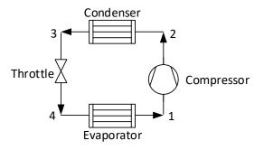
Fig. 2.1: Basic components of the heat pump process.
