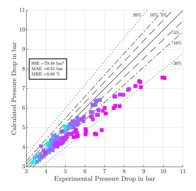
**Fig. 5.4:** Comparison between the experimental pressure drops (DPR-1) of the increasing subcooling paths and the predicted pressure drops in the copper capillary using the viscosity correlation provided by Beattie and Whalley (1982) and the parametrization of e with  $Rz_{Copper}=1.285e-6$  m and  $\xi_{Rz}=2.3475$  (classified by the predicted void fraction  $\alpha_{out}$  at the outlet of the capillary).
