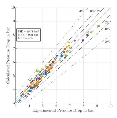
**Fig. 5.7:** Comparison between the experimental pressure drops (DPR-1) of all measurement series and the predicted pressure drops in the copper capillary applying the modified B&W viscosity correlation in Eq. (5.6) with the following parametrization:  $e = Rz_{Copper} =$ 1.285e-6 m,  $\xi_{Rz} = 2.3475$ ,  $\psi_{Rz} = 6.1714$  and  $e_{wetted,Rz,Copper} = 3.5906e$ -10 m (source: (Gabrisch and Repke, 2021)).
