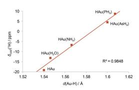
**Figure 6.** Correlation between hydride <sup>1</sup>H NMR shift and Au–H bond length in the selected neutral HAuL complexes (see Table S1 for numerical data).
