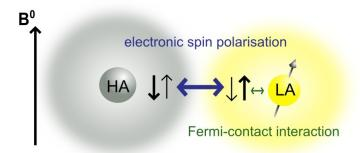
**Figure 6.** Schematic mechanism of the main FC-based HALA effect. The spin-orbit induced spin polarisation of the heavy atom (HA) extends throughout the system to the light atom (LA) affecting its nuclear spin states by hyperfine interactions.
