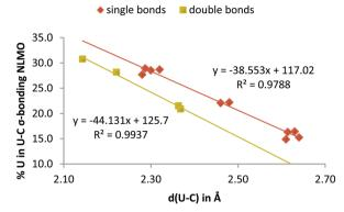
Fig. 7 Correlation between total uranium involvement in the U-C  $\sigma$ -bonding NLMO with U-C bond length, with separate regression lines for U-C single bonds (1-10, red diamonds) and carbene U=C double bonds (11-14, yellow squares). NHC complex 3 has been plotted with the single-bonded species.
