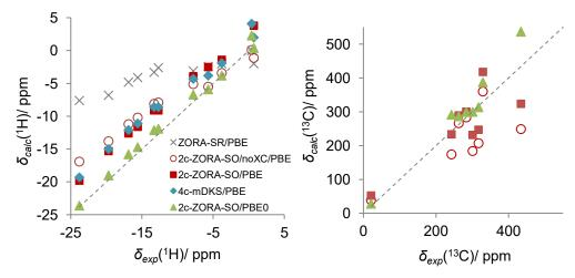
**Figure 7.** Computed vs. experimental NMR shifts (in ppm vs. TMS) for a series of *trans*-[HPtL(PMe<sub>3</sub>)<sub>2</sub>] complexes (left) and for various organometallic U(VI) complexes (right) (adapted from Paper I and Paper III, respectively). The dashed line represents the ideal agreement with experiment.
