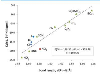
**Figure 2.** Correlation between computed <sup>1</sup>H NMR hydride shifts (2c-ZORA(SO)/PBE0/TZ2P results) and optimized Pt—H bond lengths in *trans*-[HPtL(PMe<sub>3</sub>)<sub>2</sub>] series (cf. Table 1). The dashed line represents the linear-regression line of the values represented by triangles.
