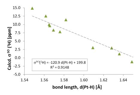
**Figure S3.** Correlation of the SO-induced hydride shielding ( $\sigma^{SO}$ ) within *trans*-[HPtL(PMe<sub>3</sub>)<sub>2</sub>] series with the Pt–H bond length.
