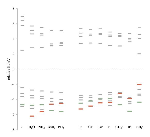
**Figure S1.** Quasirelativistic energies of the frontier MO spinors for the HAuL<sup>q</sup> series (q = 0, -1). The highest occupied  $\pi$ -type spinors with some  $\sigma$  character are highlighted in green, whereas the highest occupied  $\sigma$ -type spinor with significant *trans* ligand character is highlighted in red (2c-ZORA-SO/PBE0/TZ2P results).
