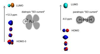
**Figure 10.** Illustration of the predominant  $^1\text{H}$   $\sigma^{\text{p+SO}}$  contributions in HAu and HHgH from two-component spinors (the predominant occupied virtual spinor coupling is in both cases indicated by an arrow), in relation to the direction of SO-induced current loops. Spinors are shown as isosurface plots ( $\pm\,0.03\,$  a.u.).
