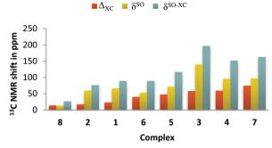
Fig. 3 Total XC-kernel contribution ( $\Delta_{XC} = \delta_{2c}^{xc} - \delta_{2c}$ ) to the calculated <sup>13</sup>C NMR shifts for complexes 1-8 in comparison with the SO shift contributions without ( $\delta^{SO}$ ) and with ( $\delta^{SO-XC}$ ) exchange-correlation kernel at PBE level; ordered by increasing  $\Delta_{XC}$ .
