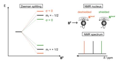
**Figure 4.** Separation of nuclear spin states due to Zeeman splitting for a bare nucleus (black) in comparison with a deshielded (orange) and shielded nucleus (green); the resulting NMR shifts are also indicated.
