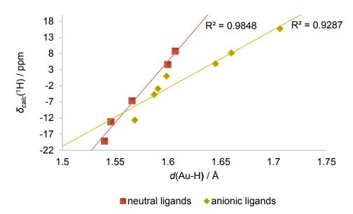
**Figure S2.** Correlation between hydride  ${}^{1}H$  NMR shifts and Au-H bond lengths in the HAuL<sup>q</sup> series (see Table S1 for numerical data), with separate regression lines for neutral (q = 0, red squares) and anionic ligands (q = -1, yellow diamonds).
