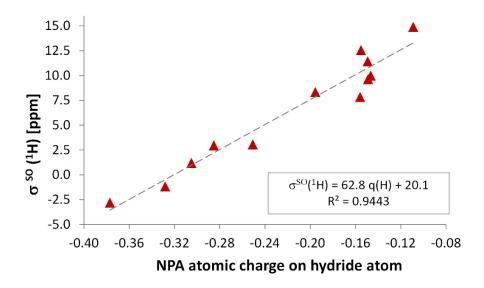
**Figure S4.** Correlation of the SO-induced hydride shielding ( $\sigma^{SO}$ ) within *trans*-[HPtL(PMe<sub>3</sub>)<sub>2</sub>] series with the hydride NPA atomic charge.
