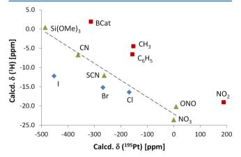
**Figure 7.** Correlation of computed  $^1H$  and  $^{195}Pt$  chemical shifts within the trans-[HPtL(PMe<sub>3</sub>)<sub>2</sub>] series (2c-ZORA(SO)/PBE0/TZ2P results). See data in Tables 1 and 6. The dashed line represents the linear-regression line of the values represented by green triangles.
