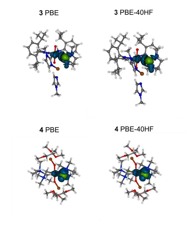
**Figure S1.** Isosurface plots ( $\pm 0.0005$ ) of spin densities induced by a finite Fermi contact perturbation ( $\lambda$ =0.01) for a uranium-bound carbon atom in **3** and **4** with PBE and PBE-40HF functionals, respectively.
