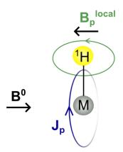
**Figure 5.** Schematic representation of the Buckingham-Stephens effect. A magnetic field perpendicular to the M-H bond produces a paramagnetic ring current inducing a shielding local magnetic field at the off-center position of the hydride.
