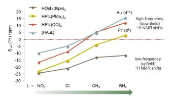
**Figure 1.** Dependence of hydride <sup>1</sup>H shifts (in ppm vs. TMS) on the *trans* ligand effect in widely different sets of d<sup>6</sup> (Os<sup>II</sup>), d<sup>8</sup> (Pt<sup>II</sup>), and d<sup>10</sup> (Au<sup>I</sup>) 5d transition-metal hydride complexes (2c-ZORA-SO/PBE0/TZ2P results; cf. Figure 2 for schematic structures and Table S1 in the Supporting Information for numerical data).
