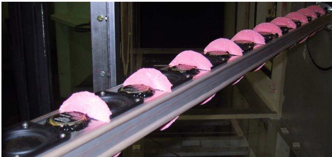
Fig. 2.5: Internal beam holding the actuators, with dividers
