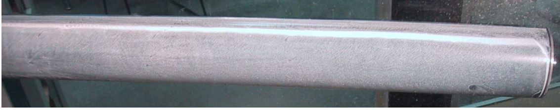
Fig. 4.10: China clay visualization, \Lambda = 64^\circ , Re_n = 35000
