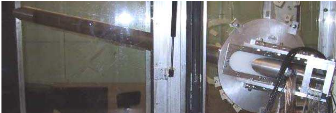
Fig. 2.1: Test section with model and original plexiglass side wall, side view, flow from right
