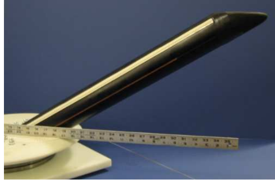
Fig. 2.6: The swiveling cylinder with trip strip, the ruler indicates the horizontal
