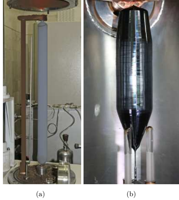
Figure 1.8: (a) Polycrystalline ^{28}\text{Si} rod of in the deposition apparatus; (b) Float-zone grown monocrystalline ^{28}\text{Si} with [001] as growth direction [77, 26].
