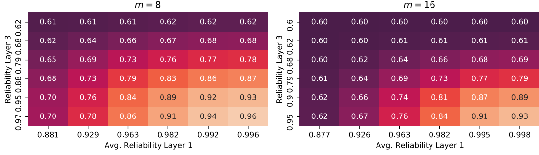
Figure 8.2.3.: Simulated reliability of the 64-bit LP-PUFs depending on reliability of the building blocks.
