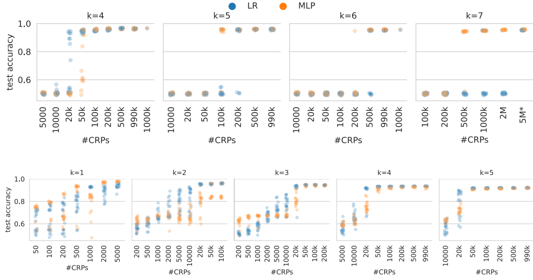
Figure 3.6.2.: Comparison of improved LR attack (Section 3.4) and our MLP attack (Section 3.6.3) on FPGA data from Mursi et al. [Mur+20] (top row) and Aghaie and Moradi [AM21] (bottom row). The results are in line with our results on simulated data: the MLP attack shows lower data complexity for XOR Arbiter PUFs with a large number of XORs k . (*Training set size was actually 4,990,000; 10,000 CRPs were used for testing.)
