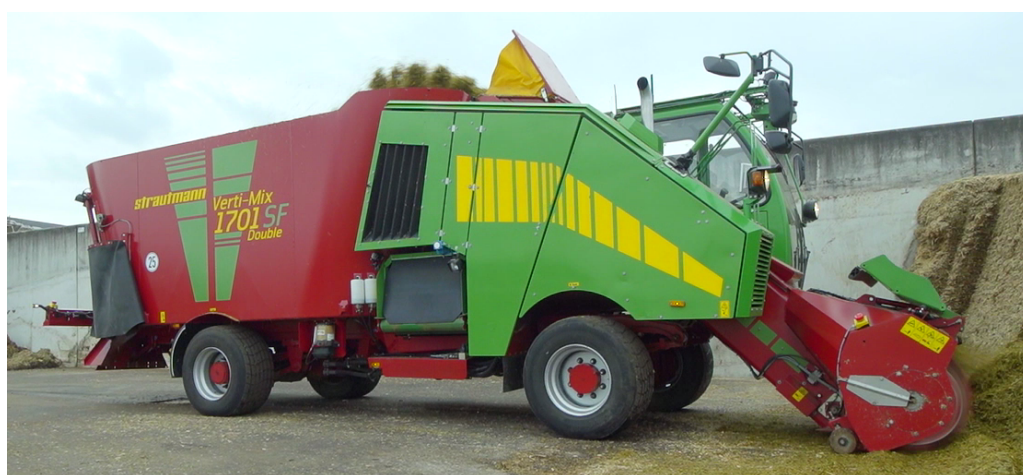
Figure 1. An unmanned feeding mixer is already working with autonomous driving and working functionality. In the developed safety concept, a non-contact sensor system is still missing for the human protection at the autonomous feeding mixer, which may be used both for indoor and outdoor on an agricultural environment.
