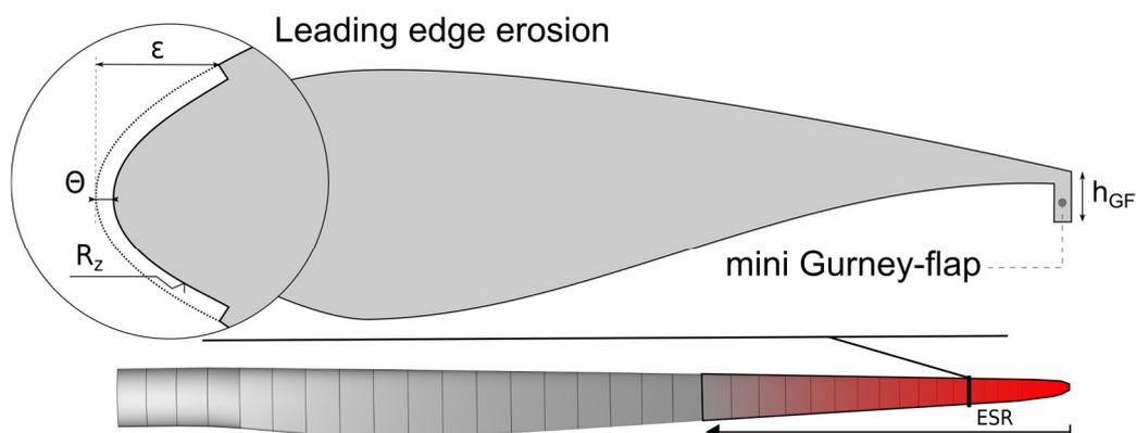
**Figure 1.** Erosion modelling parameters. Example of resulting intensity of erosion-related performance decrease along the blade in red.
