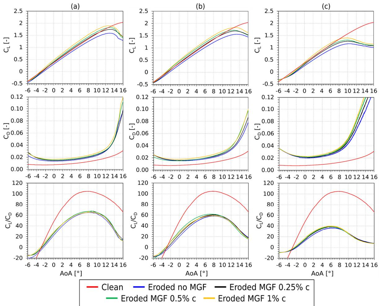
**Figure 4.** Lift, Drag and Lift to Drag ratio characteristics for the three simulated blade sections (FFAW3-241 airfoil at Re number ranging from  $3.5 \cdot 10^6$  to  $14 \cdot 10^6$ ) Column (a): most inner section (section 1). Column (b): intermediate section (section 2). Column (c): most tip section (section 3). Reference undamaged curve is calculated with the same inflow conditions as Section 2.
