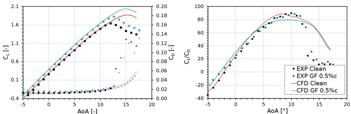
**Figure 3.** Lift, drag and lift-to-drag ratio of CFD airfoil model of DU97-W-300 compared to experimental data from [9] at Reynolds =  $1.5 \cdot 10^6$ .
