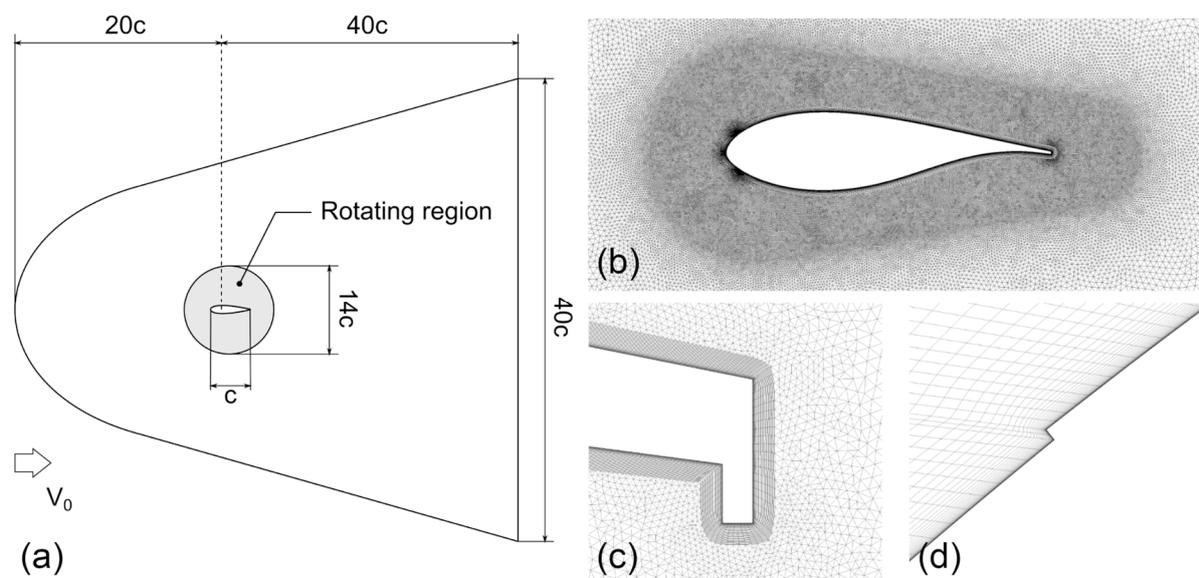
**Figure 2.** Details of the mesh for airfoil simulations: a) computational domain b) airfoil c) MGF d) end of the LE erosion zone.
