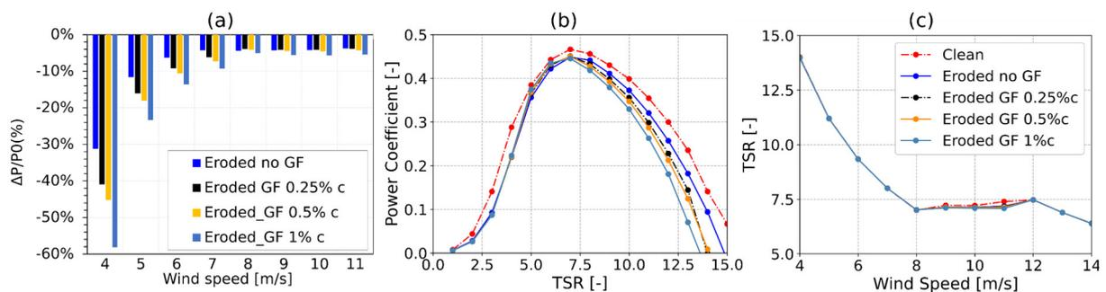
**Figure 5.** Generator power difference relative to undamaged turbine at various wind speeds (left). Power coefficient as a function of tip-speed ratio (right)
