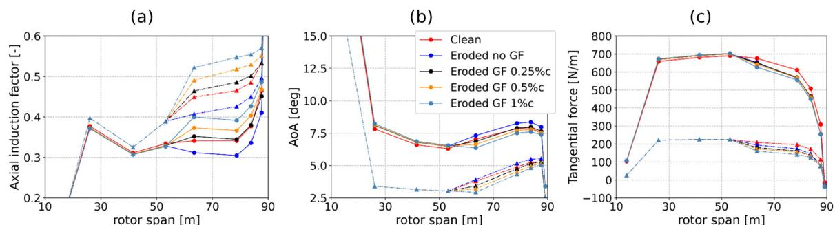
**Figure 6.** Axial induction Factor (a), Angle of attack (b) and tangential force per unit length (c) along the blade span for various MGF heights. Continuous lines for 9m/s wind speed and dashed lines for 6m/s wind speed.
