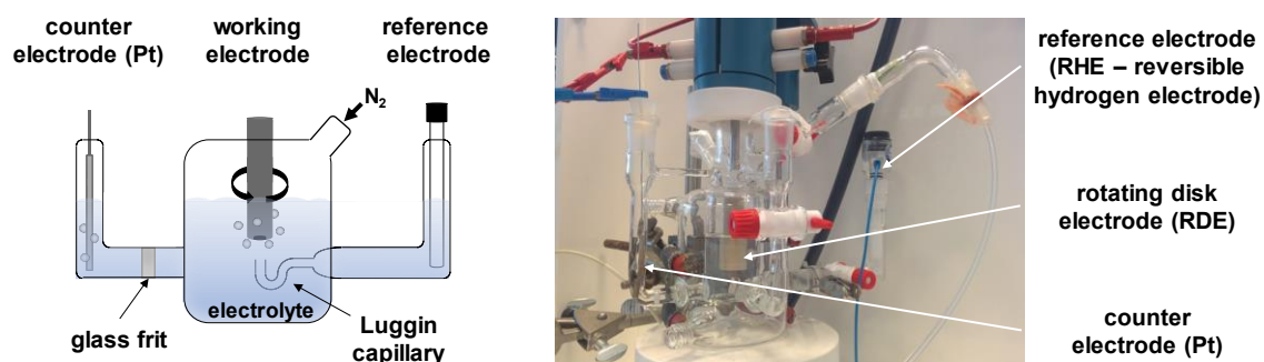
Figure 13: Illustration of the three-electrode disc setup used for electrocatalytic studies. Mesoporous \text{IrO}_x coated Ti substrate (5 mm) served as working electrode, a Pt gauze as counter electrode and a reversible hydrogen electrode (RHE) as reference electrode. All potentials were corrected for iR drop. Electrochemical measurements were either performed in \text{N}_2 purged (30 min) 0.5M \text{H}_2\text{SO}_4 or 0.1M \text{HClO}_4 and a rotating disc speed of 1600 rpm.
