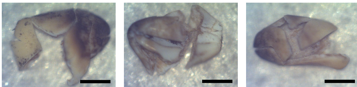
Figure 5.9: Optical microscopy images of 3 examples of 0.5 M \text{Na}_2\text{SiO}_3 incorporated FS based particles. Irregular shape and inhomogeneity formation occurred due to high concentration/amount of \text{Na}_2\text{SiO}_3 (scale bar: 0.5 mm)
