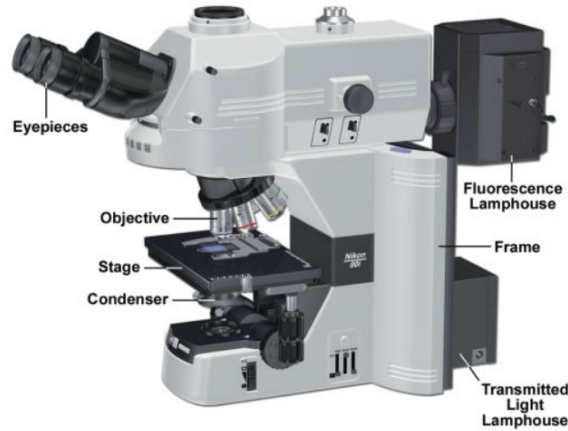
Figure 2.1: Main components of a compound light microscope. Reproduced from ref 2
