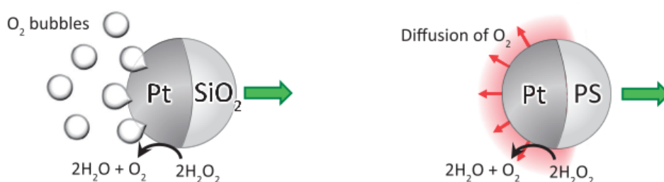
Figure 1.15: Schematic illustration of propulsion mechanisms in the opposite direction of the catalyst: Left: Bubble propulsion, Right: Self-diffusiophoresis. Reproduced from ref 41
