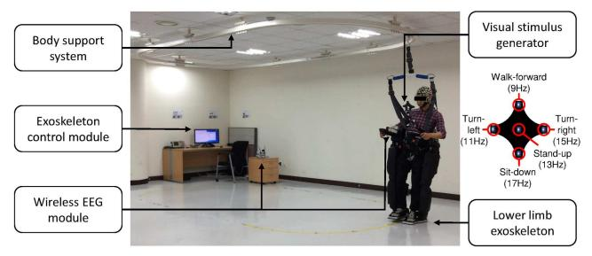
**Fig 1. Experimental environment.** Subject wearing the lower-limb exoskeleton and focusing on an LED from the visual stimulus generator. The EEG is transferred by a wireless interface to the PC. A body support system (a rail beneath the ceiling) was connected to the subject for safety purposes. The exoskeleton was controlled by an external operator using a keyboard controller.
