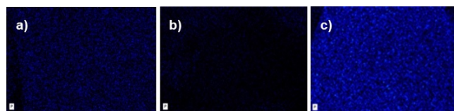
Figure 9. EDX mapping with color-coded intensity range of phosphorus. a) 5bb @SiO 2 after five reaction cycles, b) neat SiO 2 support, and c) immobilized catalyst 5bb @SiO 2 . [24]
