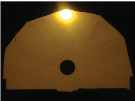
Figure 6: Illumination of the half sphere with a HPS lamp through a diffuser
