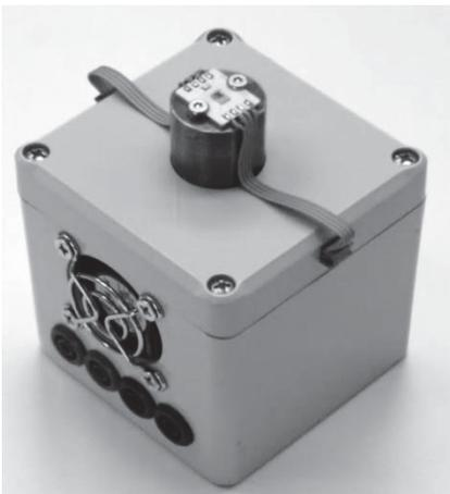
Figure 2: Temperature controlled test socket equipped with LED
