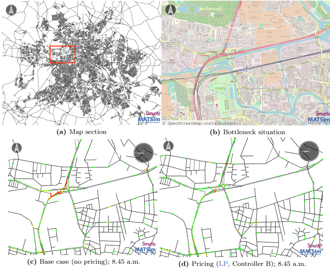
Figure 4.6: An inner-city motorway bottleneck situation: Red indicates a delayed vehicle; Green indicates a non-delayed vehicle. Map layer: © OpenStreetMap contributors. (Simulation experiment with route, departure time and mode choice)
