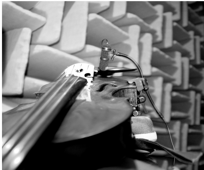
Figure 6.3: Position of the DPA microphone on the violin.
