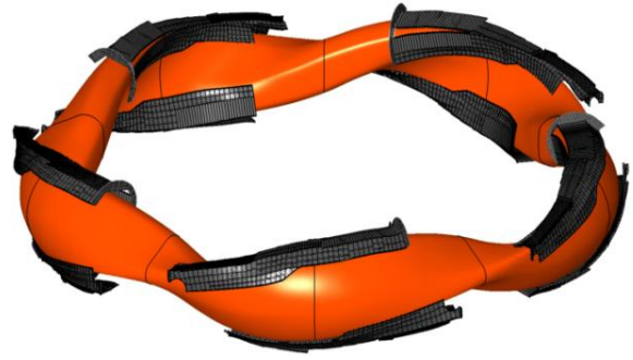
Fig. 2: Plasma contour (orange) with (a) 5 inboard limiters made of graphite (black stripes) defining the last closed flux surface. Fig. 2(b) shows the ten divertor units with the target plates following the topology of the resonant magnetic island divertor.
