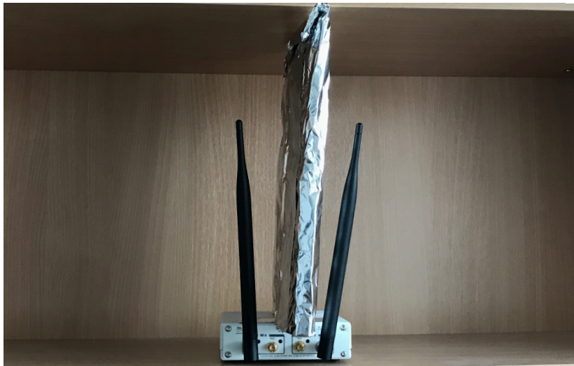
FIGURE 3.11 – Very simple passive suppression approach that isolates the Tx-Rx front-ends.
