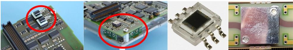
**Figure 4.5:** Attitude sensors of BEESAT-1: Magnetic field sensors on left side, gyroscopes in the center, sun sensor aperture plate and PSD on right side [132, 133]
