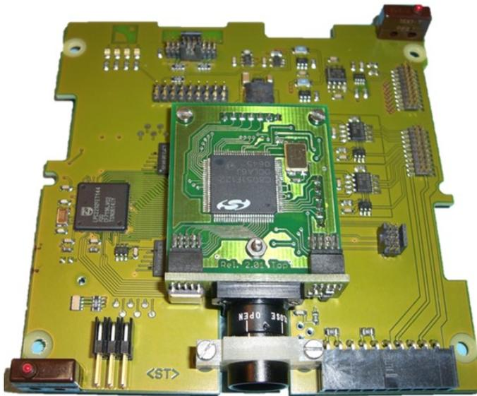
**Figure 4.10:** Payload Data Handling of BEESAT-2 with camera module (image credit: Sebastian Trowitzsch)
