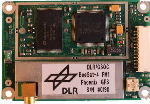
**Figure 2.4:** Flight model of the Phoenix GPS receiver for BEESAT-4
