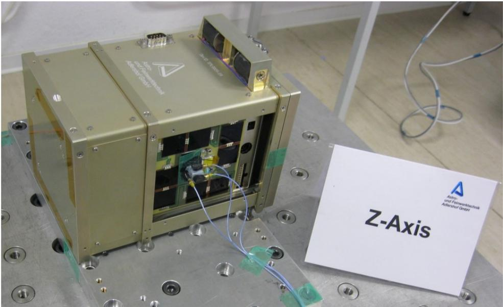
**Figure 5.5:** BEESAT-4 on the shaker in an SPL
