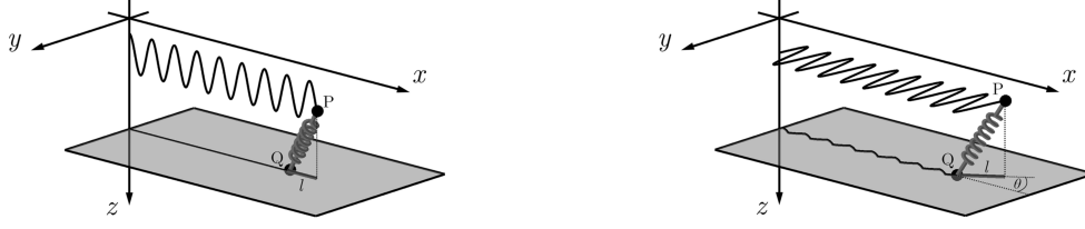
Figure 5: An elastic body modeled as a spring with a normal and tangential stiffness is forced into a controlled movement at the upper point P, while the contact point Q follows according to the equilibrium conditions. Left: Schematic representation of the considered system for the case of normal oscillations, right: schematic representation of the considered system for the case of sideways oscillations. Images: (Benad, Popov et al. 2018)
