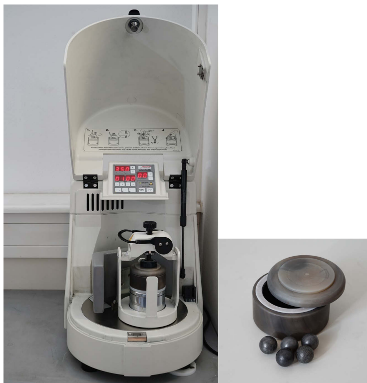
Figure 3.2.: Ball mill PULVERISETTE 6 and agate grinding bowl/balls
