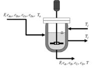
Figure 2. General scheme of the CSTR including all inputs and outputs.
