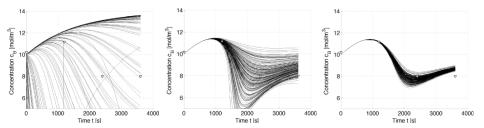
Figure 4. Monte Carlo simulation for the first parameter estimation with all parameters (a), with SsS 0 (b), and with SsS III (c) (from left to right) for experiment 7.
