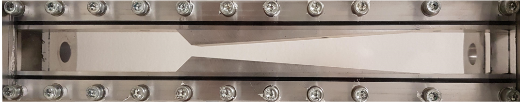
Figure 3.18: Visualization section for the shadowgraphy measurements. In this figure, a ramp geometry is installed with a converging area ratio of 4.0, a convergent half-angle of 45^\circ , and a divergent half-angle of 4^\circ .
