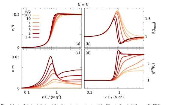
**Figure 2.** Leaving the bad cavity limit: variation of the external pumping strength for different ratios  $\kappa/g$ : (a) the normalized TLS excitation number  $n/N = \langle J_{11} \rangle / N$ , (b) the relative superradiant subspace occupation  $R(l_{\text{max}} = N/2)$ , (c) the cavity output rate  $\kappa m = \kappa \langle b^{\dagger}b \rangle$  and (d) the photonic second order correlation function  $g^{(2)}(0)$ : drastic qualitative change for  $\kappa/g$  approaching unity.
