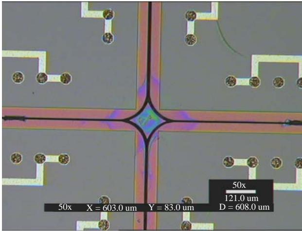
commercial available wafers. Therefore, a modified DbyT process was developed where a good edge quality is achieved by a combination of sawing and etch processes (Feil *et al.*, 2004).
