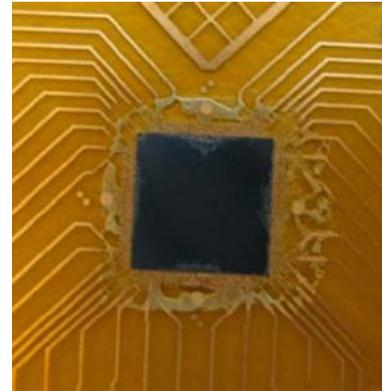
contamination and process disturbance are a consequence. Too small an amount fails to fill the gap between chip and substrate. The latter may result in opens between chip and substrate and therefore has to be avoided. The bonding temperature at its maximum was 230°C and was held for 20 s, followed by cooling at a rate of 10°C/s. An 8.8 kg force during bonding was applied before the maximum temperature was reached and released when the temperature had dropped below 100°C.
