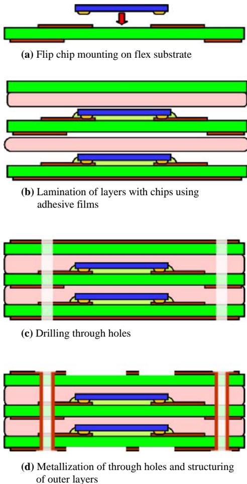
**Figure 3** Four layers of FPC with ultra thin flip chips symmetrically laminated. White dots are the filler particles of the ACA
