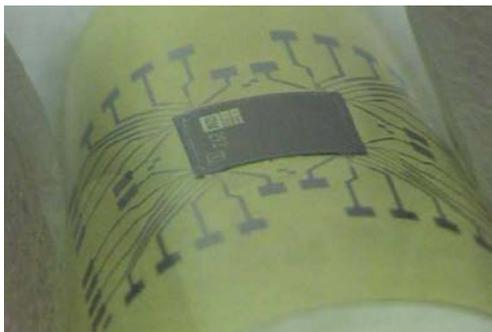
This results in a very thin flexible chip package (down to 60 μm thickness) (Figure 9).
