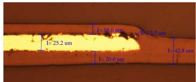
**Figure 7** Fan out metallization
