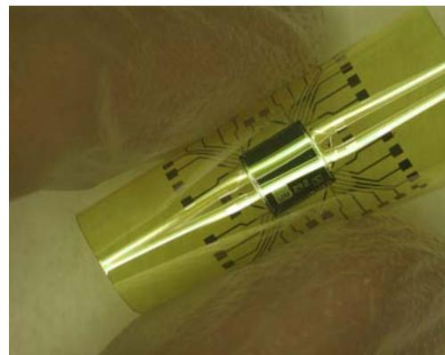
**Figure 10** Rounded corners of a 25 μm thin chip; prepared by dry etched grooves at front side of wafer and subsequent backside thinning
