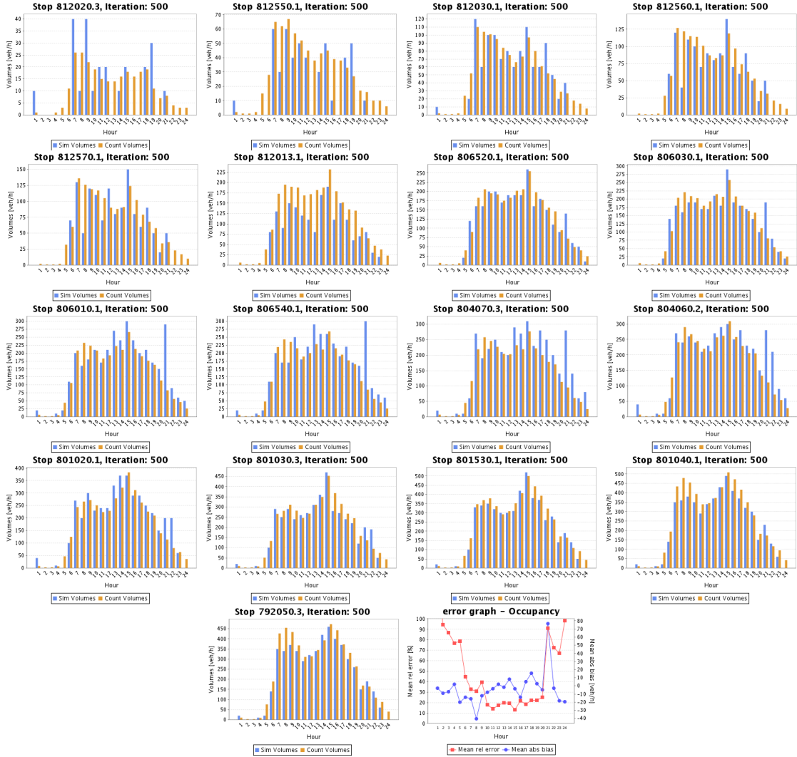
FIGURE 4.1: Per stop counts data-simulation comparison plots and general error graph after automatic calibration (5x expanded population).
