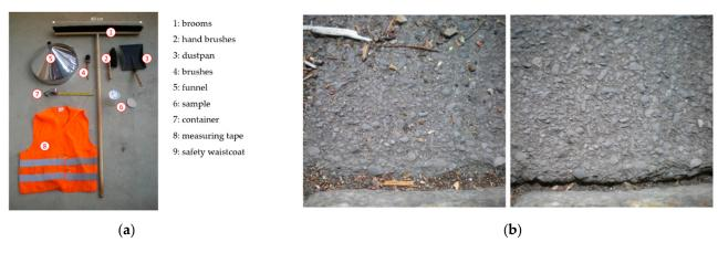
Figure 2. (a) RDS sample equipment (b) before/after close-up of a RDS sampling.
