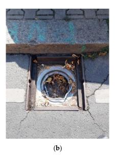
Figure 3. (a) Road runoff sampling basket (full flow sampling) and (b) in situ use.
