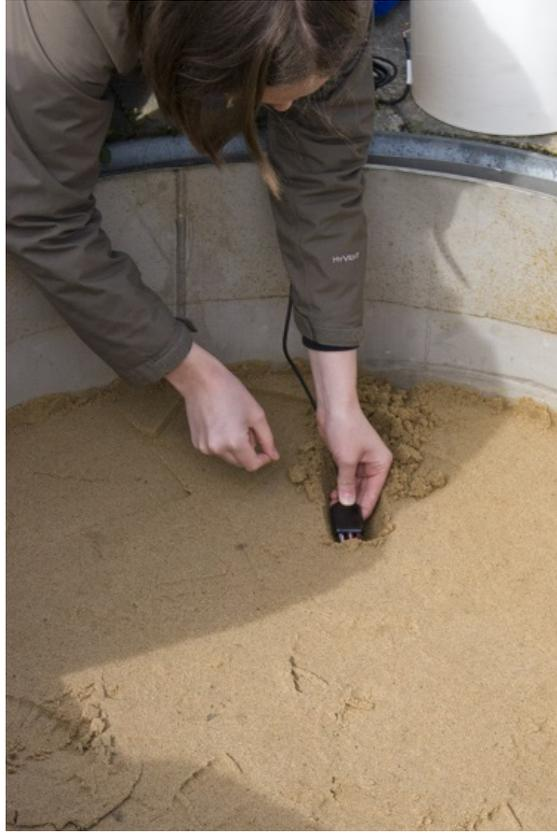
Figure A.4: Installation of sensor for soil water content and temperature measurement, sensor is pushed into already compacted soil
