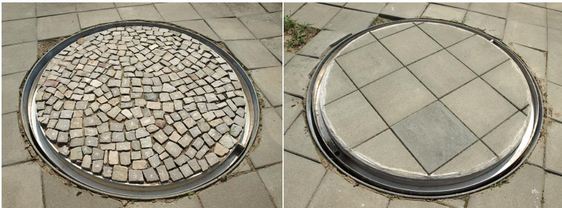
Figure 3.3: Lysimeter surfaces: left – cobblestones, right – concrete slabs
