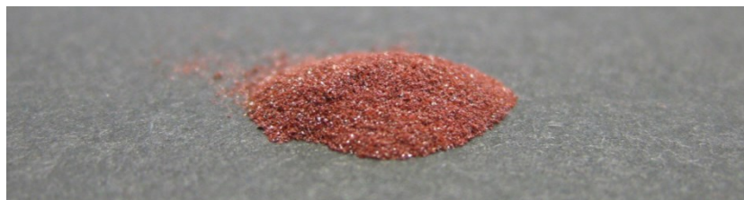
Figure 9.1. Sample of \delta -TaON with \gamma -TaON and \text{Ta}_3\text{N}_5 side phases.
