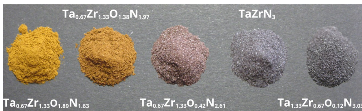
Figure 9.2. Synthesized tantalum zirconium oxide nitrides and the nitride \text{TaZrN}_3 . Left to right: \text{Ta}_{0.67}\text{Zr}_{1.33}\text{O}_{1.89}\text{N}_{1.63} , \text{Ta}_{0.67}\text{Zr}_{1.33}\text{O}_{1.38}\text{N}_{1.97} , \text{Ta}_{0.67}\text{Zr}_{1.33}\text{O}_{0.42}\text{N}_{2.61} , \text{TaZrN}_3 , and \text{Ta}_{1.33}\text{Zr}_{0.67}\text{O}_{0.12}\text{N}_{3.03} .
