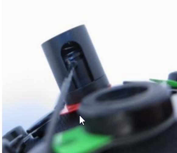
FIGURE 2.8: Spring-loaded fiber holders. The spring keeps the tip of the optode at constant pressure, reducing the possibility of loss of contact between the tip and the scalp.
