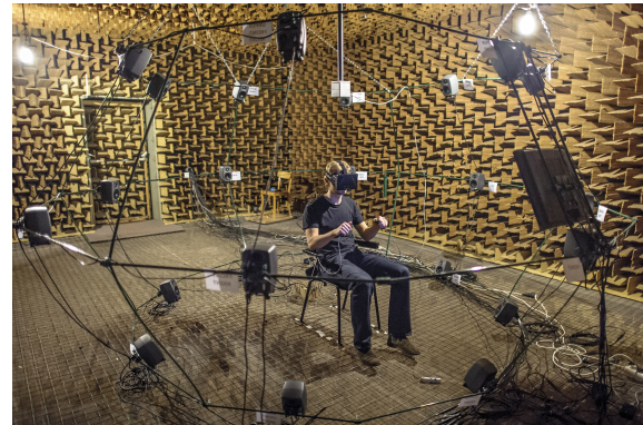
Figure 4: Listening tests were conducted in an anechoic chamber equipped with 24 loudspeakers for spatial reproduction.
