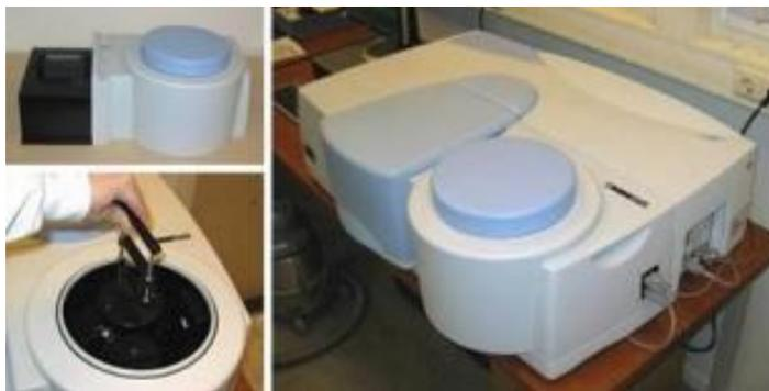
Fig 3. 3 UV/VIS/NIR spectrometer with ARTA [78].
