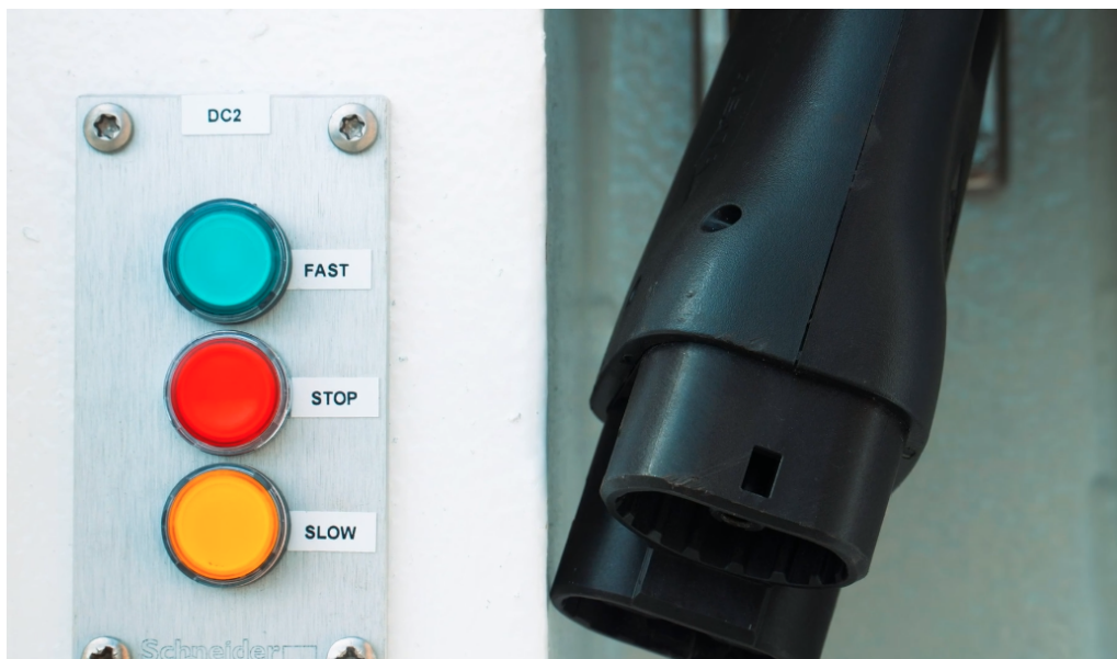
Figure 2.3: The controls of construction site BESS
