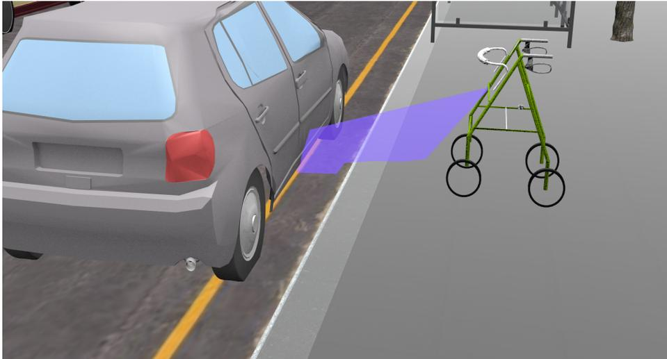
**Figure 4.14:** A 3D model of the LEDDAR sensor to detect the curbstone
