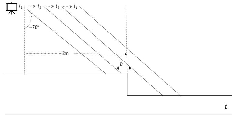
**Figure 4.13:** Schematic diagram of the LEDDAR sensor
