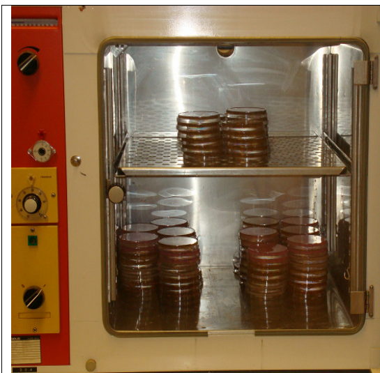
A. 100: Static incubator for agar cultures
