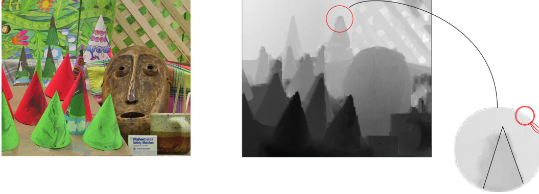
Figure 5.4: Estimation of depth map using a pair of images.
