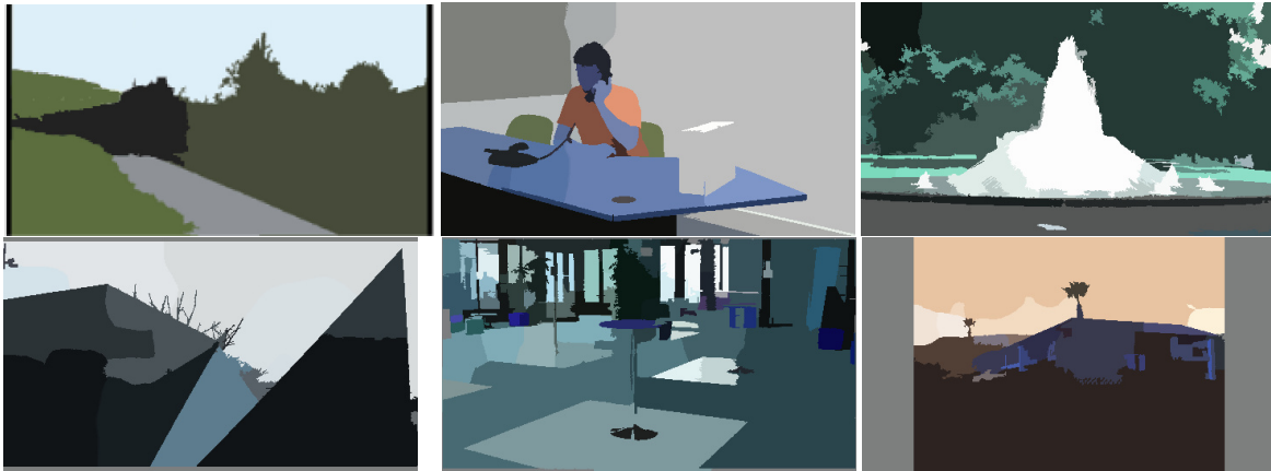
Figure 5.12: Example of image segmentation using the mean-shift.
