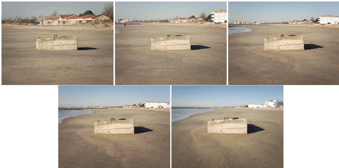
Figure 2.32: Relation between object geometry and focal length (images from Micaël Reynaud)
