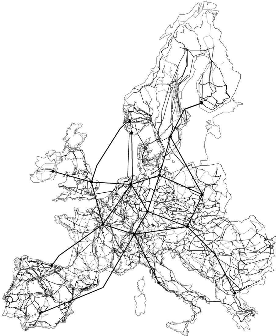
Figure 7.2: Initial network topology for Europe and HVDC overlay grid<sup>111</sup>
