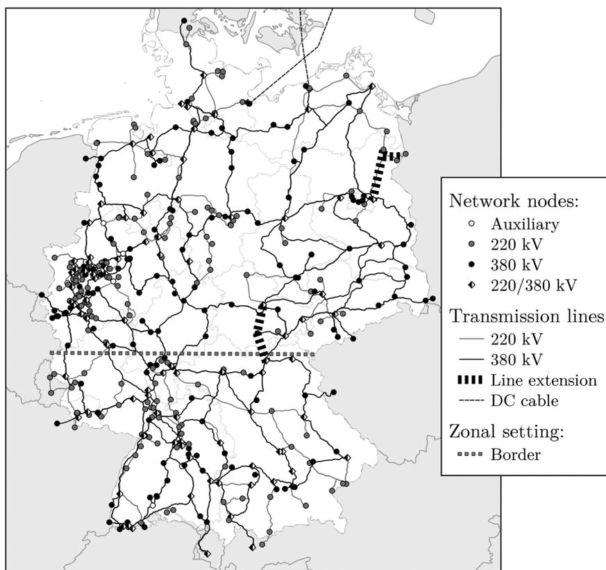
Figure 3.3: High-voltage transmission network in 2012, two bidding zones, and additional lines in the transmission extension scenario
