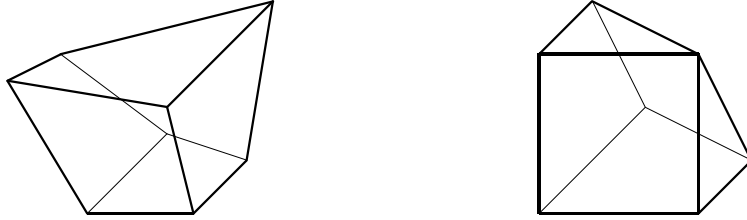
Figure 4.1: A non-degenerate and a degenerate hexahedron.
