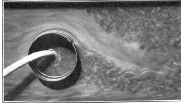
Figure 1.1: Active separation control conducted by Ludwig Prandtl - the figure shows the flow around a cylinder where suction is applied on the upper surface; photogram taken by Prandtl (1904), based on figure in Ref. [5]
