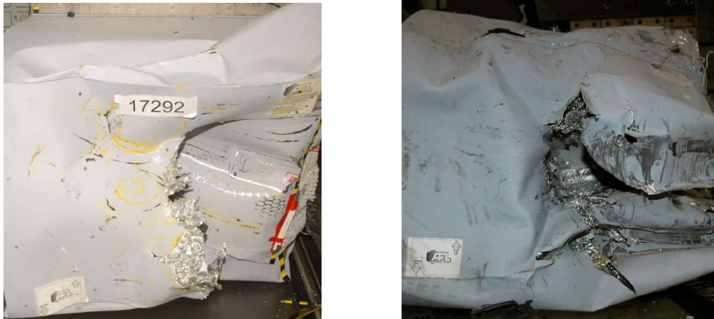
Figure 4.56: Covered pocket due to rotation of the vehicle (left) and covered areas due to rupture of the cladding plate (right).
