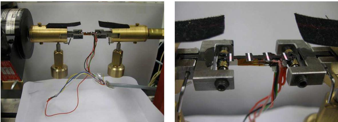
Figure 6.7: Experimental setup of tension and compression tests.
