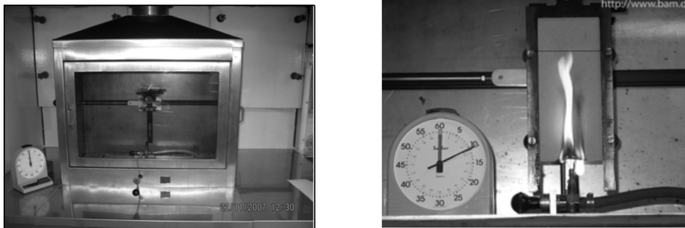
Figure 2.7 Flame test according to DIN 4102-1 (Single-Flame Source Test (Ignitability Apparatus, EN ISO 11925-2))
