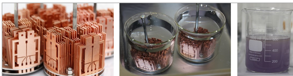
Figure 4.4: Cleaning process of the lead frames, first placing of lead frames into the carrier (left), cleaning in the ultrasonic bath in cleaning solution and in distilled water (middle), cleaning solution, which changes the color from transparent to violet after the cleaning (right)
