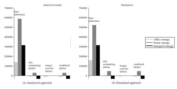
Fig. 2: Energy consumptions for the one percent sample. The first data triple are absolute consumptions (base case); the next three data triples are differences compared to the base case.
