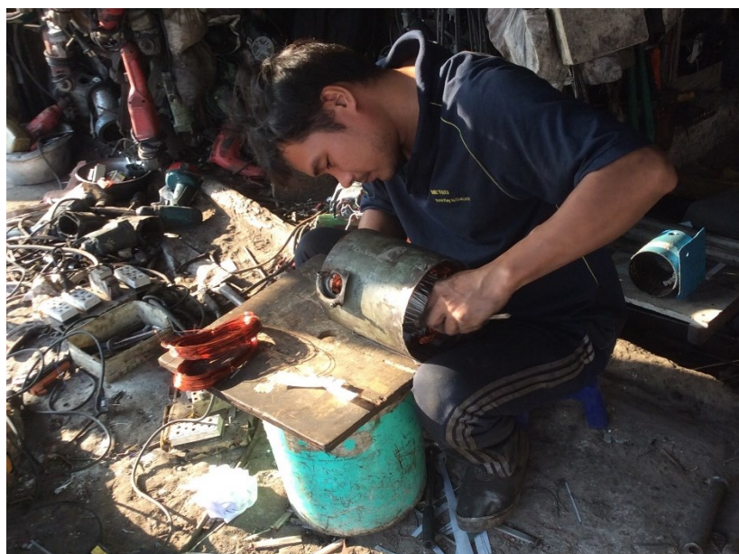
Figure 5-1: Water pump rewinding in a Vietnamese repair workshop
