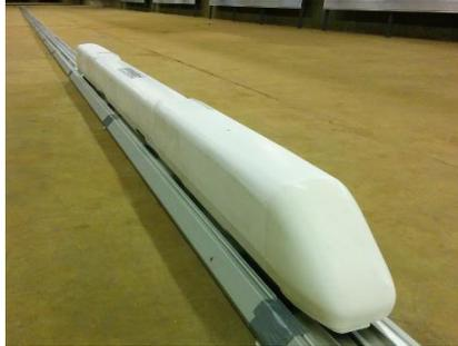
Fig. 10: 1:22 scale 3-car ICE/V model (simple configuration) on test track in empty towing tank
