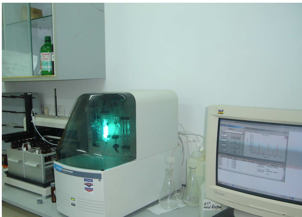
Fig. 3.15 Laboratory analyses of samples for Organic and Inorganic Carbon
