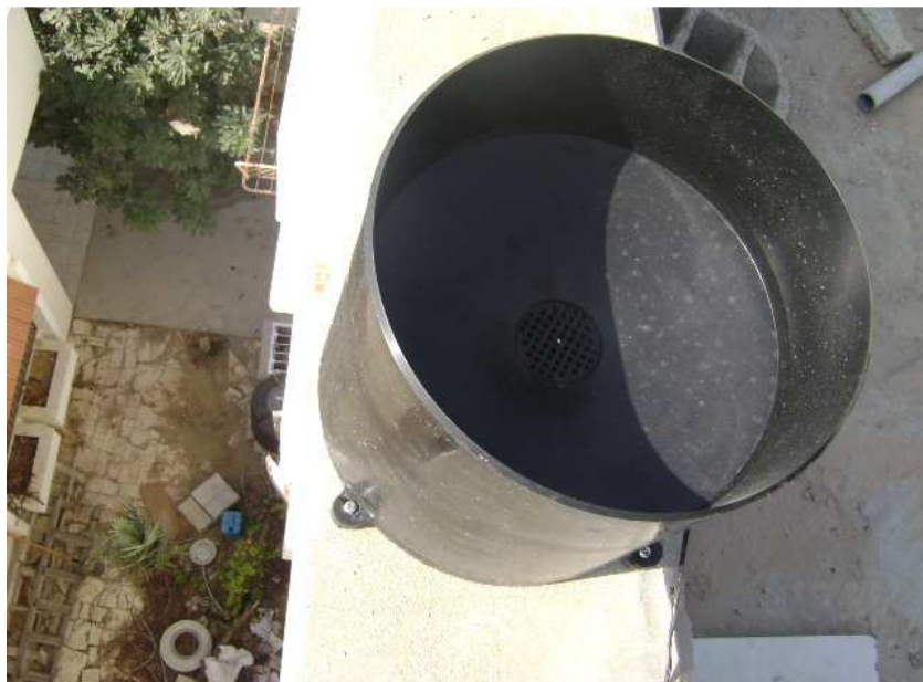
Fig. 3.7 Installed rain gauge on the house roof
