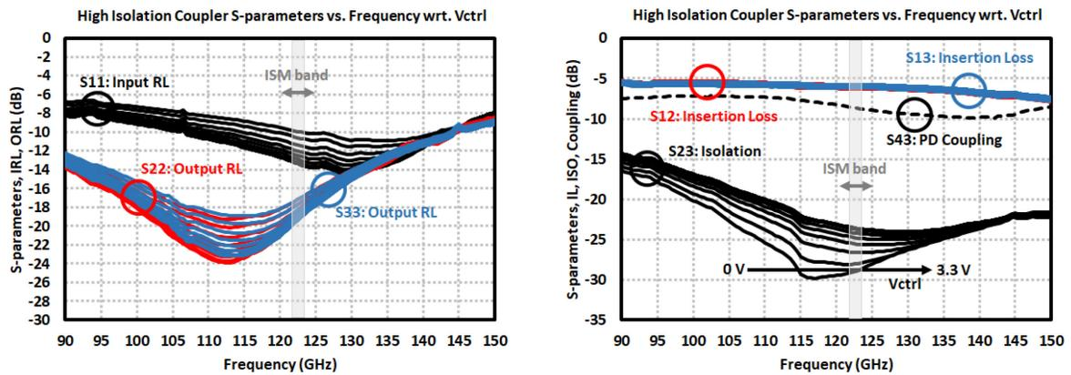
Figure 3.24: Simulation results of 122 GHz high isolation coupler: (*left*) input and output return losses, (*right*) insertion loss, isolation and coupling loss to power detector with respect to tuning voltage.
