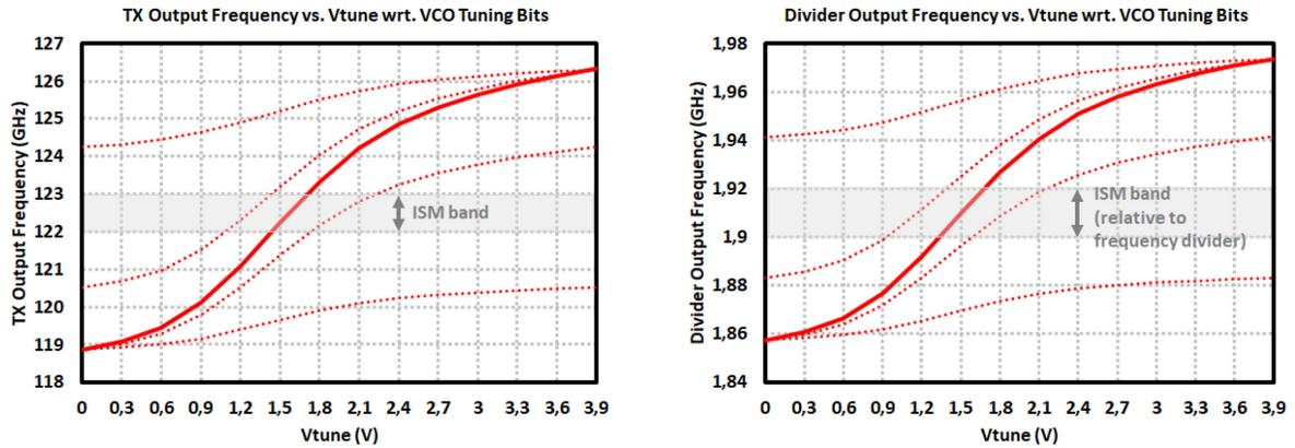
Figure 4.11: Measurement results of the 122-GHz TR2 TRx: (*left*) Tx output frequency and (*right*) Frequency Divider output frequency vs. VCO tuning voltages with respect to VCO tuning bits.
