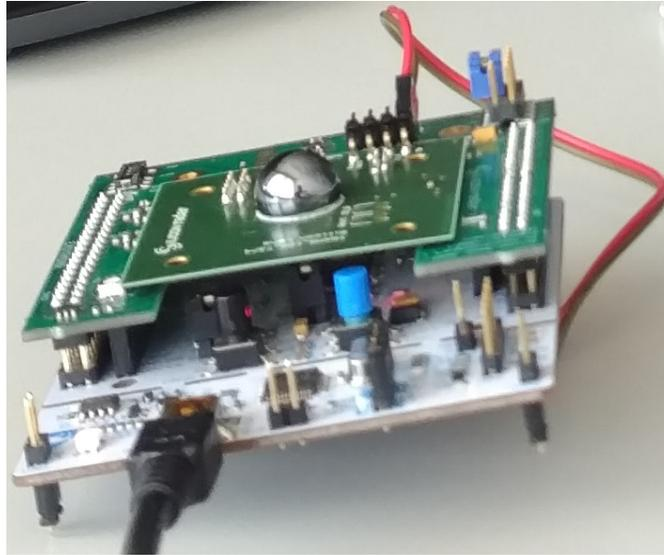
Figure 5.22: Radar evaluation board of 122-GHz TRMant chip with Silicon-lens of 2.0 mm height and 5.5 mm radius.
