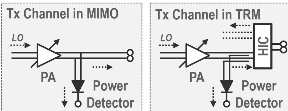
Figure 3.31: BIST circuits and coupling mechanisms including power detectors in Tx channels of, (left) 60-GHz MIMO TRx, (right) 60- / 122-GHz TRM.
