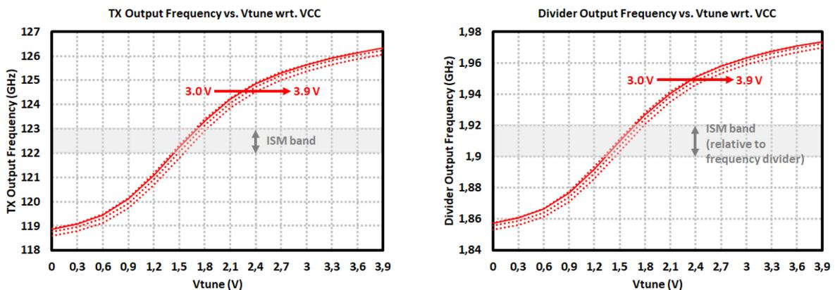
Figure 4.12: Measurement results of the 122-GHz TR2 TRx: (*left*) Tx output frequency and (*right*) Frequency Divider output frequency vs. VCO tuning voltages with respect to changing supply voltages between 3.0 V – 3.9 V.
