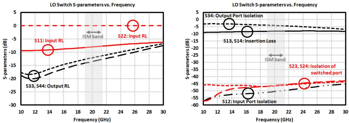
Figure 3.47: Simulation results of 20-GHz differential multiplexer.
