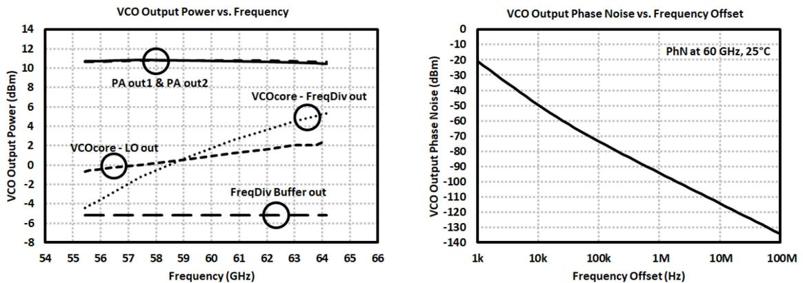
Figure 3.38: 60 GHz VCO, (Left) power levels: PA out1 / out2 output power, frequency divider and PA input power delivered from VCO core, frequency divider buffer output power, (Right) phase noise at 60 GHz.
