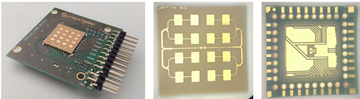
Figure 5.32: Photo of fabricated 60-GHz TRM BSA package and its view in radar evaluation board.
