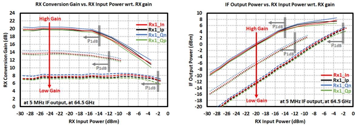
Figure 4.9: Measurement results of the 60-GHz TR2 TRx: (*left*) Rx channel 1 conversion gain, and (*right*) IF channel 1 output power vs. Rx input power at 64.5 GHz with respect to Rx gain control voltages.
