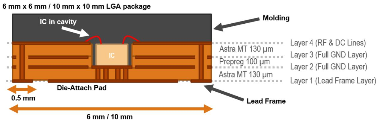
Figure 5.35: 60-GHz LGA package PCB stack-up.
