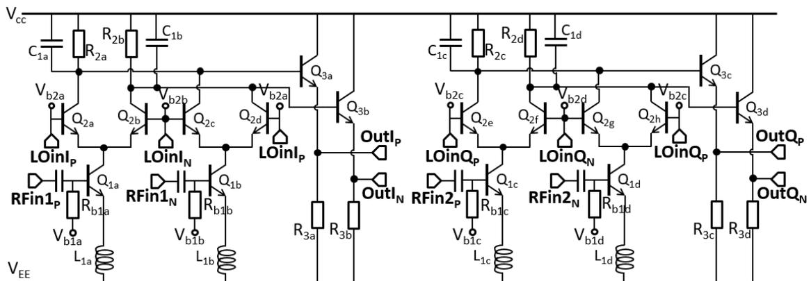
Figure 3.13: Schematic of 60 GHz double-balanced Gilbert-cell based quadrature mixer.
