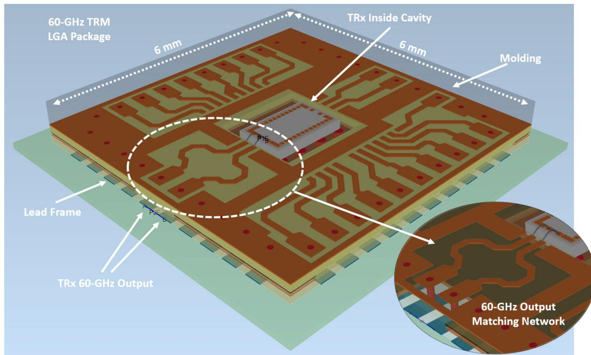
Figure 5.39: Simulated 60-GHz TRM 6 x 6 mm<sup>2</sup> LGA package structure.
