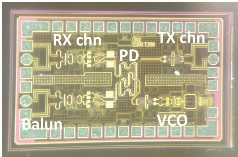
Figure 4.10: Photo of the fabricated 122-GHz TR2 transceiver chip occupying 1.54 mm x 0.92 mm area.
