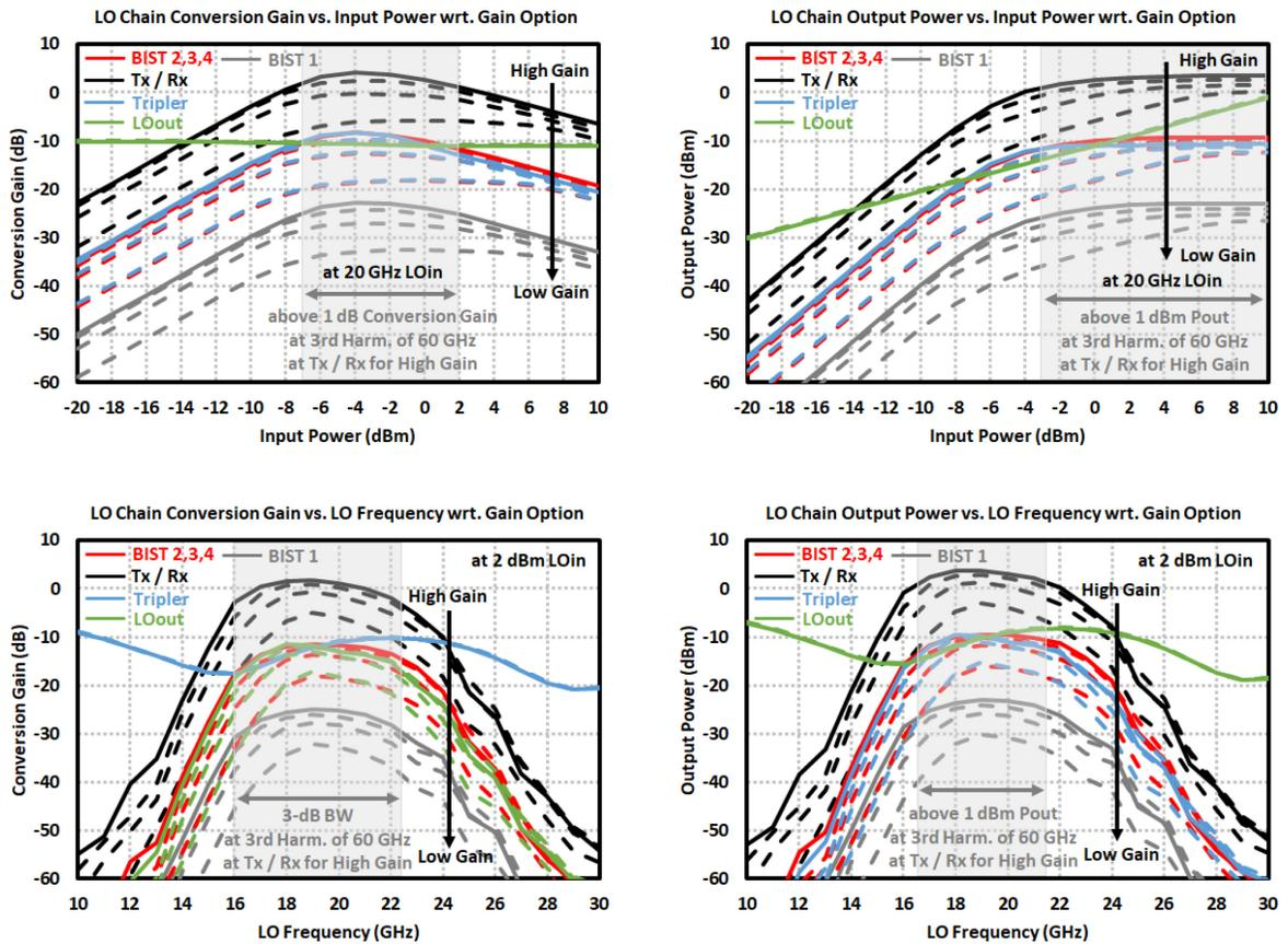
Figure 3.67: Simulation results of the complete LO chain in 60-GHz MIMO TRx with respect to different gain options in *master* mode: (*top left*) conversion gain vs. input power at 20 GHz internal VCO input, (*top right*) output power vs. input power at 20 GHz internal VCO input, (*bottom left*) conversion gain vs. LO input frequency at 2 dBm internal VCO input, (*bottom right*) output power vs. LO input frequency at 2 dBm internal VCO input.
