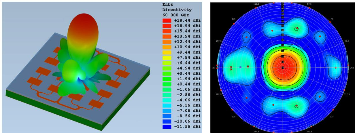
Figure 5.33: 60-GHz TRM BSA antenna simulation results (3D radiation pattern at 60 GHz).
