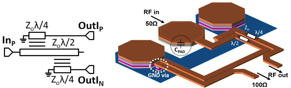
Figure 3.20: Schematic and layout of 122 GHz Marchand Balun.
