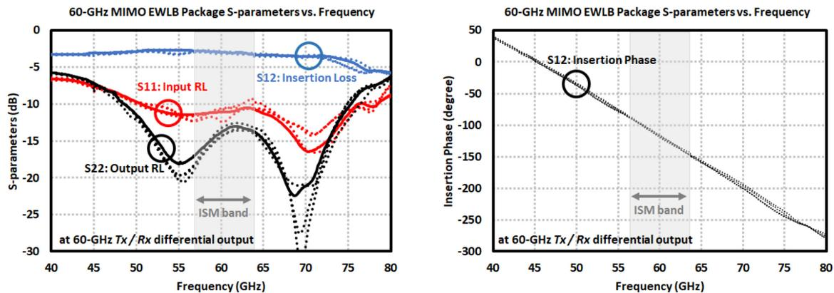
Figure 5.59: S-parameter results of differential 60-GHz Tx / Rx outputs in EWLb package.
