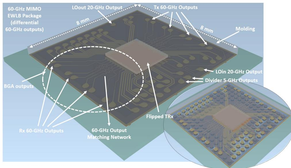
Figure 5.55: Simulated 60-GHz MIMO  $8 \times 8 \text{ mm}^2$  EWL B package structure with differential 60-GHz outputs.
