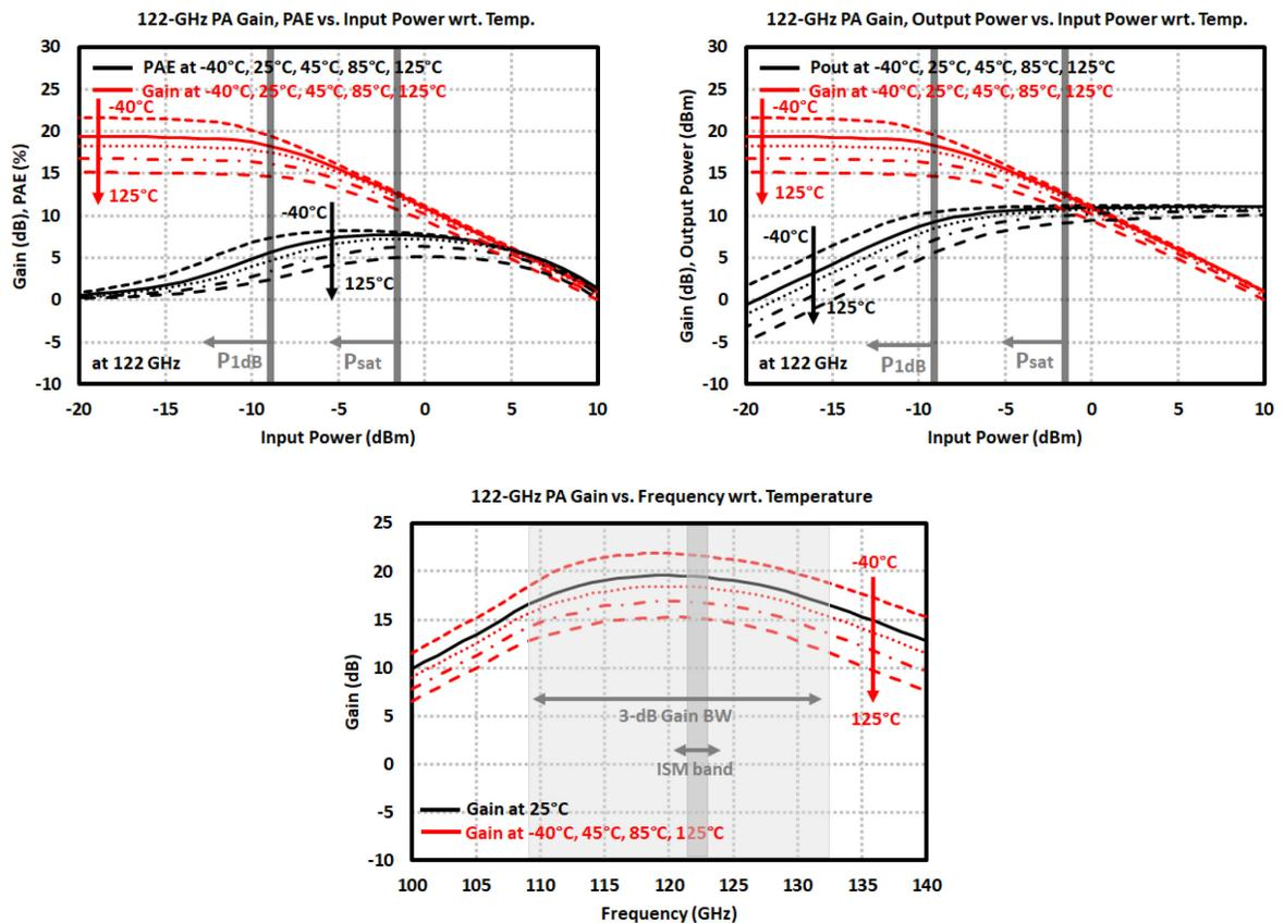
Figure 3.30: Simulation results of 122-GHz PA: (top left) gain and PAE at 122 GHz with respect to temperature, (top right) gain and output power at 122 GHz with respect to temperature, (bottom) gain with respect to temperature.
