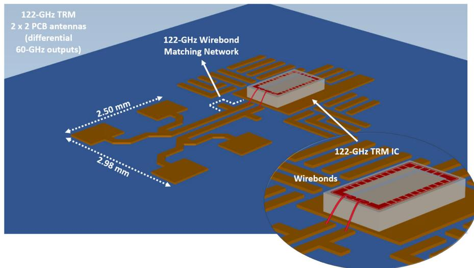
Figure 5.2: PCB antenna concepts of 122-GHz TRM chips including wirebond compensation network.
