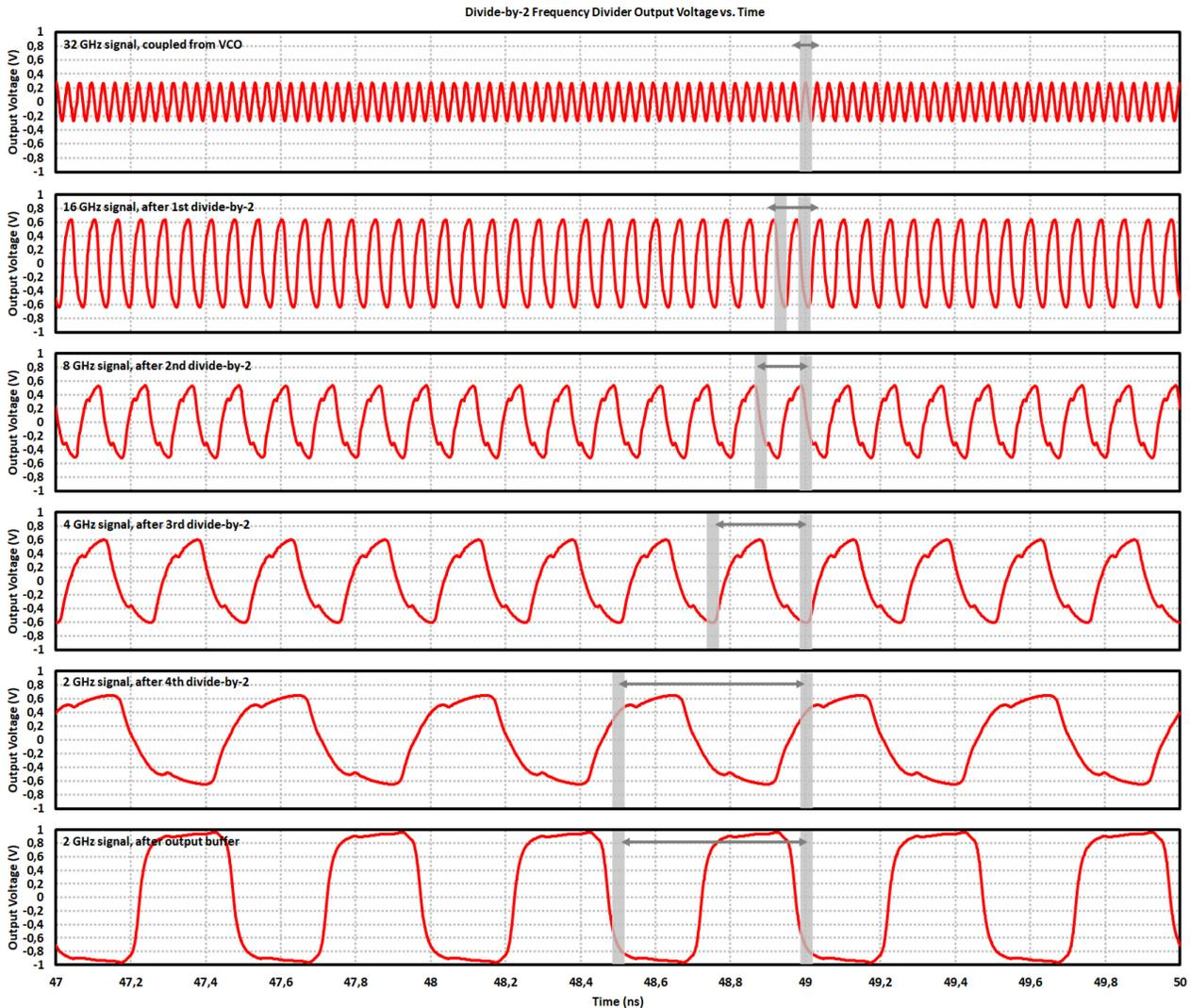
Figure 3.44: Divide-by-16 frequency divider output voltage at each divide-by-2 output node.
