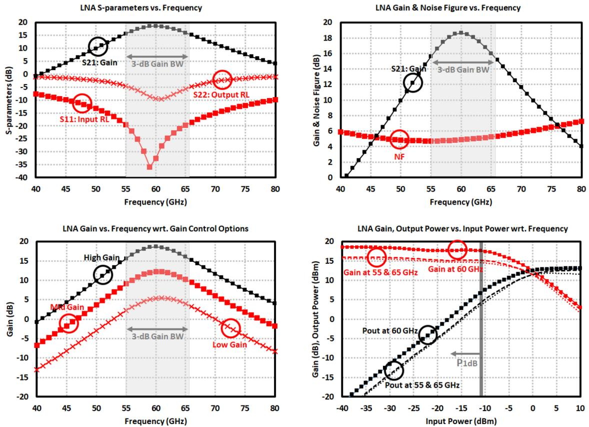
Figure 3.7: Simulation results of 60 GHz LNA: (*top left*) S-parameters, (*top right*) gain and noise figure, (*bottom left*) gain with respect to control options, (*bottom right*) gain and output power with respect to frequency.
