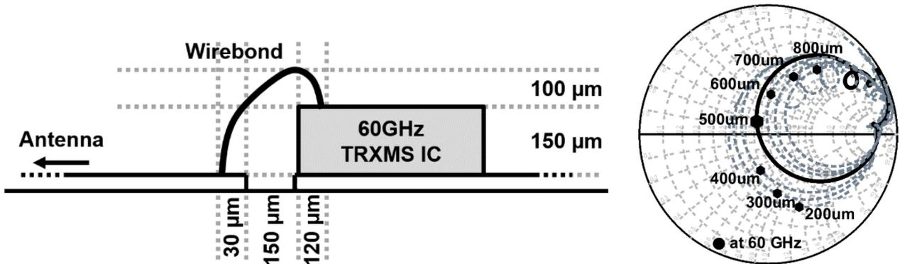
Figure 5.3: Wirebond drawing and effect of wirebond length on return loss [18].
