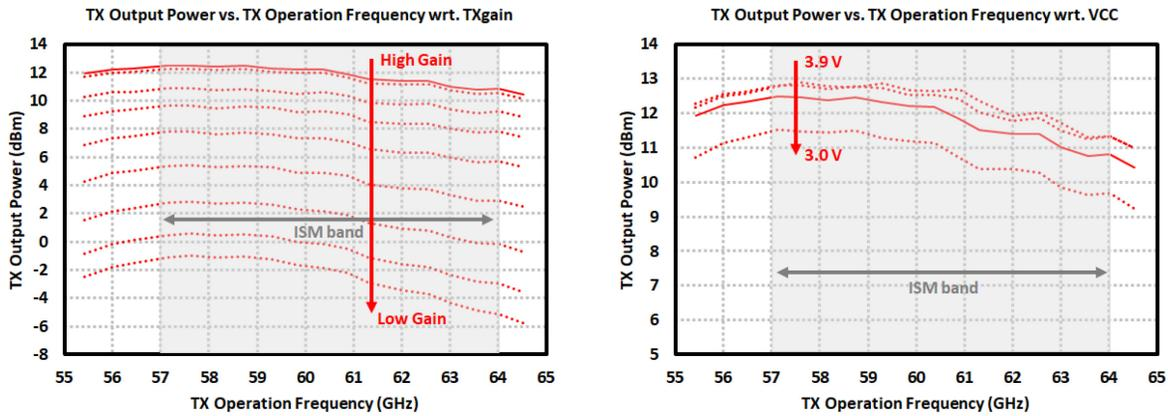
Figure 4.33: Measurement results of the 60-GHz MIMO TRx in *master* mode where internal VCO is enabled: Tx output power vs. frequency with respect to (left) Tx gain control voltages 0 V – 3.3 V and (right) changing supply voltages between 3.0 V – 3.9 V.
