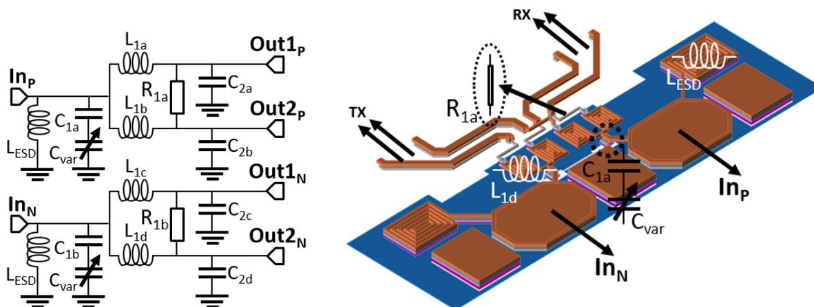
Figure 3.22: Schematic and layout of 60 GHz high isolation coupler.
