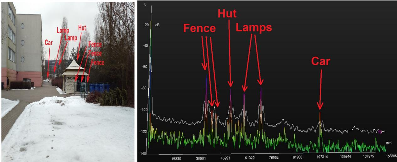
Figure 6.12: Outdoor measurement using the radar board of 122-GHz TRM including the lens with the farthest available target being the mid-sized vehicle at 107 m [16].
