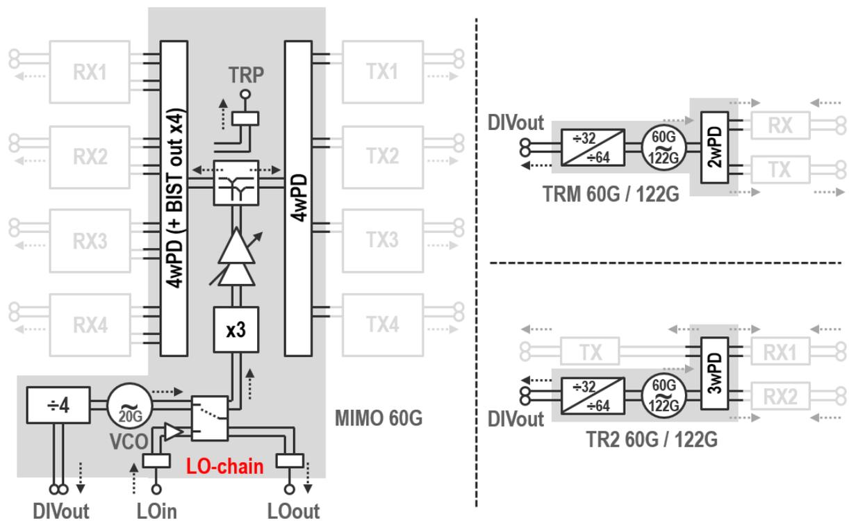
Figure 3.35: LO signal distribution networks for different chips including monostatic, double-receive, MIMO TRx.
