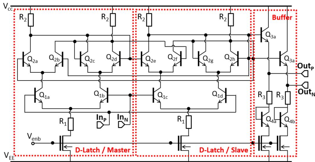
Figure 3.42: Schematic of Divide-by-2 circuit composed of two D-latches and a buffer.
