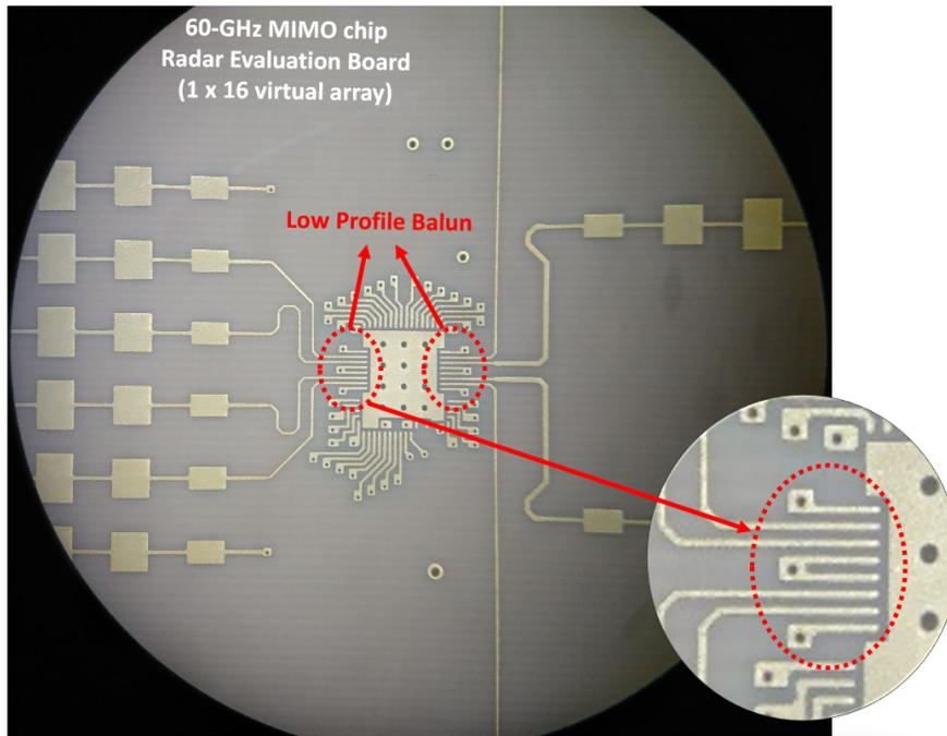
Figure 5.14: 60-GHz MIMO radar evaluation boards highlighting the PCB-based balun.
