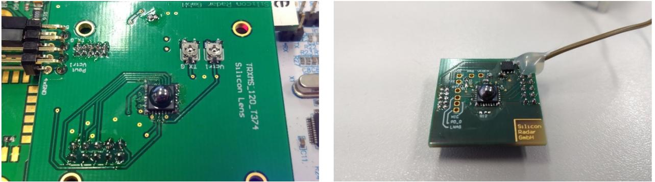
Figure 5.26: Manufactured radar evaluation boards including (left) 122-GHz TRMant and (right) 60-GHz TRMant Silicon package.
