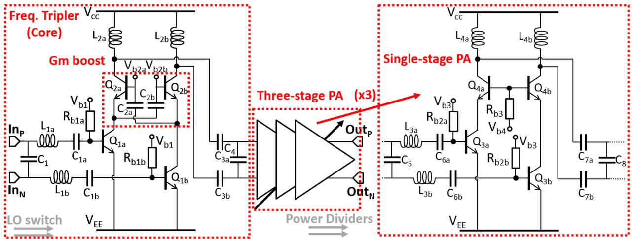
Figure 3.48: Schematic of 60-GHz frequency tripler.
