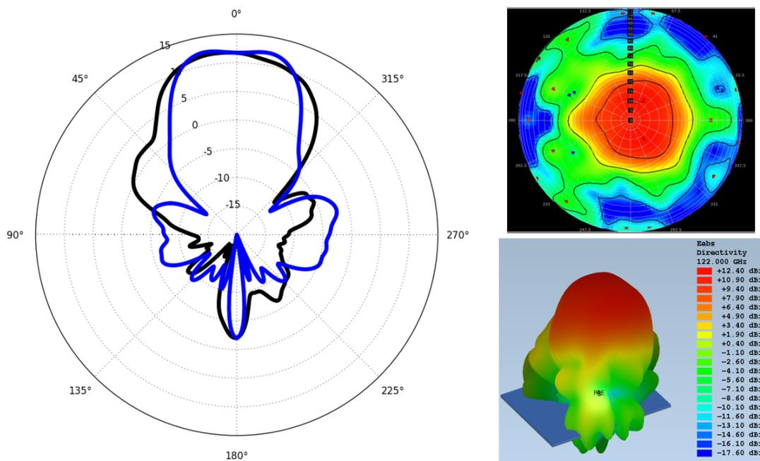
Figure 5.6: Simulation results of PCB antenna of 122-GHz TRM chip including wirebond compensation network.
