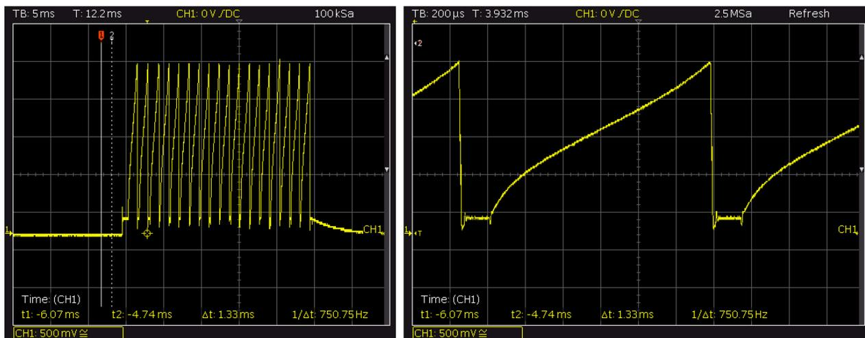
Figure 6.2: Saw-tooth chirp train generated by PLL to be sent through the Tx for 5 GHz modulation bandwidth.
