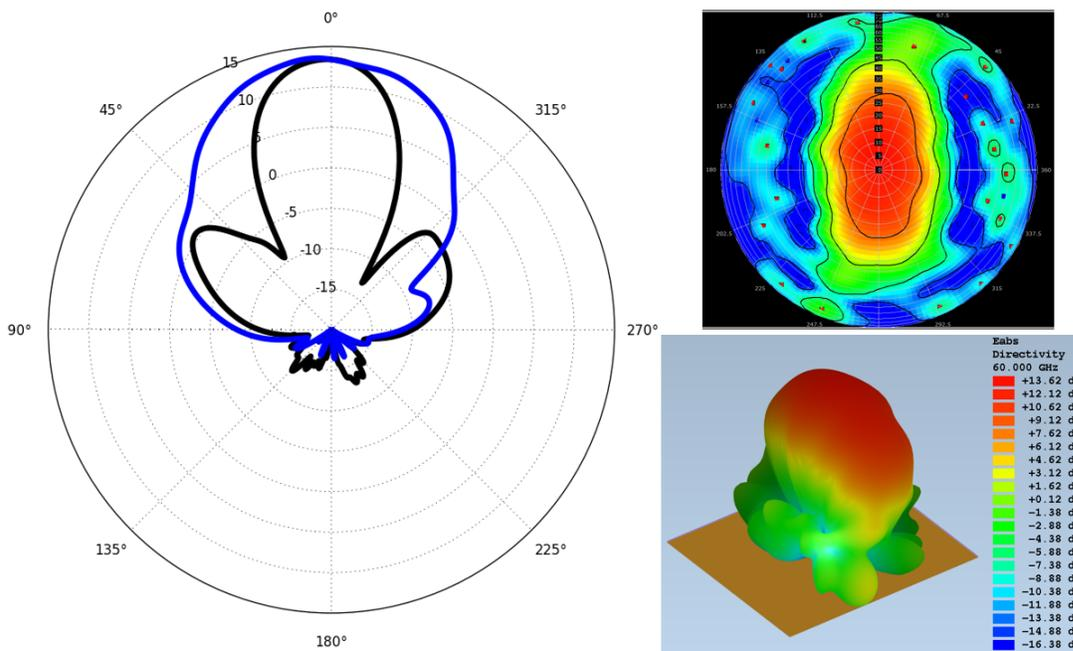
Figure 5.11: Simulation results of PCB antenna (2 x 2 patch array) of 60-GHz TR2 chip.
