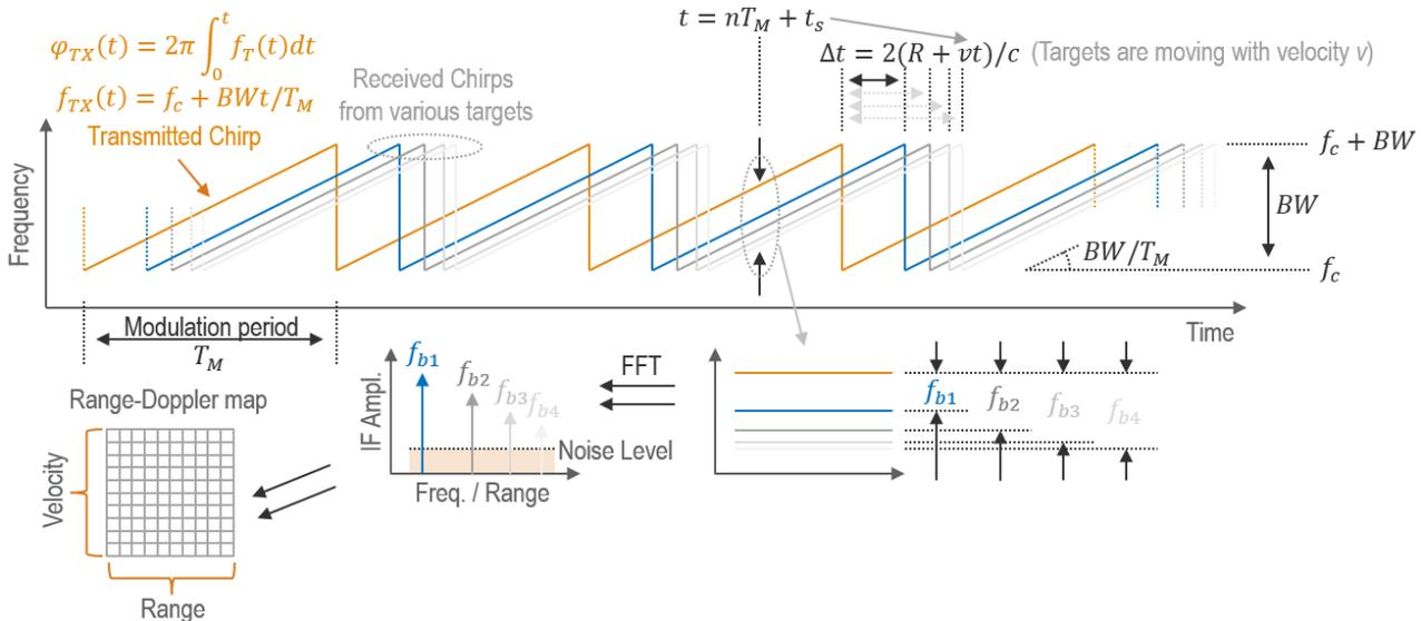
Figure 2.2: FMCW system illustration showing chirp modulation and beat frequency spectrum of the detected targets.
