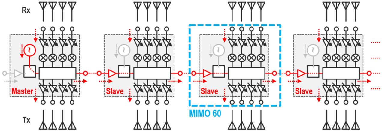
Figure 2.7: Block diagram of the massive MIMO chain composed of multiple scalable MIMO TRxs [19].
