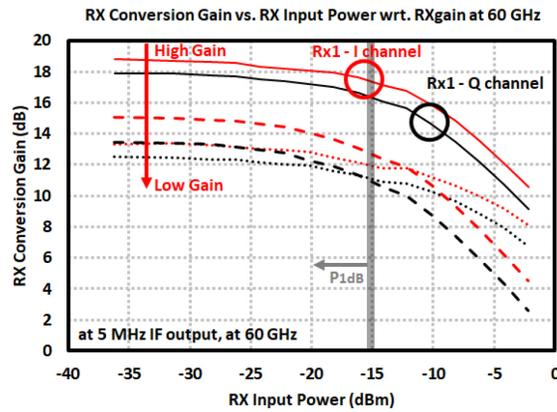
Figure 4.36: Measurement results of the 60-GHz MIMO TR<sub>x</sub> in *master* mode where internal VCO is enabled: Rx channel 1 conversion gain vs. Rx input power with respect to Rx gain control voltages.
