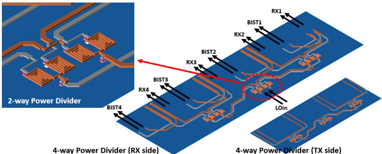
Figure 3.63: Layout of 60-GHz four-way power divider.
