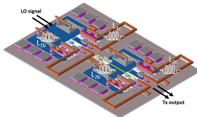
Figure 3.26: Layout of 60 GHz differential two-stage cascode PA circuit.
