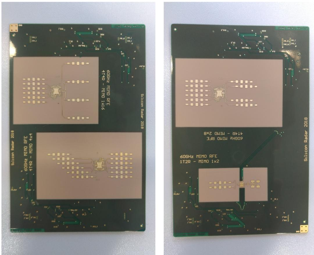
Figure 5.15: 60-GHz MIMO radar evaluation boards including antenna arrays for different virtual arrays.
