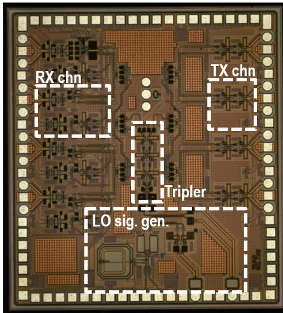
Figure 4.31: Photo of the fabricated 60-GHz MIMO transceiver chip occupying  $2.16$  mm x  $2.39$  mm area) [19].
