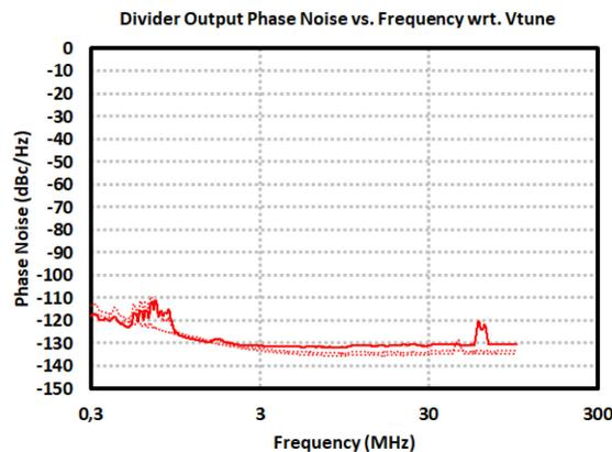
Figure 4.30: Measurement results of the 122-GHz TRM TRx: Frequency Divider phase noise at 1.86 GHz, 1.91 GHz and 1.97 (corresponding to Tx operation frequencies of 119.1 GHz, 122.2 GHz and 126.1 GHz).
