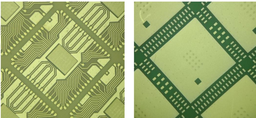
Figure 5.38: 60-GHz MIMO 10 x 10 mm<sup>2</sup> LGA package, top (RF and DC connections) and bottom (lead frame).
