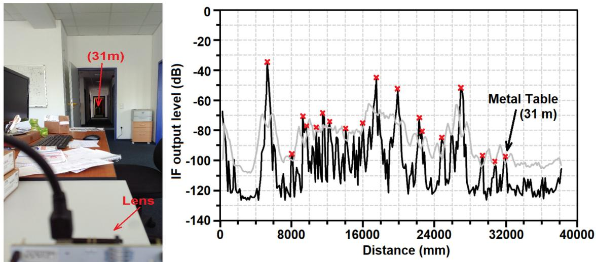
Figure 6.5: Complex indoor measurement using the radar board of 60-GHz TRM including the lens with the farthest available target being the metallic table at 31 m [18].
