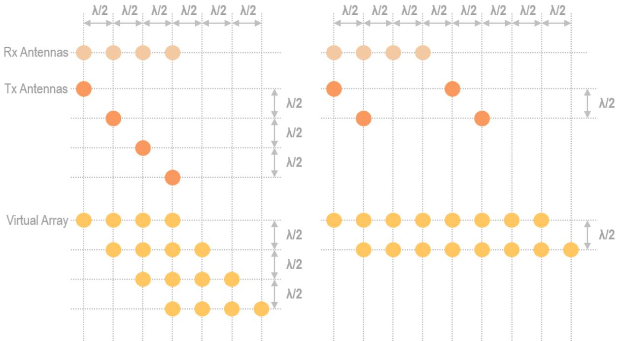
Figure 5.13: Illustration of two-dimensional 4 x 4 and 2 x 8 MIMO virtual array formations.
