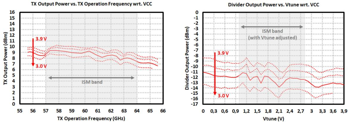
Figure 4.21: Measurement results of the 60-GHz TRM TRx: (*left*) Tx output power vs. frequency, and (*right*) Frequency Divider output power vs. VCO tuning voltages with respect to changing supply voltages between 3.0 V – 3.9 V.
