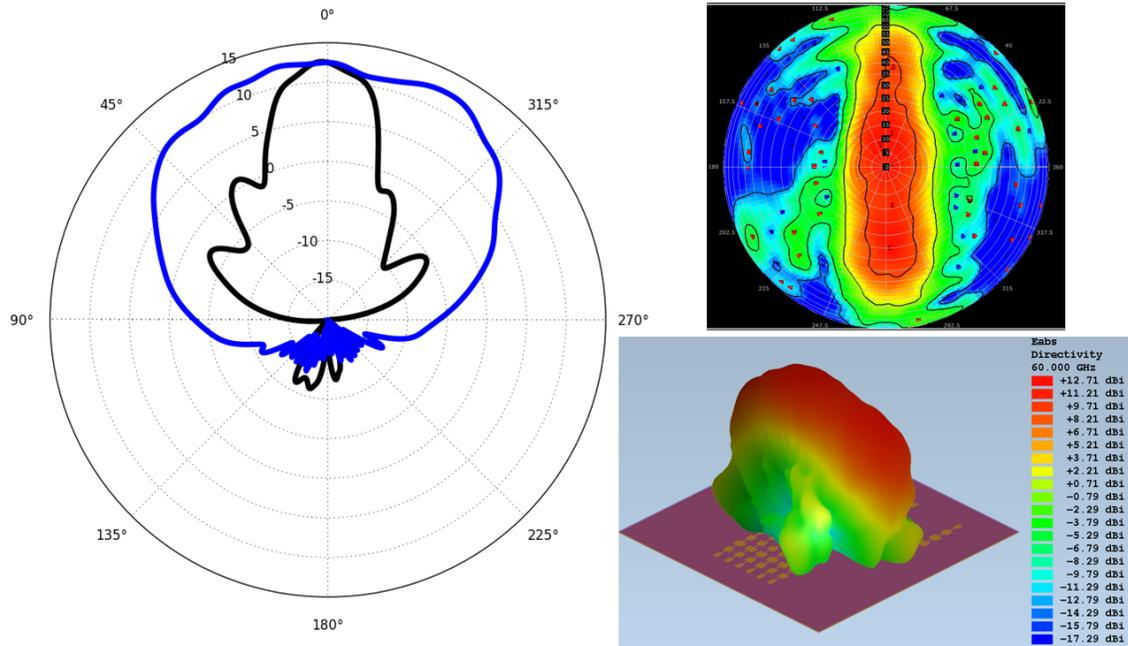
Figure 5.16: Simulation results of PCB antenna (1 x 5 patch array) of 60-GHz MIMO chip (Rx1 is excited).
