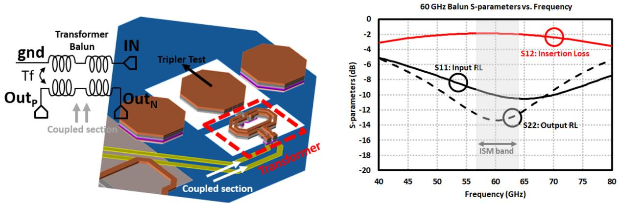
Figure 3.57: Layout and simulation results of 60-GHz balun in two-way power for frequency tripler.
