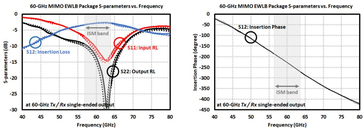
Figure 5.60: S-parameter results of single-ended 60-GHz Tx / Rx outputs in EWLb package.
