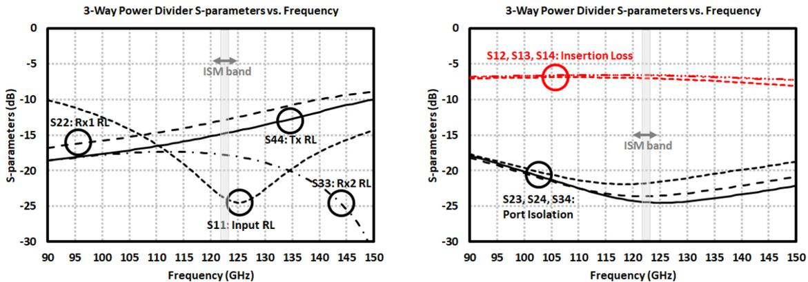
Figure 3.62: Simulation results of 122-GHz three-way power divider.
