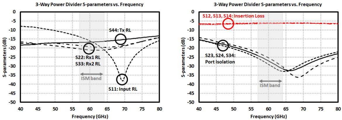
Figure 3.61: Simulation results of 60-GHz three-way power divider.
