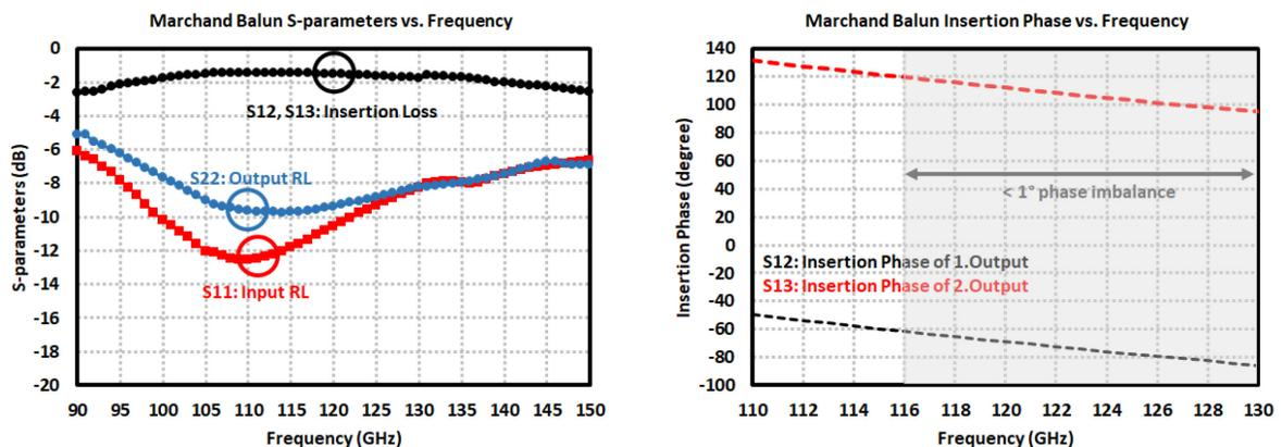
Figure 3.21: Simulation results of 122 GHz Marchand balun.
