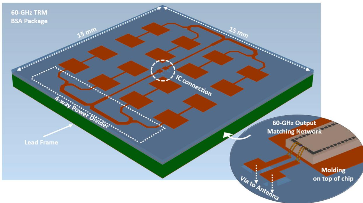
Figure 5.31: 60-GHz TRM 15 x 15 mm<sup>2</sup> BSA package and antenna.
