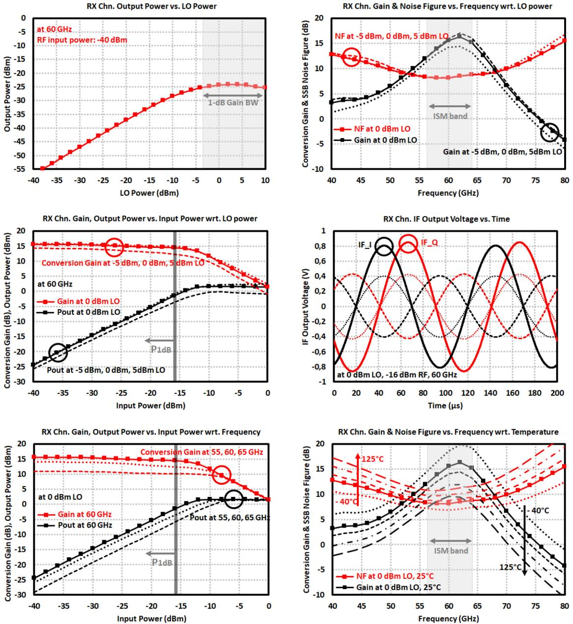
Figure 3.18: Simulation results of 60 GHz Rx channel: (*top left*) output power vs. LO power, (*top right*) conversion gain and noise figure with respect to LO power, (*middle left*) conversion gain and output power with respect to LO power, (*middle right*) IF output voltages in time domain, (*bottom left*) conversion gain and output power with respect to frequency, (*bottom right*) conversion gain and noise figure with respect to temperature.
