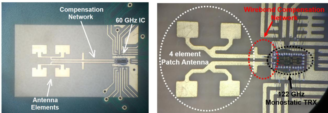
Figure 5.4: Manufactured evaluation boards with 60- / 122-GHz TRM chips and PCB antennas [15], [18].
