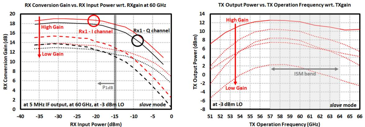
Figure 4.39: Measurement results of the 60-GHz MIMO TRx in *slave* mode where external LO is applied: (*left*) Rx channel 1 conversion gain vs. Rx input power with respect to Rx gain control voltages at -3 dBm LO input power, (*right*) Tx output power vs. frequency with respect to Tx gain control voltages at -3 dBm LO input power.
