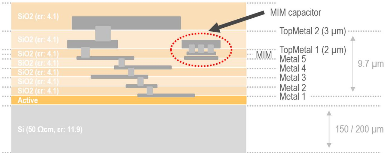
Figure 3.1: Cross section of the 7-layer SiGe BiCMOS technology.
