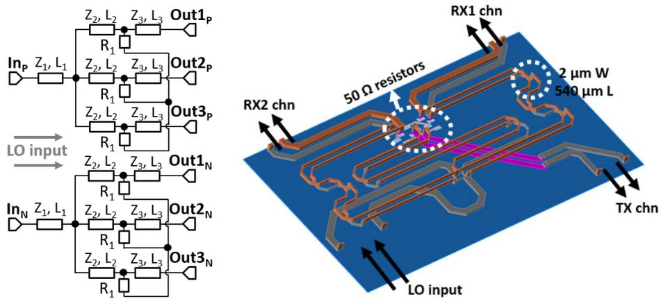
Figure 3.60: Schematic and layout of 60-GHz three-way power divider.
