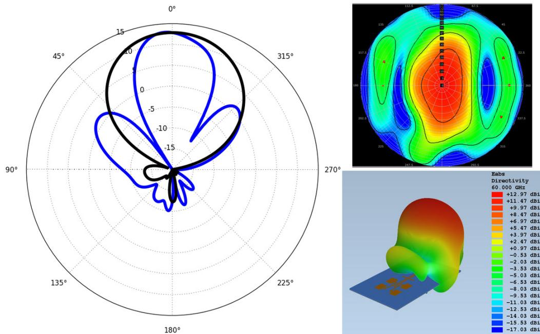
Figure 5.5: Simulation results of PCB antenna of 60-GHz TRM chip including wirebond compensation network.
