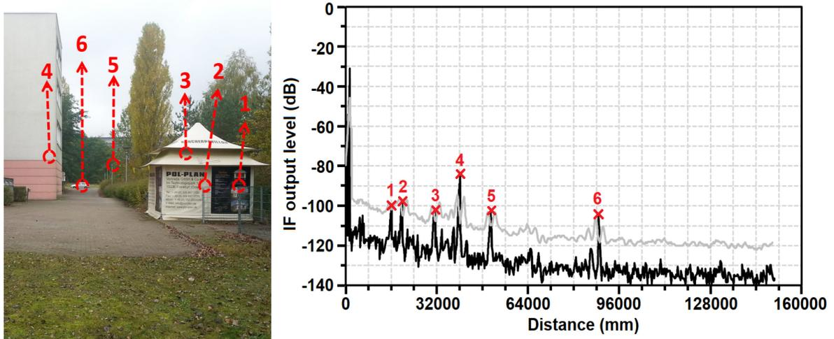
Figure 6.7: Outdoor measurement using the radar board of 60-GHz TRM including the lens with the farthest available target being the mid-sized vehicle at 90 m [18].
