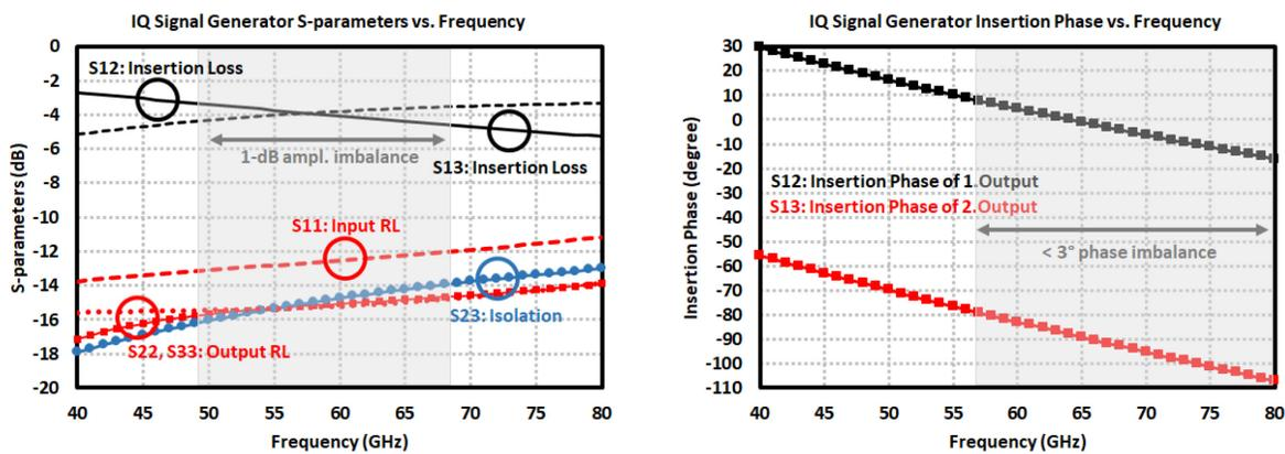
Figure 3.12: Simulation results of 60 GHz differential I/Q signal generator: (left) S-parameters, (right) insertion phase at the divider outputs.
