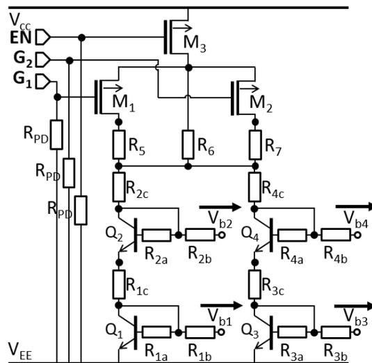
Figure 3.4: Schematic of a general use bias circuit based on current mirror topology.
