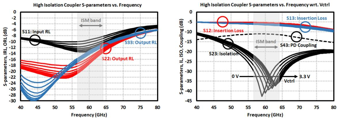
Figure 3.23: Simulation results of 60 GHz high isolation coupler: (*left*) input and output return losses, (*right*) insertion loss, isolation and coupling loss to power detector with respect to tuning voltage.
