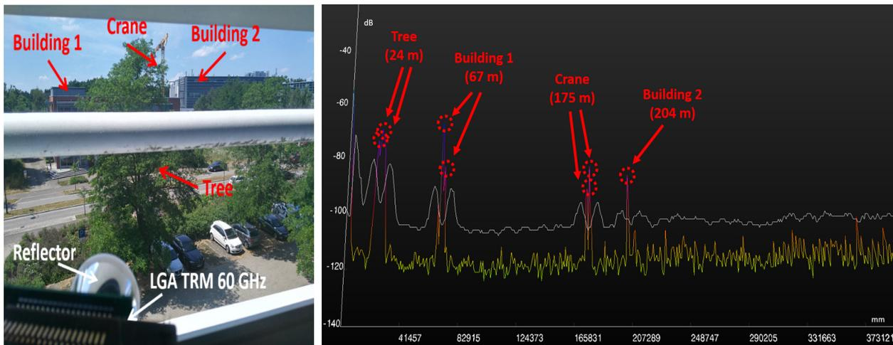
Figure 6.9: Outdoor measurement using the radar board of 60-GHz TRM in the LGA package (having 4 x 4 antennas and a reflector with 40 dB gain) with the farthest available target being the building at 204 m.
