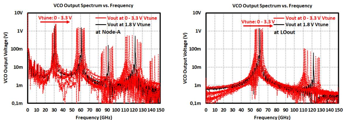
Figure 3.39: 60 GHz VCO output voltage spectrum, (*Left*) at node-A, emitter terminal, (*Right*) at *LOout* of PA.
