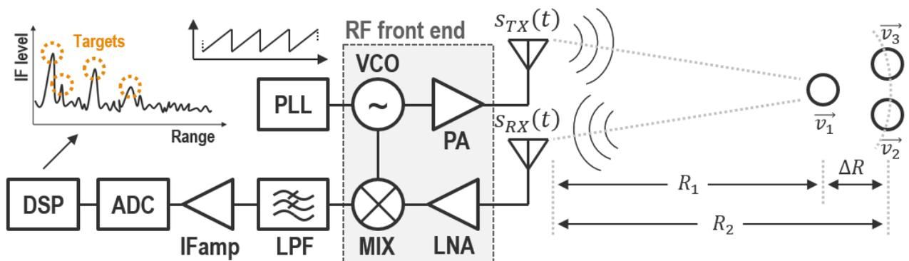
Figure 2.1: Block diagram of a typical target detecting radar system.
