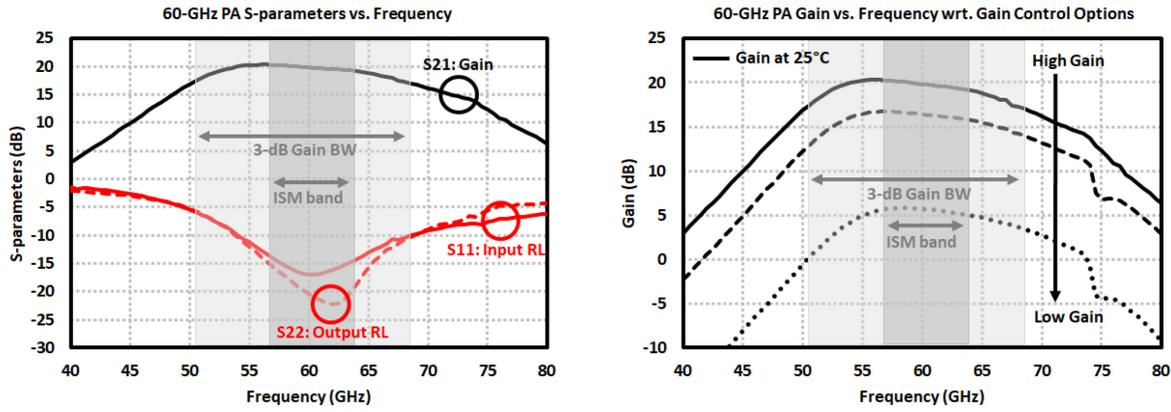
Figure 3.27: Simulation results of 60-GHz PA: (left) S-parameters, (right) gain with respect to gain control options.
