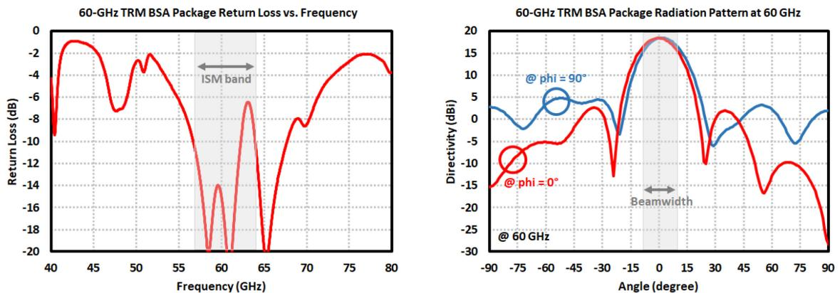
Figure 5.34: 60-GHz TRM BSA antenna simulation results (radiation pattern at 60 GHz and return loss).
