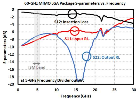
Figure 5.44: Return loss and insertion loss of 5-GHz frequency divider outputs of 60-GHz MIMO LGA package.
