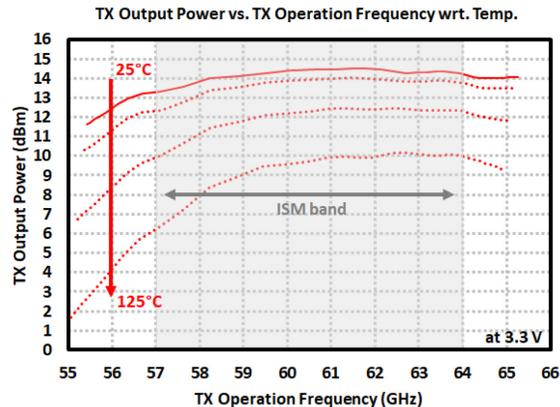
Figure 4.5: Measurement results of the 60-GHz TR2 TRx: Tx output power vs. frequency with respect to temperature.
