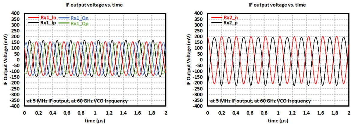
Figure 4.37: Measurement results of the 60-GHz MIMO TR<sub>x</sub>: 5-MHz IF output voltages at 60 GHz (left) from quadrature Rx channel 1, and (right) Rx channel 2.
