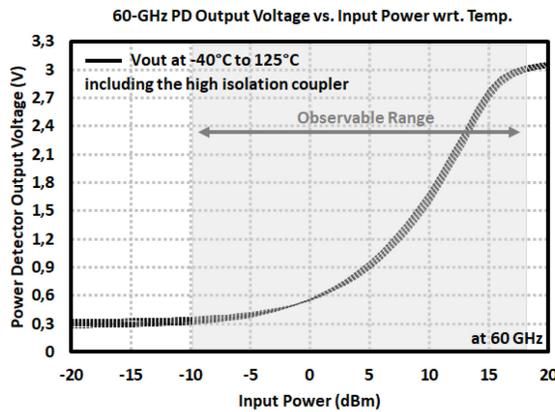
Figure 3.34: Power detector output voltage with respect to temperature.
