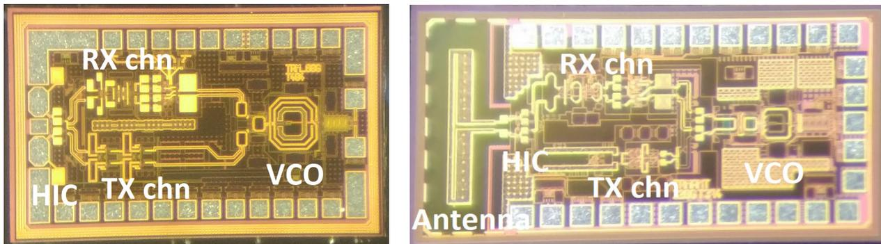
Figure 4.26: Photo of the fabricated 122-GHz TRM and TRMant transceiver chips occupying  $1.35 \text{ mm} \times 0.76 \text{ mm}$  and  $1.49 \text{ mm} \times 0.73 \text{ mm}$  area.
