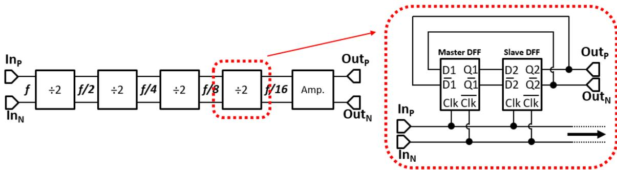
Figure 3.43: Block diagram of the divide-by-16 frequency divider and its divide-by-2 master / slave DFF sub-block.
