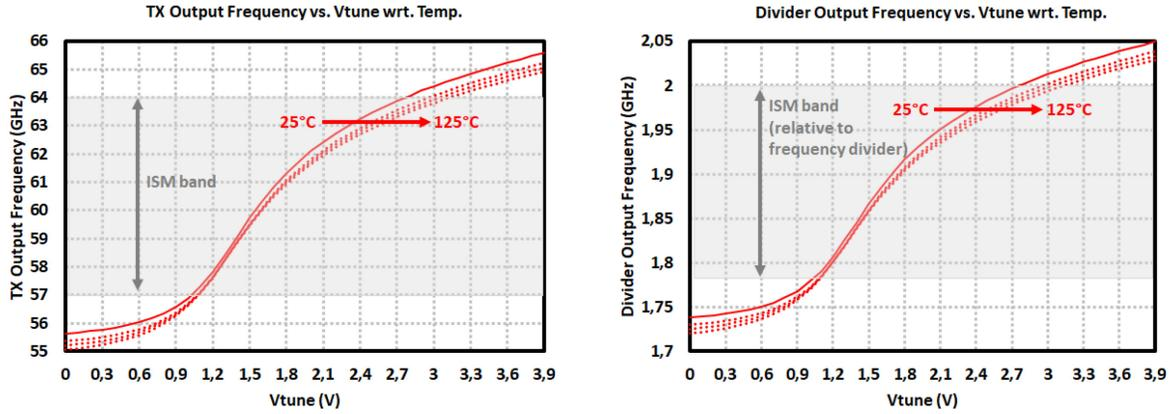
Figure 4.23: Measurement results of the 60-GHz TRM TRx: (left) Tx output frequency and (right) Frequency Divider output frequency vs. VCO tuning voltages with respect to temperature.
