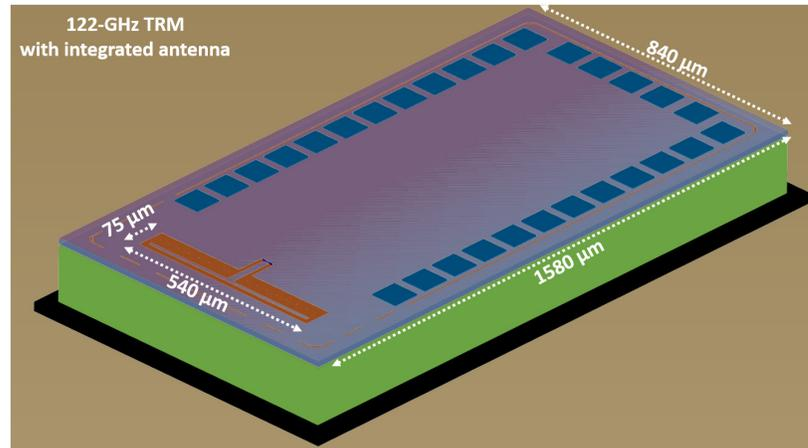
Figure 5.19: 122-GHz TRMant chip.
