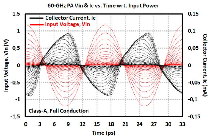
Figure 3.25: Class-A PA collector current and input voltage for swept input power levels for the fabricated 60-GHz PA.
