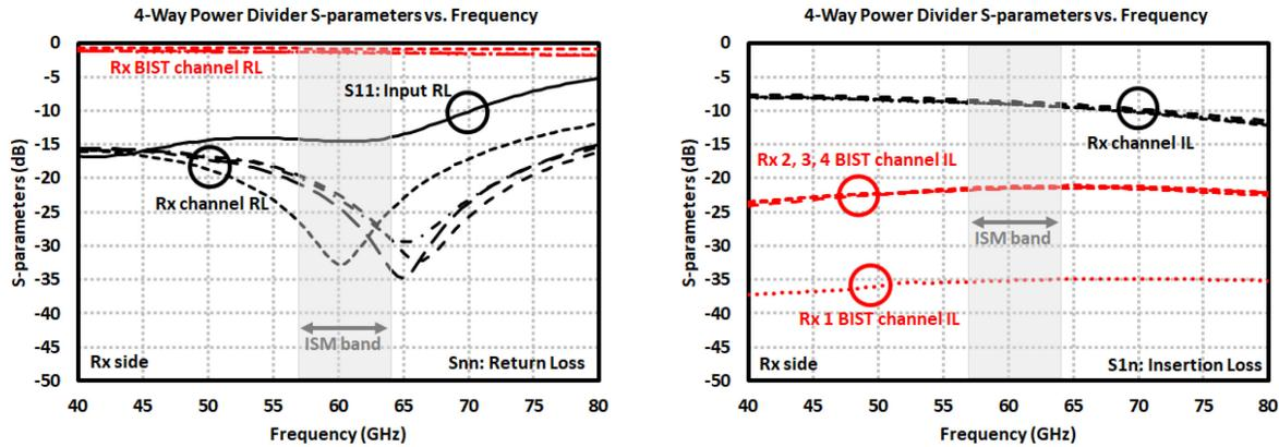
Figure 3.64: Simulation results of 60-GHz four-way power divider on Rx side.
