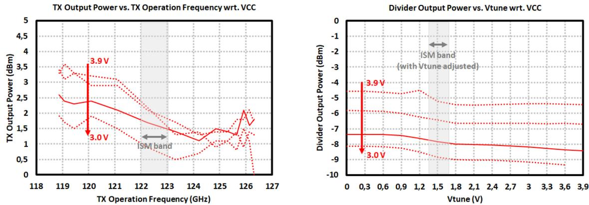
Figure 4.13: Measurement results of the 122-GHz TR2 TRx: (*left*) Tx output power vs. frequency, and (*right*) Frequency Divider output power vs. VCO tuning voltages with respect to changing supply voltages between 3.0 V – 3.9 V.
