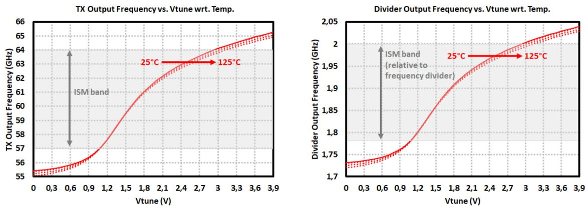
Figure 4.6: Measurement results of the 60-GHz TR2 TRx: (*left*) Tx output frequency and (*right*) Frequency Divider output frequency vs. VCO tuning voltages with respect to temperature.
