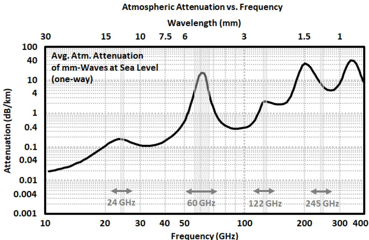
Figure 1.1: One-way average atmospheric attenuation of mm-Wave frequencies at sea level highlighting the common ISM bands.
