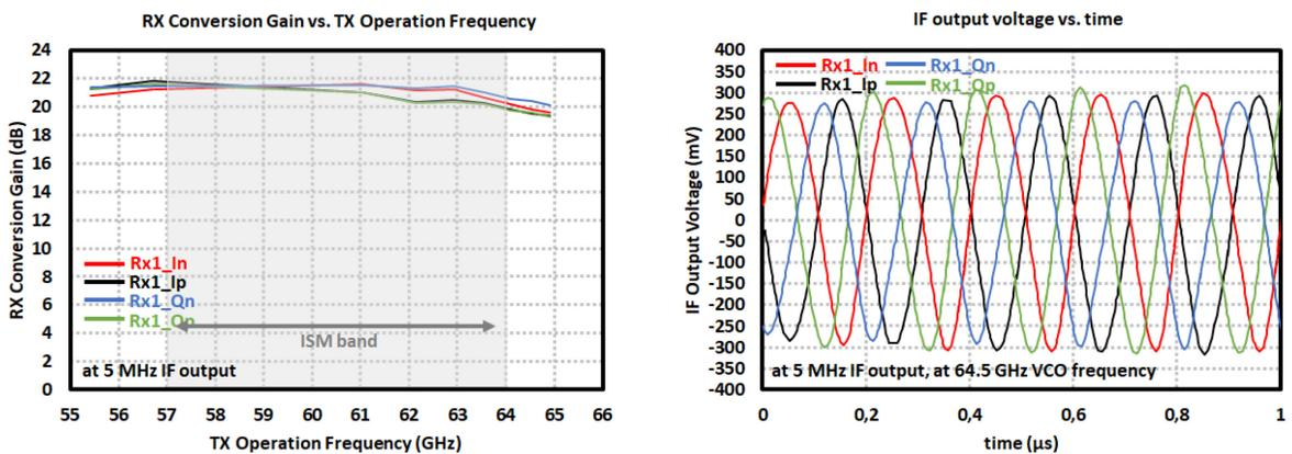
Figure 4.8: Measurement results of the 60-GHz TR2 TRx: (*left*) Rx channel 1 conversion gain vs. frequency, (*right*) 5-MHz IF output voltages at 64.5 GHz.
