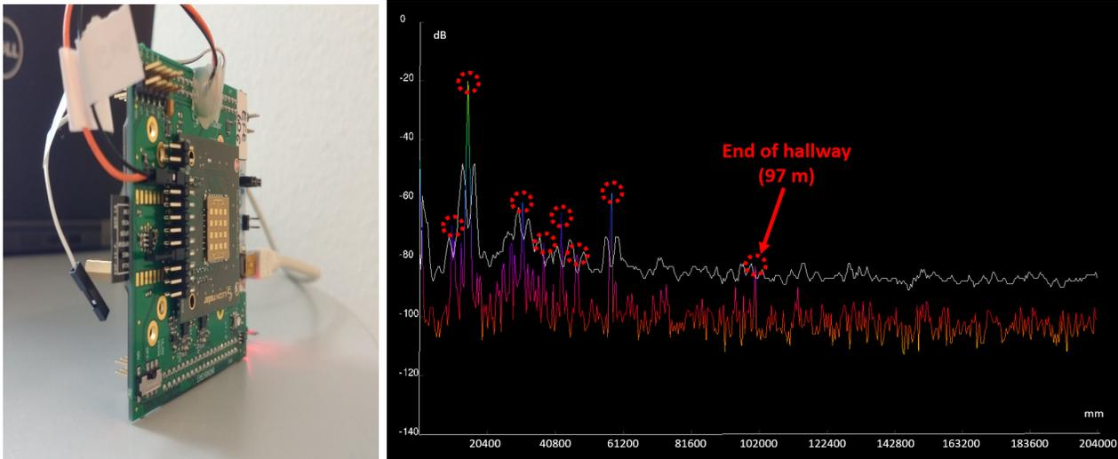
Figure 6.8: Complex indoor measurement using the radar board of 60-GHz TRM in the BSA package (having 4 x 4 antennas and excluding the lens) with the farthest available target being the metallic door at 97 m.
