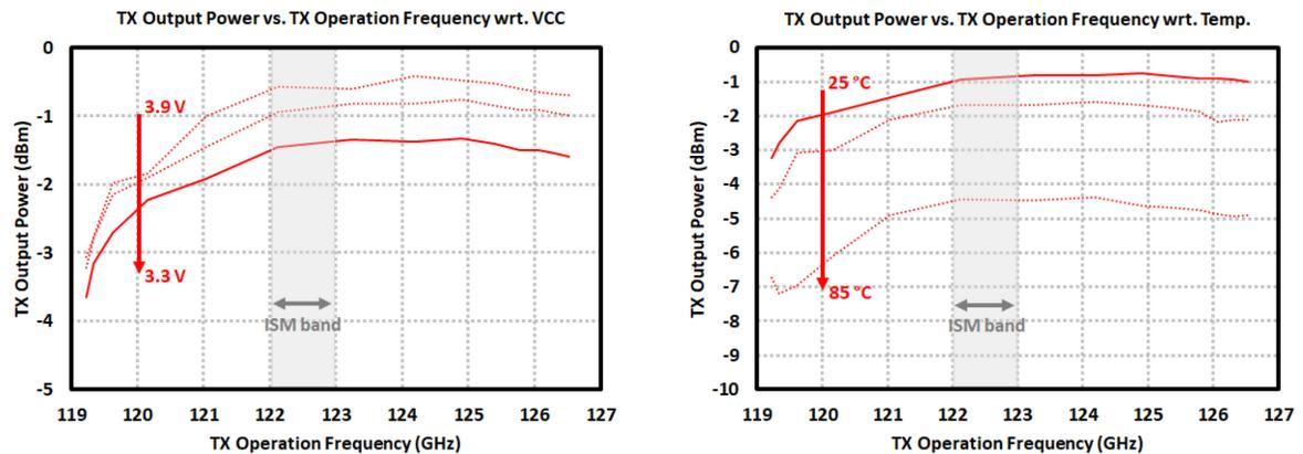
Figure 4.28: Measurement results of the 122-GHz TRM TRx: (*left*) Tx output power vs. frequency with respect to changing supply voltages between 3.3 V – 3.9 V, (*right*) Tx output power vs. frequency with respect to temperature.
