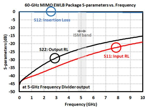
Figure 5.57: S-parameter simulation results of differential 5-GHz frequency divider outputs in EWLB package.
