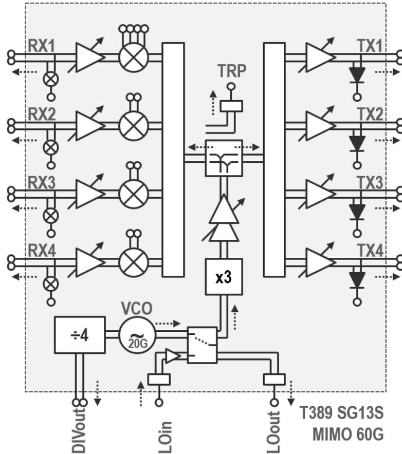
Figure 2.6: Block diagram of the 60-GHz MIMO TRx with 4-Tx and 4-Rx channels [19].
