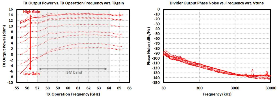
Figure 4.7: Measurement results of the 60-GHz TR2 TRx: (*left*) Tx output power vs. frequency with respect to Tx gain control voltages 0 V – 3.3 V, (*right*) Frequency Divider phase noise with respect to VCO tuning voltages.
