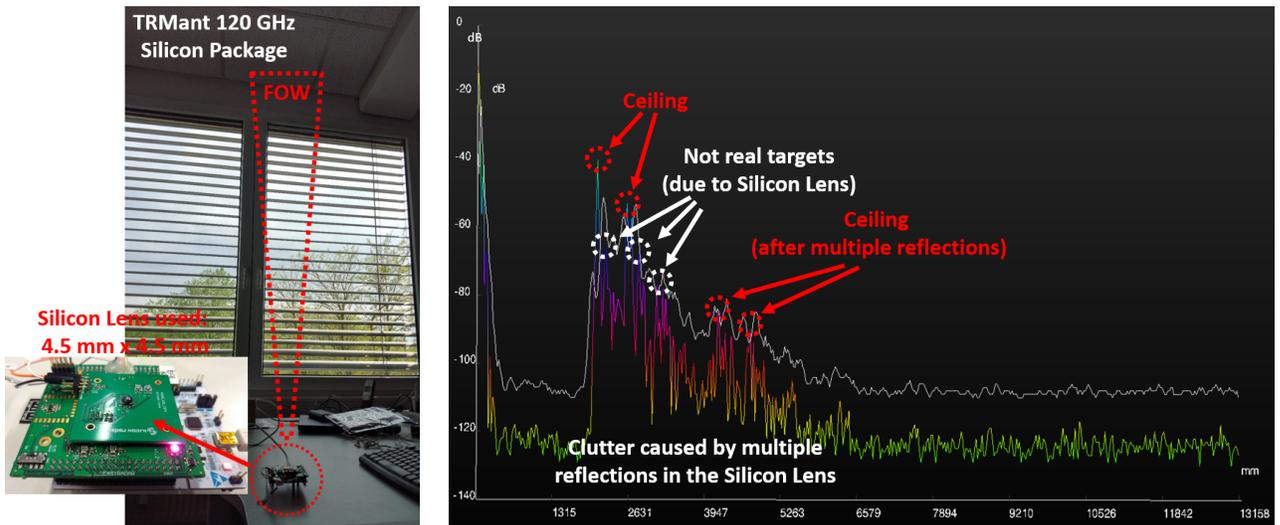
Figure 5.27: Simple indoor measurement using the radar board of 122-GHz TRMant Silicon package including the hemispherical Silicon lens having 4.5 mm diameter directed towards the office ceiling.
