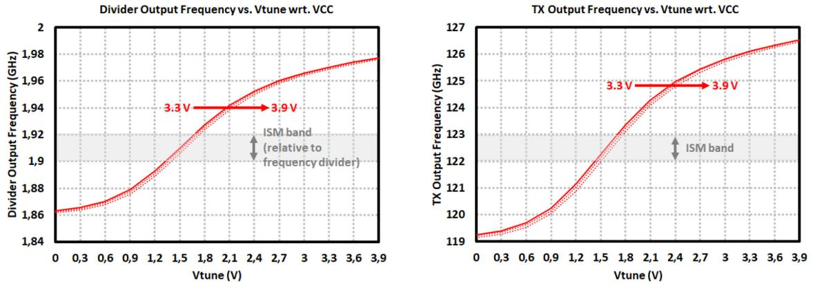
Figure 4.27: Measurement results of the 122-GHz TRM TRx: (*left*) Tx output frequency and (*right*) Frequency Divider output frequency vs. VCO tuning voltages with respect to changing supply voltages between 3.3 V – 3.9 V.
