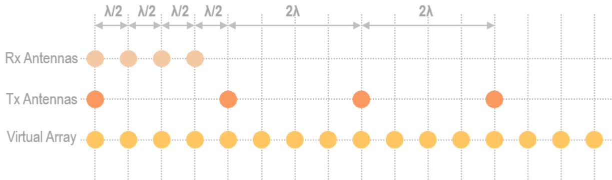
Figure 5.12: Illustration of one-dimensional 1 x 16 MIMO virtual array formation.
