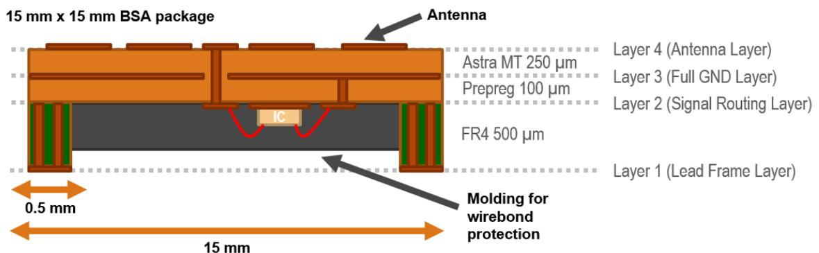
Figure 5.30: 60-GHz TRM BSA package PCB stack-up.
