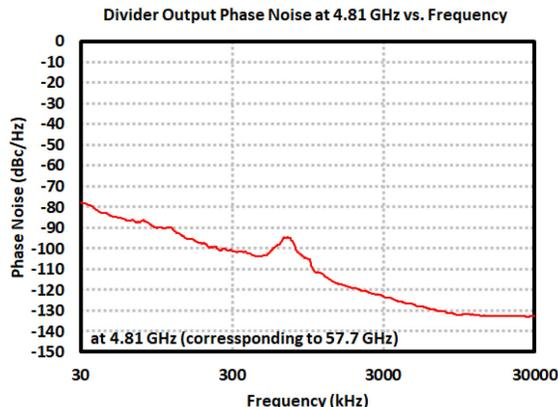
Figure 4.40: Measurement results of the 60-GHz MIMO TRx in *master* mode where internal VCO is enabled: Frequency Divider phase noise at 4.81 GHz (corresponding to Tx operation frequency of 57.7 GHz).
