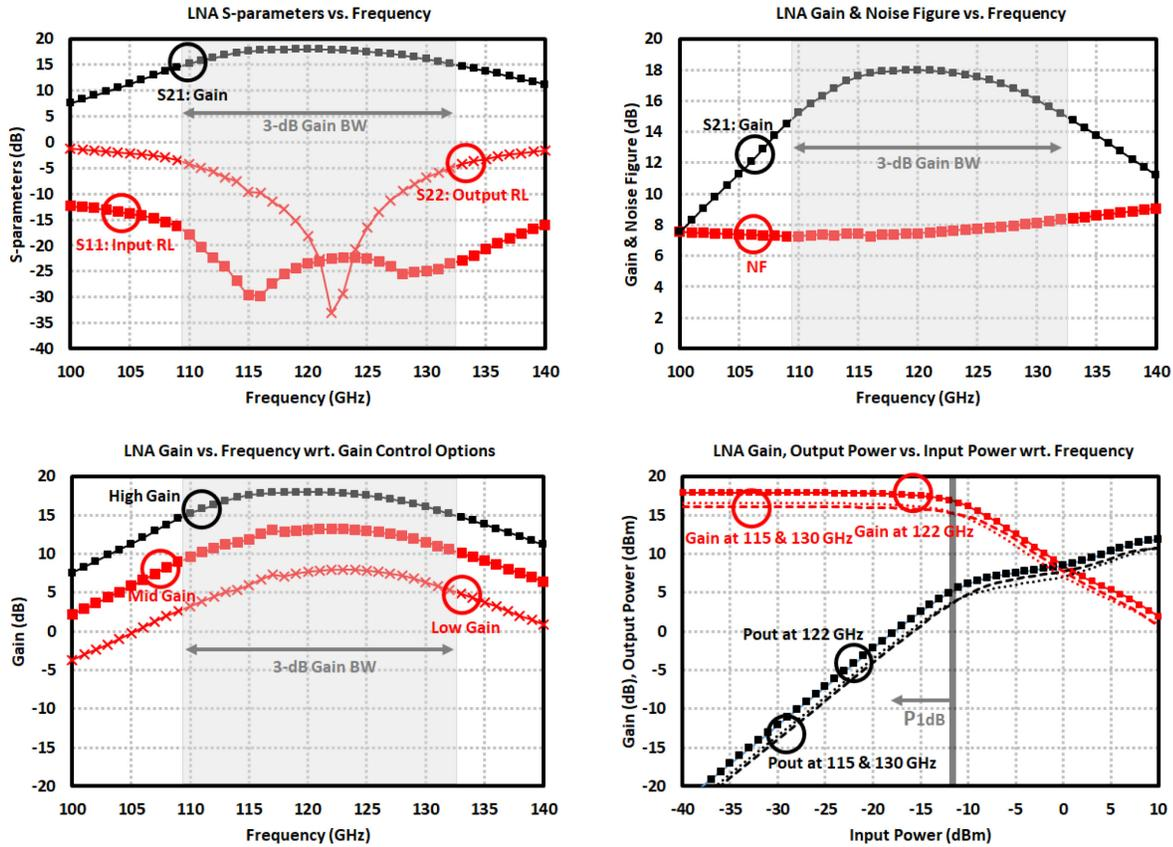
Figure 3.8: Simulation results of 122 GHz LNA: (*top left*) S-parameters, (*top right*) gain and noise figure, (*bottom left*) gain with respect to control options, (*bottom right*) gain and output power with respect to frequency.
