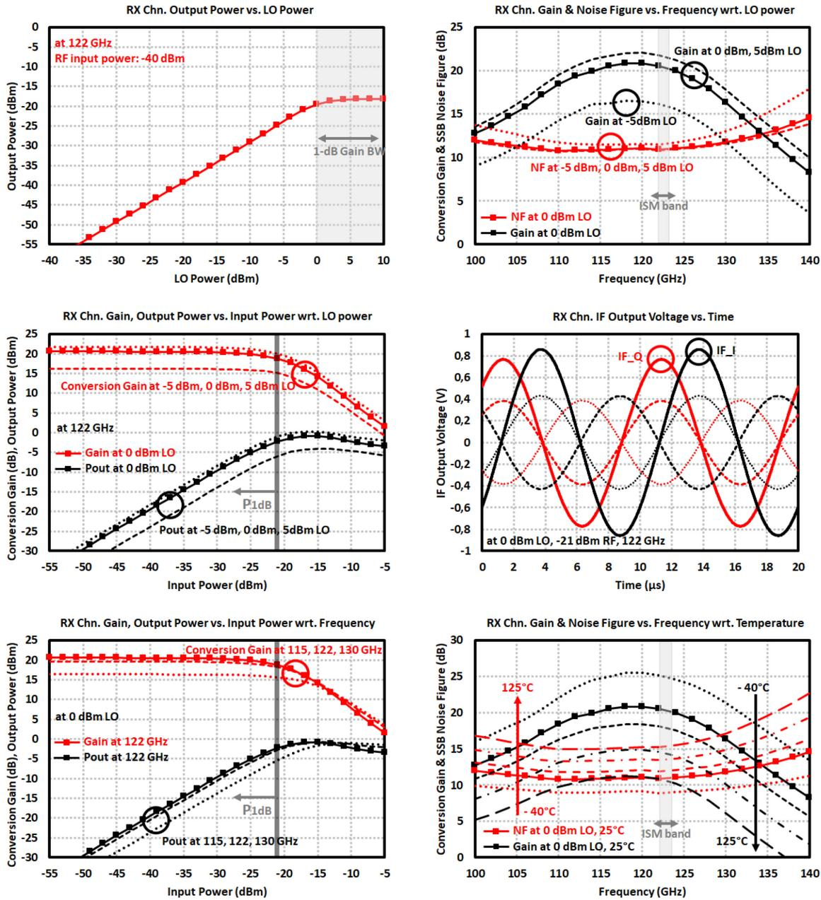
Figure 3.19: Simulation results of 122 GHz Rx channel: (top left) output power vs. LO power, (top right) conversion gain and noise figure with respect to LO power, (middle left) conversion gain and output power with respect to LO power, (middle right) IF output voltages in time domain, (bottom left) conversion gain and output power with respect to frequency, (bottom right) conversion gain and noise figure with respect to temperature.
