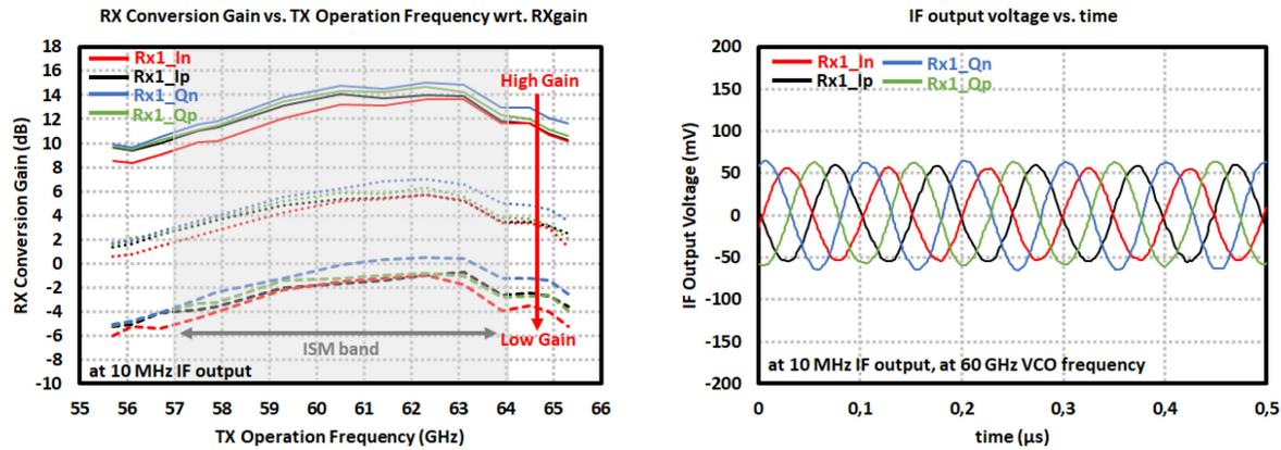
Figure 4.25: Measurement results of the 60-GHz TRM TRx: (left) Rx channel conversion gain vs. frequency with respect to Rx gain control voltages, (right) 10-MHz IF output voltages at 60 GHz.
