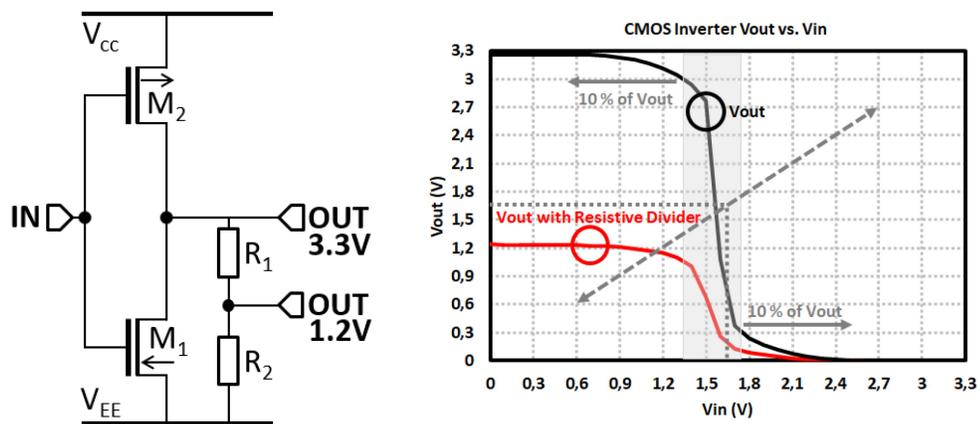
Figure 3.5: Schematic and simulation results of a CMOS inverter.
