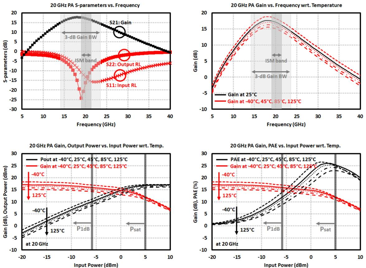
Figure 3.56: Simulation results of 20 GHz PA: (top left) S-parameters, (top right) gain with respect to temperature, (bottom left) gain and output power with respect to temperature, (bottom right) gain and PAE with respect to temperature.
