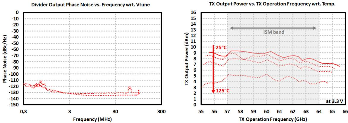
Figure 4.22: Measurement results of the 60-GHz TRM TRx: (*left*) Frequency Divider phase noise at 1.74 GHz and 2.05 (corresponding to Tx operation frequencies of 55.6 GHz and 65.6 GHz), (*right*) Tx output power vs. frequency with respect to temperature.
