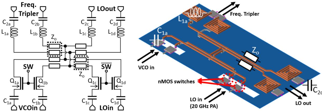
Figure 3.46: Schematic and layout of 20-GHz differential multiplexer.
