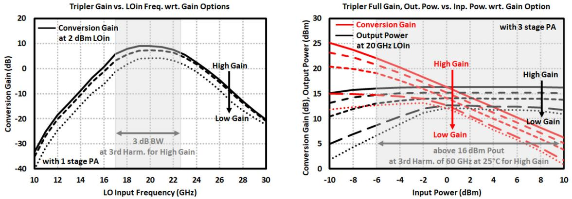
Figure 3.52: Simulation results of frequency tripler including a single-stage PA. Conversion gain and output power with respect to input power for the 3<sup>rd</sup> harmonic of 20 GHz LO input at different temperatures.
