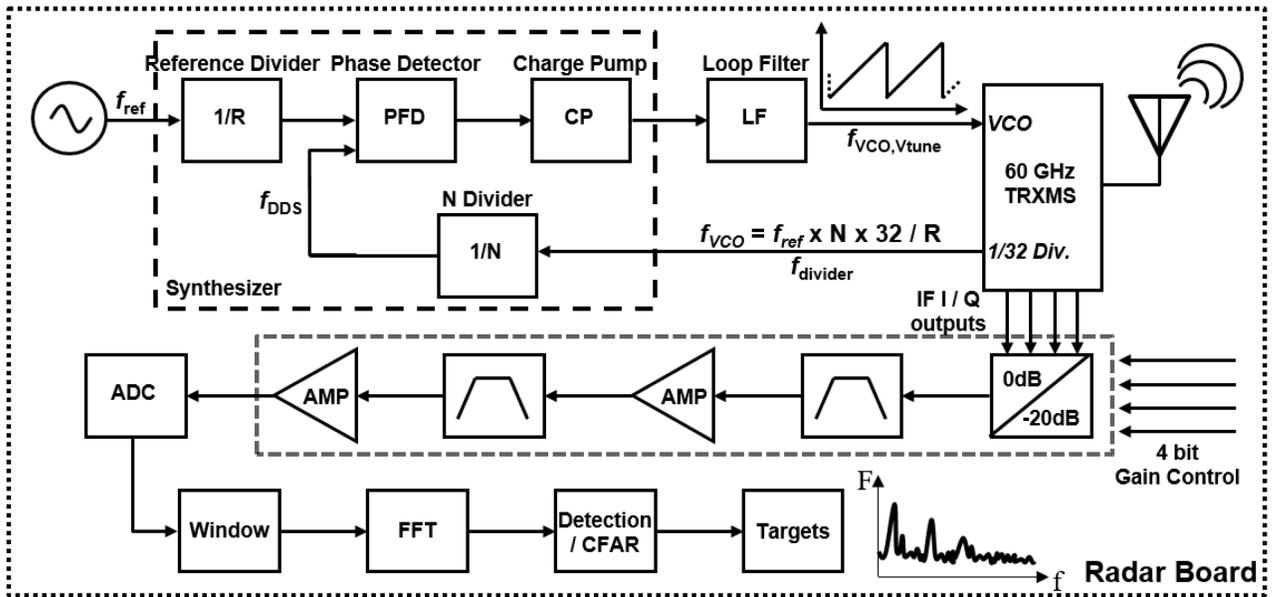
Figure 6.1: Block diagram of radar signal processing evaluation board [18].
