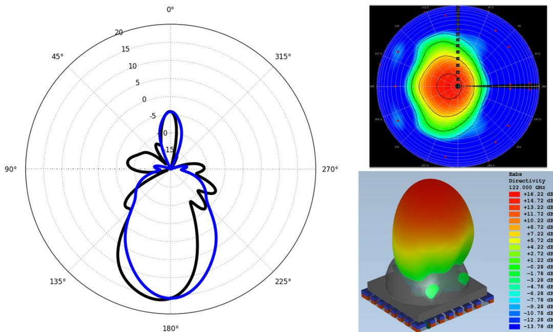
Figure 5.25: 122-GHz TRMant Silicon package antenna simulation results.
