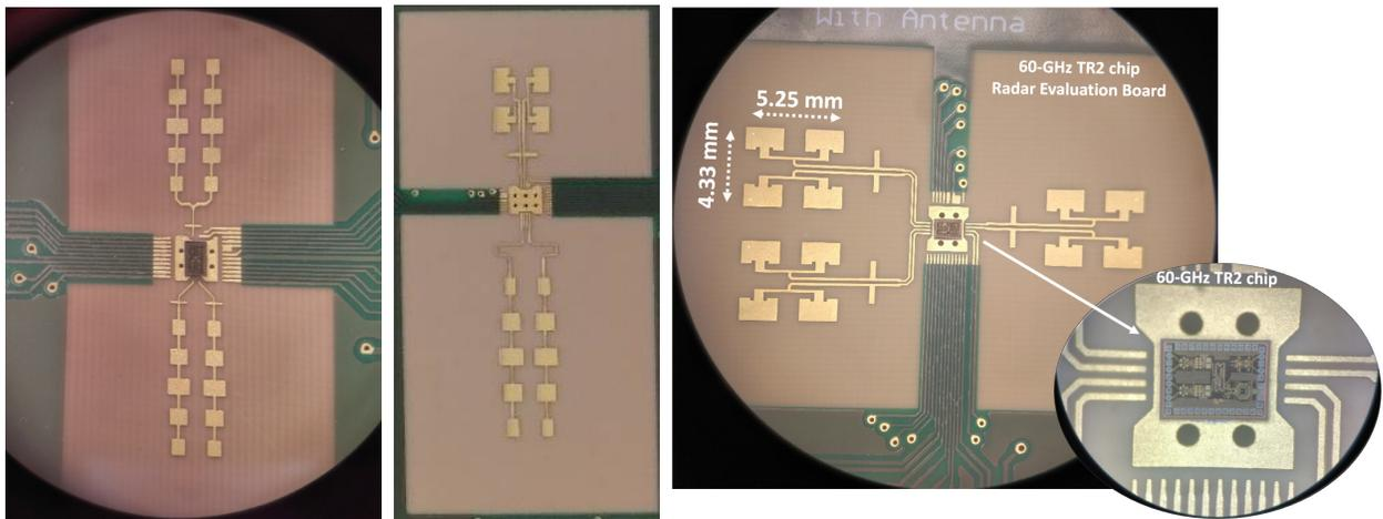
Figure 5.9: Manufactured evaluation boards and PCB antennas with (*left*) 122-GHz TR2 (1 x 5 patch array), (*middle*) 60-GHz TR2 (1 x 5 patch array), (*right*) 60-GHz TR2 (2 x 2 patch array).
