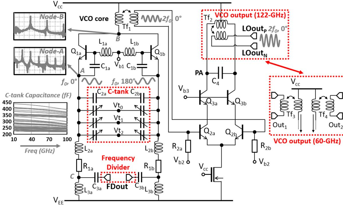
Figure 3.36: Schematic of 60 GHz VCO integrated to a PA and a Frequency Divider.
