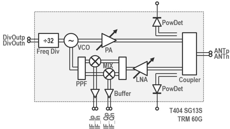
Figure 2.3: Block diagram of the single-channel monostatic 60-GHz TRx.
