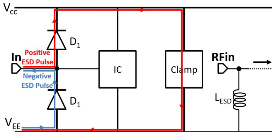
Figure 3.3: Concept of ESD protection at low- and high-frequency pads.
