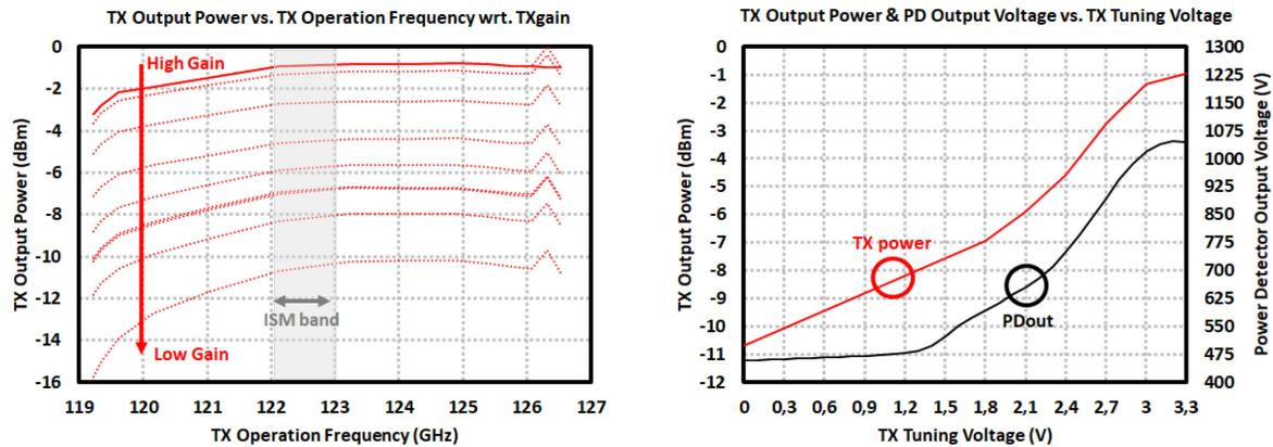
Figure 4.29: Measurement results of the 122-GHz TRM TRx: (*left*) Tx output power vs. frequency with respect to Tx gain control voltages, (*right*) Tx output power and Power Detector output voltage vs. Tx gain tuning voltages.
