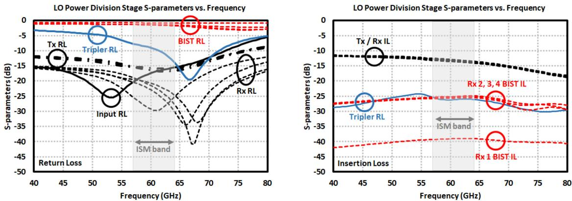
Figure 3.65: Simulation results of 60-GHz combined LO power division stage.
