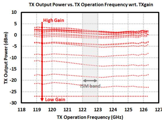
Figure 4.14: Measurement results of the 122-GHz TR2 TRx: Tx output power vs. frequency with respect to Tx gain control voltages 0 V – 3.3 V.
