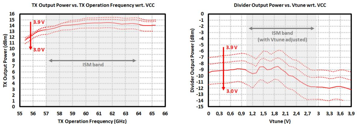
Figure 4.4: Measurement results of the 60-GHz TR2 TRx: (left) Tx output power vs. frequency, and (right) Frequency Divider output power vs. VCO tuning voltages with respect to changing supply voltages between 3.0 V – 3.9 V.
