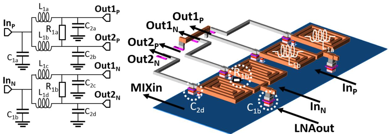
Figure 3.9: Schematic and layout of 60 GHz differential LC Wilkinson Power Divider.
