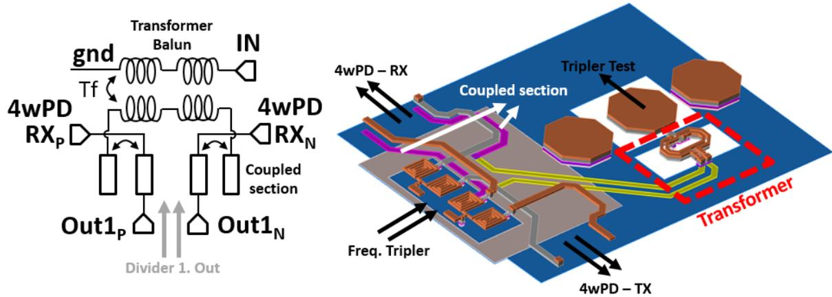
Figure 3.58: Schematic and layout of 60-GHz two-way power divider with a coupled output for frequency tripler.
