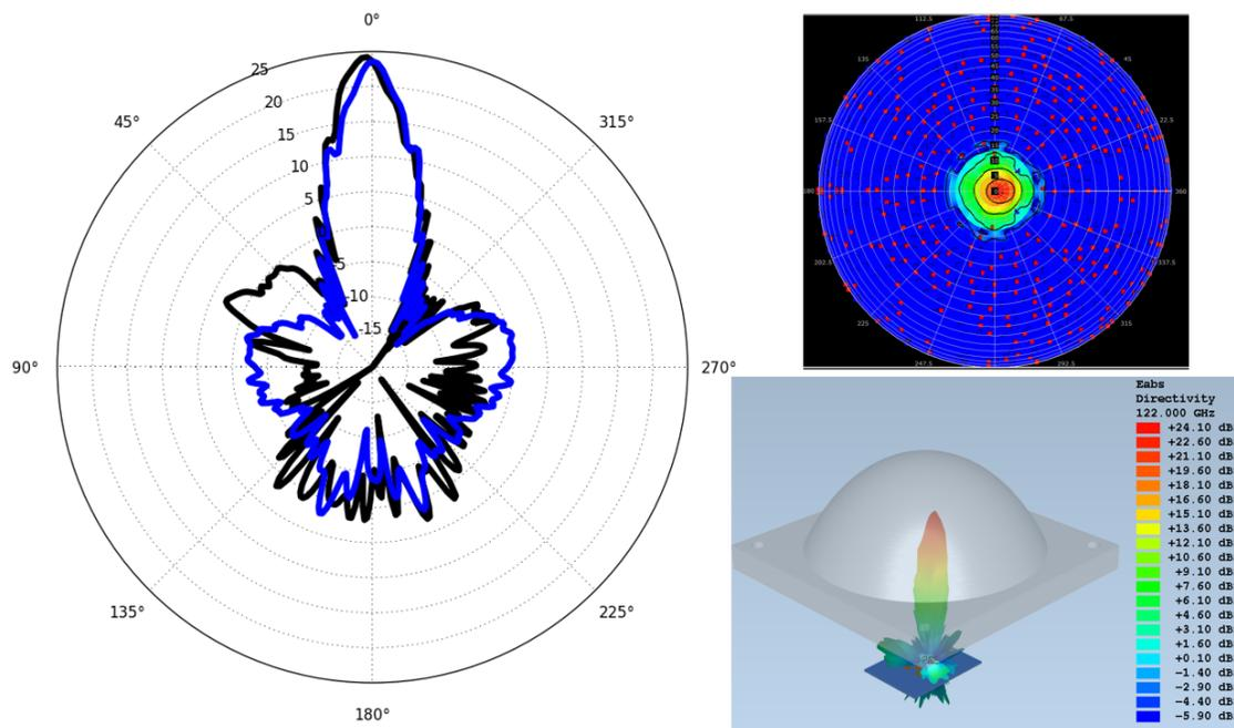
Figure 5.8: Simulation results of PCB antenna of 122-GHz TRM chip including HDPE plastic lens at 1.5 cm.
