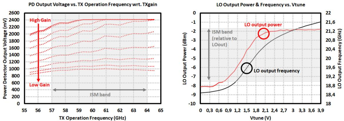
Figure 4.34: Measurement results of the 60-GHz MIMO TRx in *master* mode where internal VCO is enabled: (left) Power Detector output voltage vs. frequency with respect to Tx gain control voltages 0 V – 3.3 V, (right) *LOout* output power and frequency vs. VCO tuning voltages.
