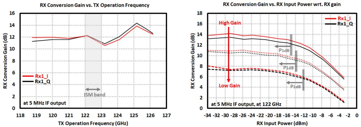
Figure 4.16: Measurement results of the 122-GHz TR2 TRx: Rx channel 1 conversion gain (left) vs. frequency, and (right) vs. Rx input power with respect to Rx gain control voltages at 122 GHz.
