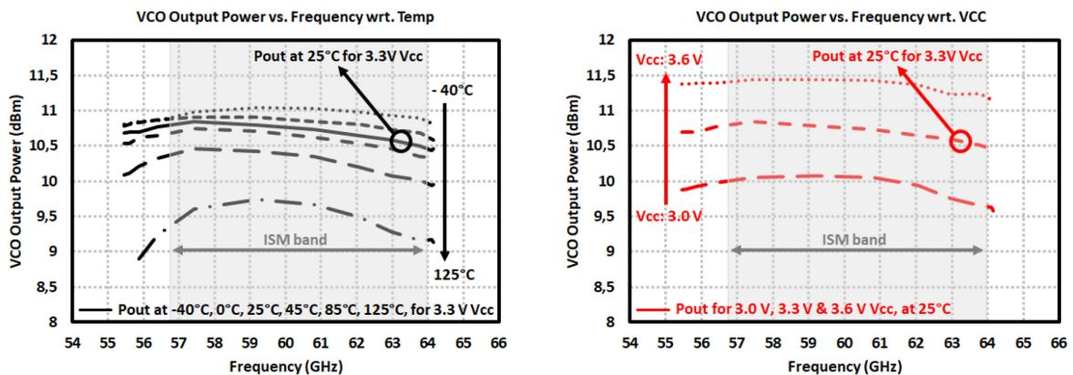
Figure 3.40: 60 GHz VCO output power with respect to swept tuning voltages for different (*Left*) operation temperature and (*Right*) supply pushing / pulling.
