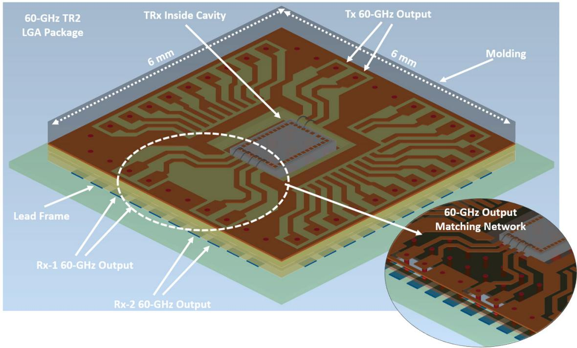
Figure 5.41: Simulated 60-GHz TR2 6 x 6 mm<sup>2</sup> LGA package structure.
