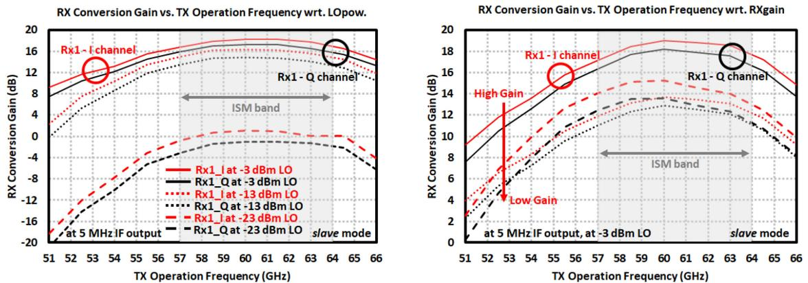
Figure 4.38: Measurement results of the 60-GHz MIMO TRx in *slave* mode where external LO is applied: (*left*) Rx channel 1 conversion gain vs. frequency with respect to applied LO power from *LOin* pad, and (*right*) Rx channel 1 conversion gain vs. frequency with respect to Rx gain control voltages at -3 dBm LO input power.
