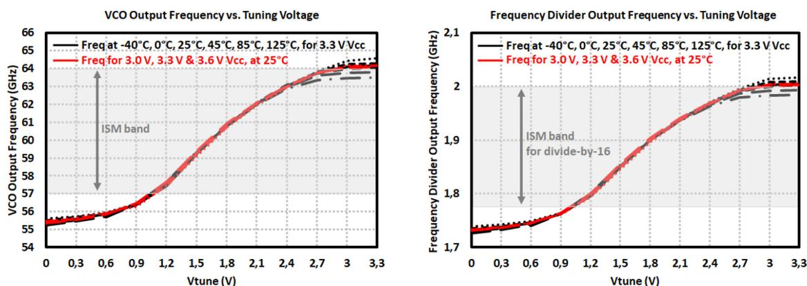
Figure 3.41: 60 GHz VCO with respect to swept tuning voltages for different operation temperature and supply pushing / pulling, (Left) LO output frequency, (Right) frequency divider output frequency.
