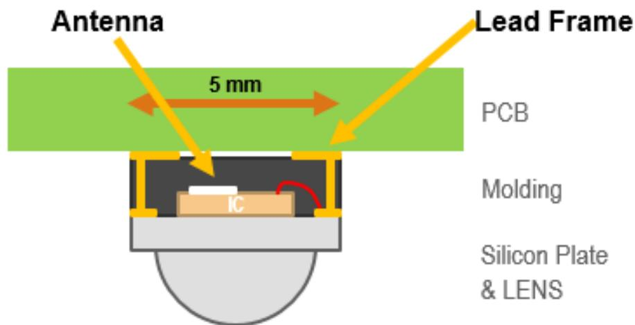
Figure 5.23: 60-GHz TRMant Silicon package with integrated Silicon-lens stack-up.
