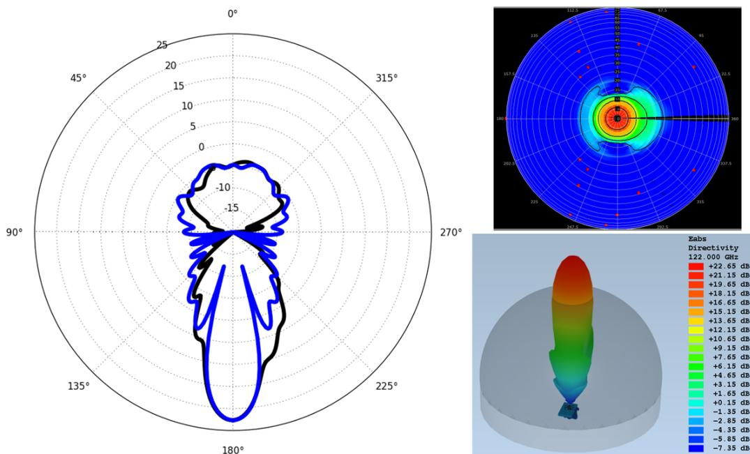
Figure 5.21: Simulation results of 122-GHz TRMant chip with Silicon-lens of 2.0 mm additional height and 5.5 mm radius.
