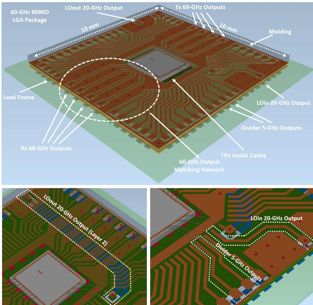
Figure 5.43: Simulated 60-GHz MIMO 10 x 10 mm<sup>2</sup> LGA package structure.
