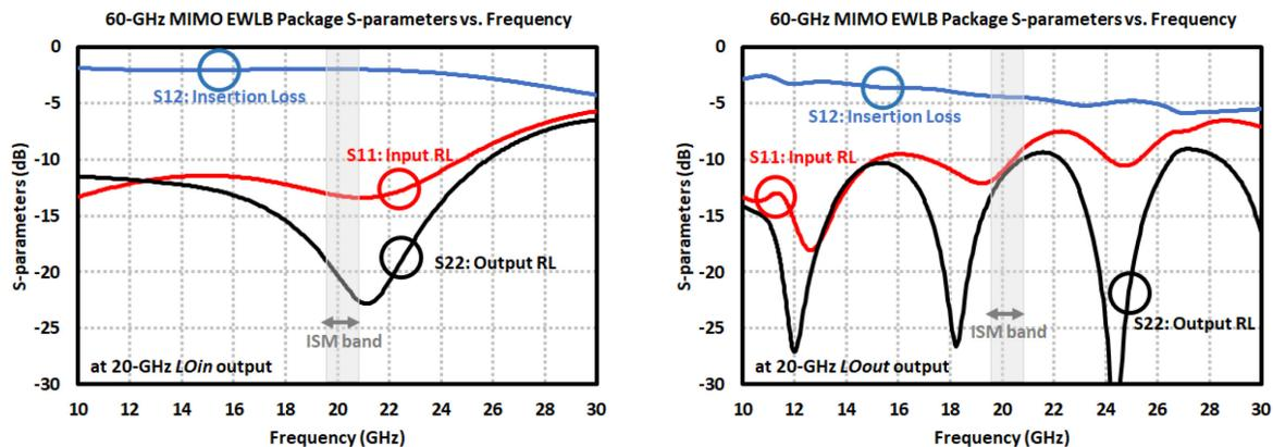
Figure 5.58: S-parameter results of single-ended 20-GHz (*left*) LOin and (*right*) LOout outputs in EWLb package.
