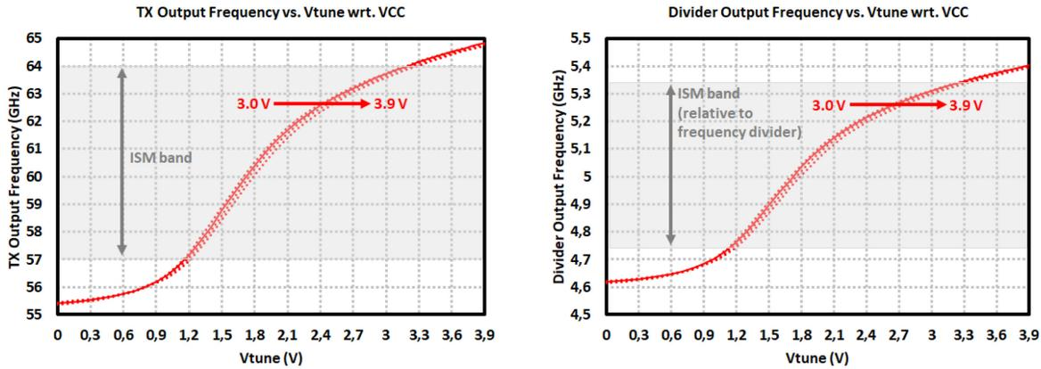
Figure 4.32: Measurement results of the 60-GHz MIMO TRx in *master* mode where internal VCO is enabled: (left) Tx output frequency and (right) Frequency Divider output frequency vs. VCO tuning voltages with respect to changing supply voltages between 3.0 V – 3.9 V.
