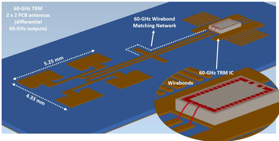
Figure 5.1: PCB antenna concepts of 60-GHz TRM chips including wirebond compensation network.
