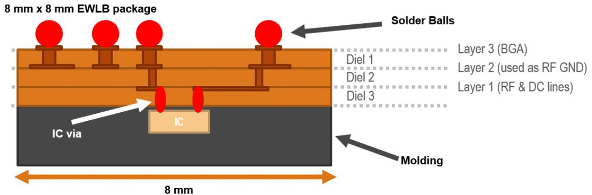
Figure 5.52: 60-GHz MIMO EWL B package stack-up.
