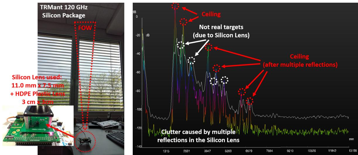
Figure 5.28: Simple indoor measurement using the radar board of 122-GHz TRMant Silicon package including the hemispherical Silicon lens having 4.5 mm diameter and additional 3 cm x 3 cm HDPE lens on top directed towards the office ceiling.
