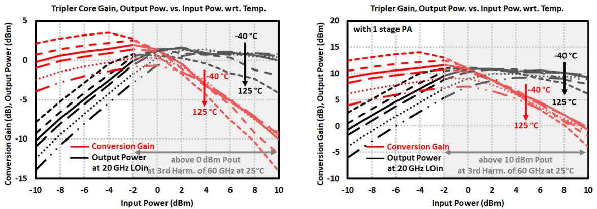
Figure 3.53: Conversion gain and output power with respect to input power for the 3<sup>rd</sup> harmonic of 20 GHz LO input at different temperatures for (left) tripler core, (right) tripler with single-stage PA.
