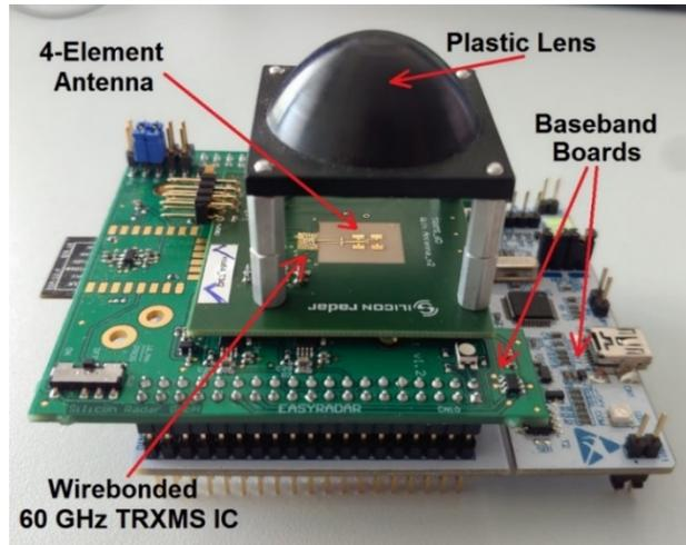
Figure 6.3: FMCW radar evaluation board demonstrated using 60-GHz TRM IC with the simulated 3 cm x 3 cm Lens [18].
