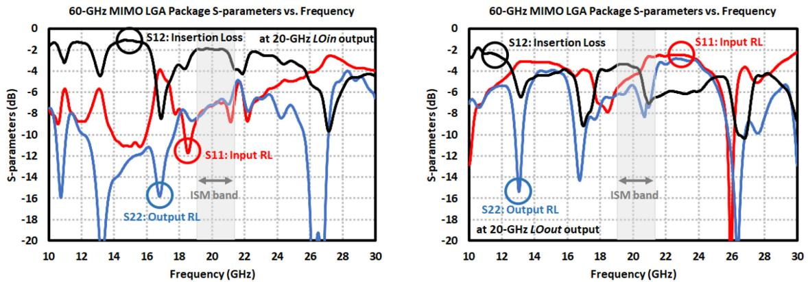
Figure 5.45: Return loss and insertion loss of 20-GHz  $LO_{in}$  and  $LO_{out}$  outputs of 60-GHz MIMO LGA package.
