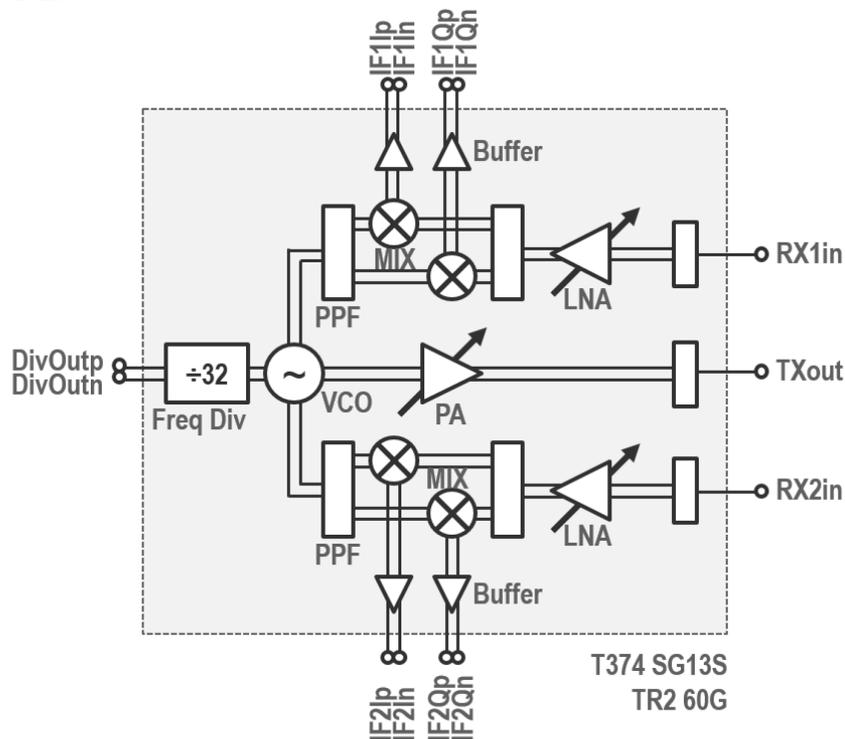
Figure 2.5: Block diagram of the double-receive-channel 60-GHz TRx.
