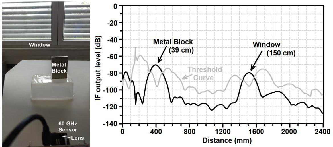
Figure 6.4: Simple indoor measurement using the radar board of 60-GHz TRM including the lens [18].
