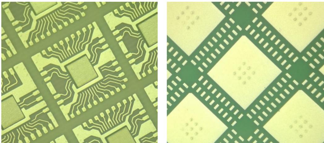
Figure 5.37: 60-GHz TR2 6 x 6 mm<sup>2</sup> LGA package, top (RF and DC connections) and bottom (lead frame).
