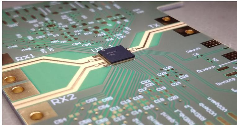
Figure 5.49: 60-GHz TR2 6 x 6 mm<sup>2</sup> LGA package mounted on the designed evaluation board.
