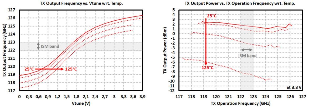
Figure 4.15: Measurement results of the 122-GHz TR2 TRx: (left) Tx output frequency vs. VCO tuning voltages, and (right) Tx output power vs. frequency with respect to temperature.
