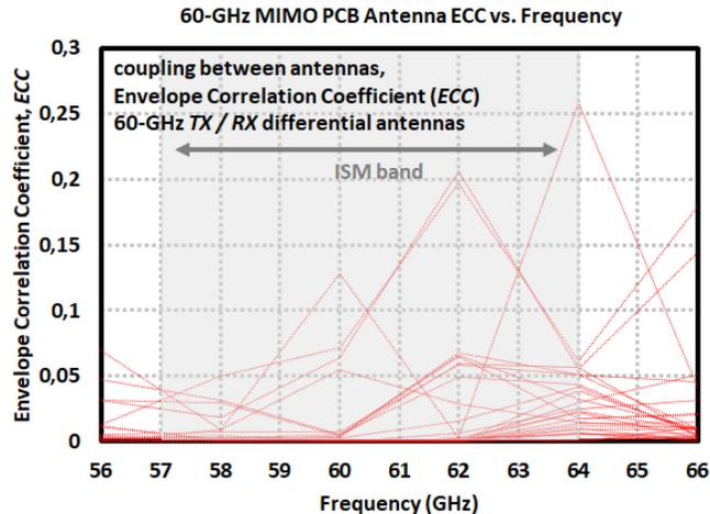
Figure 5.18: Simulation results of PCB antenna (1 x 5 patch array) of 60-GHz MIMO chip showing MIMO Envelope Correlation Coefficients (*ECC*) between each antenna.
