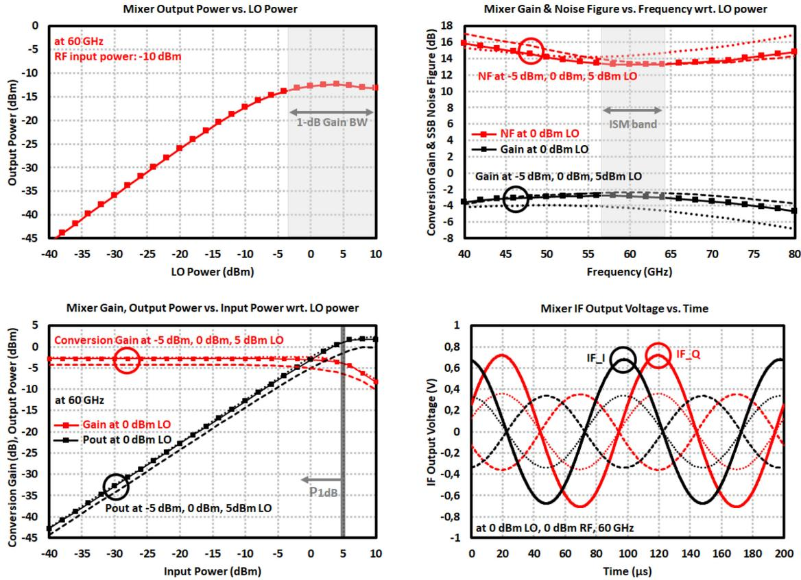
Figure 3.15: Simulation results of 60 GHz Mixer chain: (*top left*) output power vs. LO power, (*top right*) conversion gain and noise figure with respect to LO power, (*bottom left*) conversion gain and output power with respect to LO power, (*bottom right*) IF output voltages in time domain.
