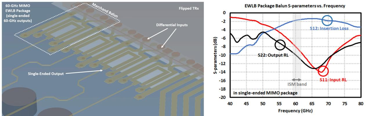
Figure 5.53: Return loss and insertion loss of Marchand balun in 60-GHz MIMO EWL B package.
