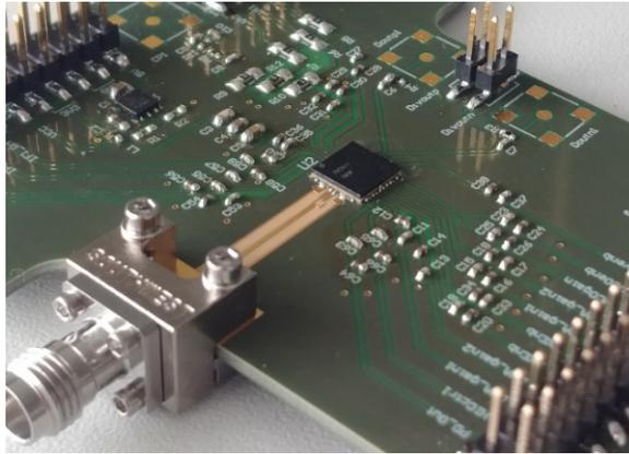
Figure 5.48: 60-GHz TRM 6 x 6 mm<sup>2</sup> LGA package mounted on the designed evaluation board.
