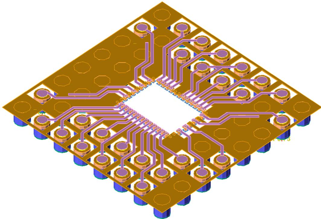
Figure 5.61: Simulated 60-GHz TR2 4 x 4 mm<sup>2</sup> IPR package structure with single-ended 60-GHz outputs.
