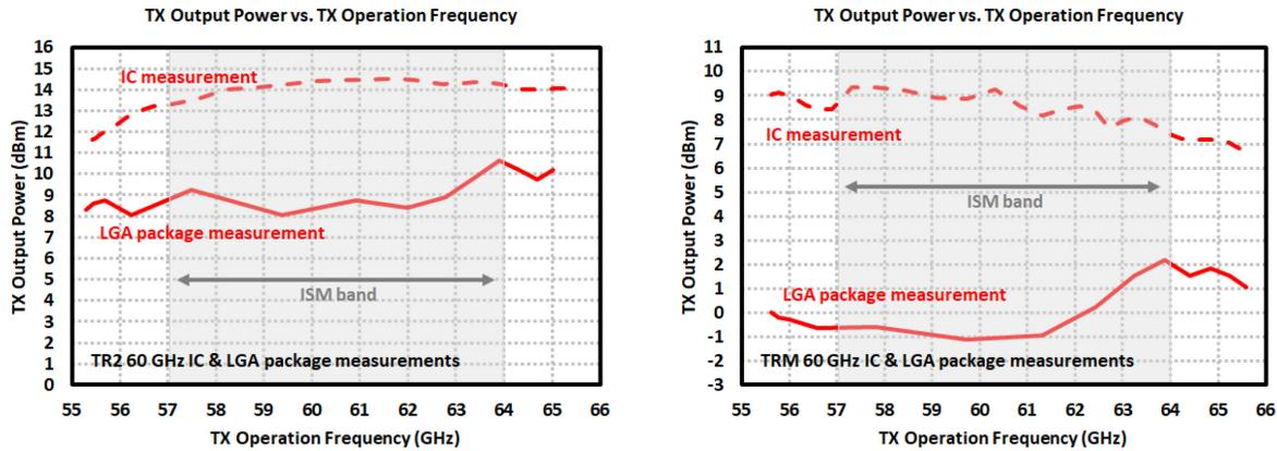
Figure 5.51: Measurement results of Tx output power in LGA packages of (*left*) 60-GHz TR2 and (*right*) 60-GHz TRM chips in comparison to their bare-die performances.
