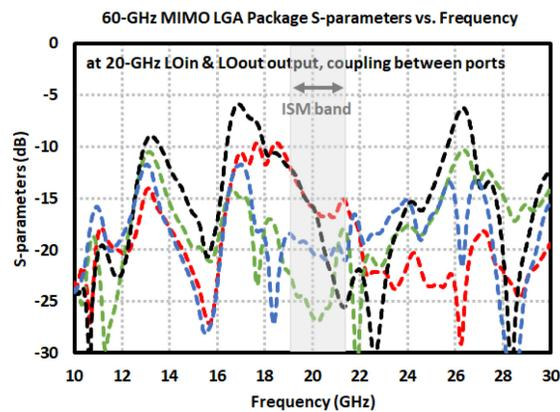
Figure 5.46: Coupling between 20-GHz  $LO_{in}$  and  $LO_{out}$  outputs of 60-GHz MIMO LGA package.
