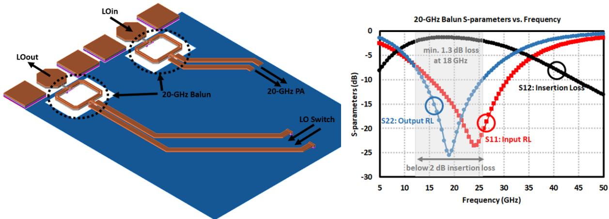
Figure 3.68: Layout and simulation results of 20-GHz balun at *LOin* and *LOout* pads in 60-GHz MIMO LO chain.
