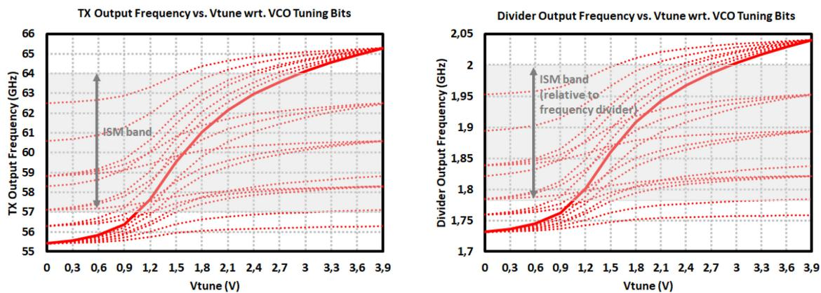
Figure 4.2: Measurement results of the 60-GHz TR2 TRx: (*left*) Tx output frequency and (*right*) Frequency Divider output frequency vs. VCO tuning voltages with respect to VCO tuning bits.
