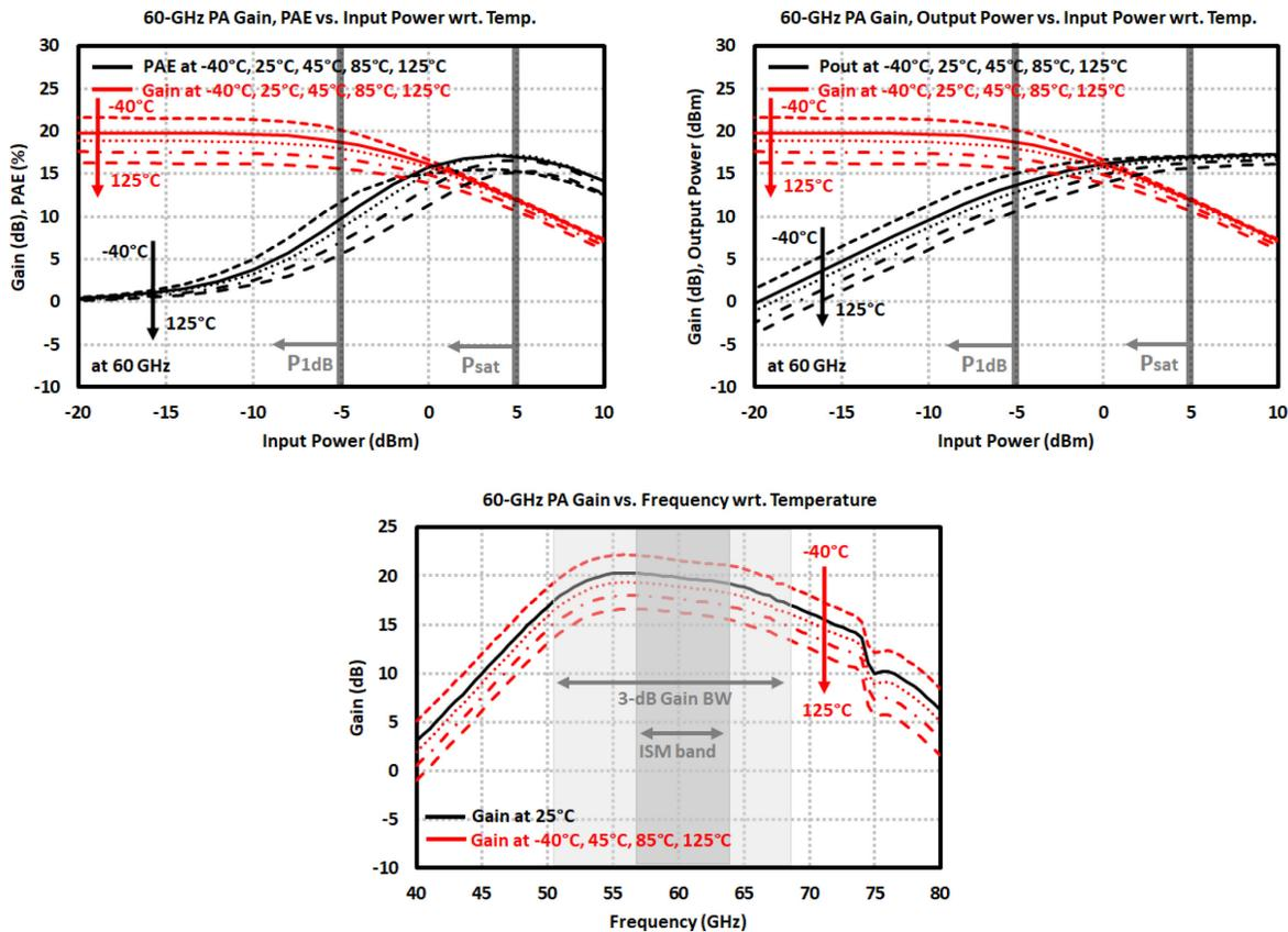
Figure 3.28: Simulation results of 60-GHz PA: (top left) gain and PAE at 60 GHz with respect to temperature, (top right) gain and output power at 60 GHz with respect to temperature, (bottom) gain with respect to temperature.
