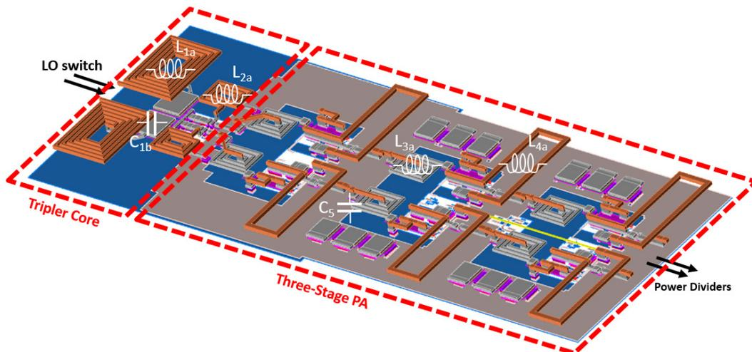
Figure 3.49: Layout of 60-GHz frequency tripler.
