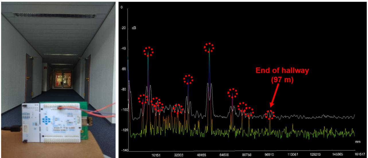
Figure 6.11: Complex indoor measurement using the radar board of 122-GHz TRM including the lens with the farthest available target being the metallic door at 97 m [16].
