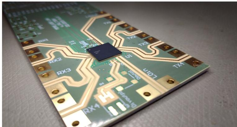
Figure 5.50: 60-GHz MIMO 10 x 10 mm<sup>2</sup> LGA package mounted on the designed evaluation board.
