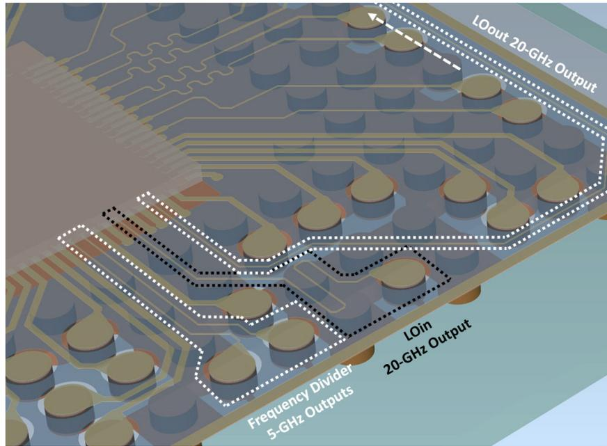
Figure 5.56: Simulated 5-GHz divider and 20-GHz  $LO_{in}$  /  $LO_{out}$  outputs in EWLB package structure.
