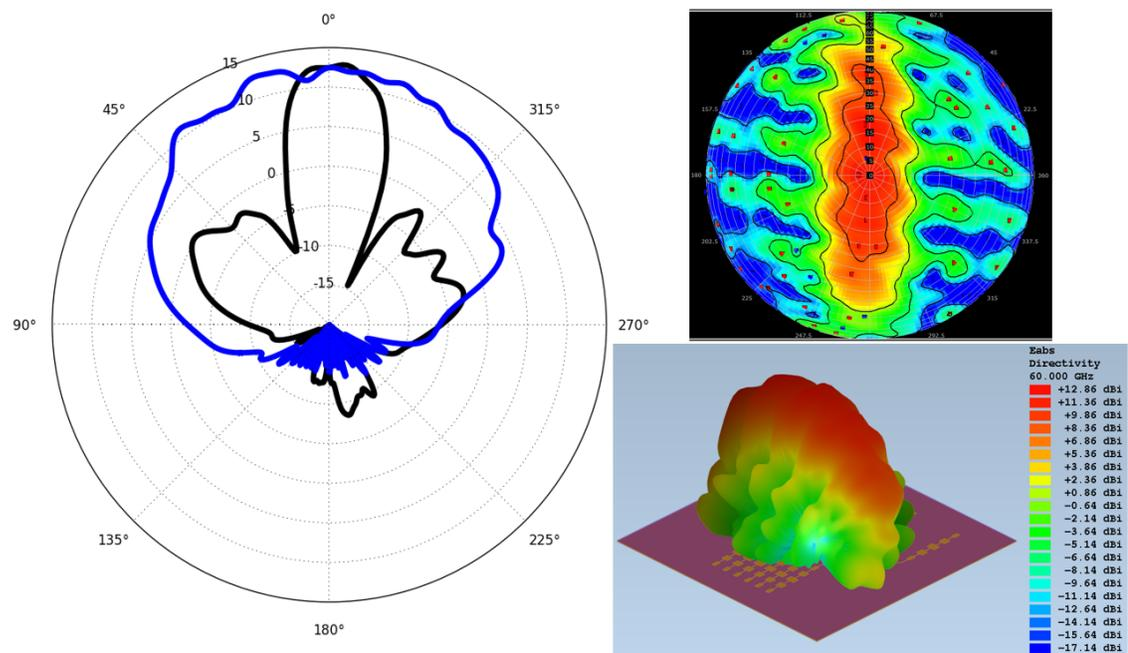
Figure 5.17: Simulation results of PCB antenna (1 x 5 patch array) of 60-GHz MIMO chip (Tx1 is excited).
