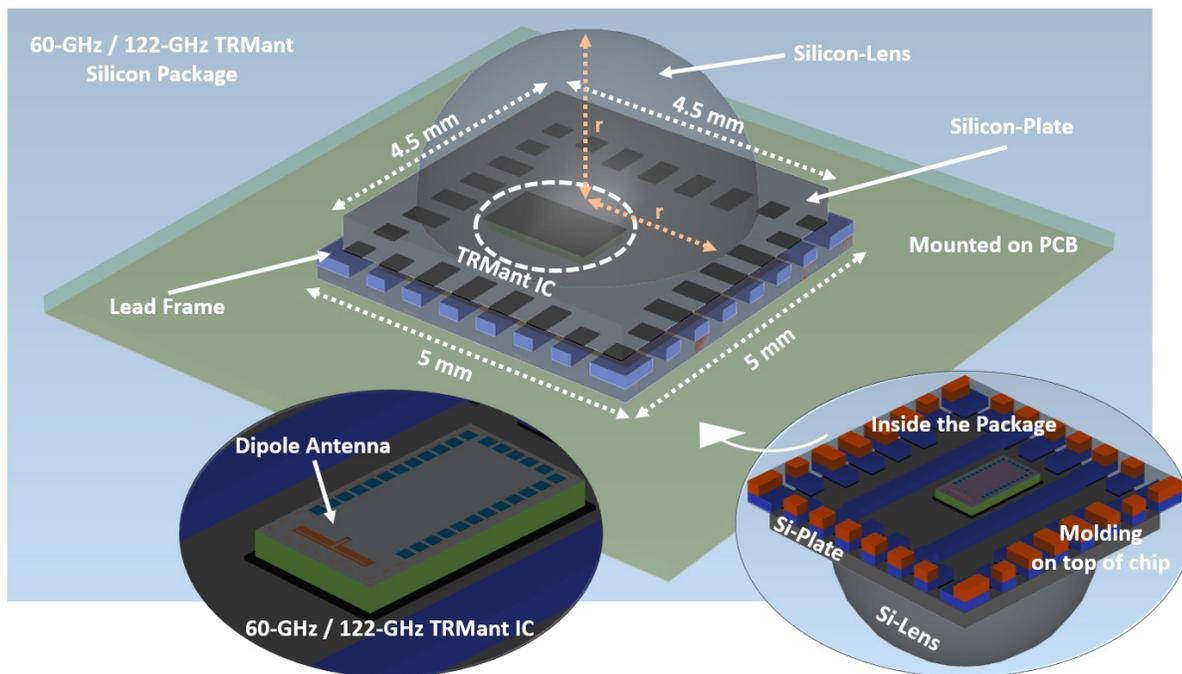
Figure 5.24: 60- / 122-GHz TRMant, 5 x 5 mm<sup>2</sup> Silicon package and antenna.
