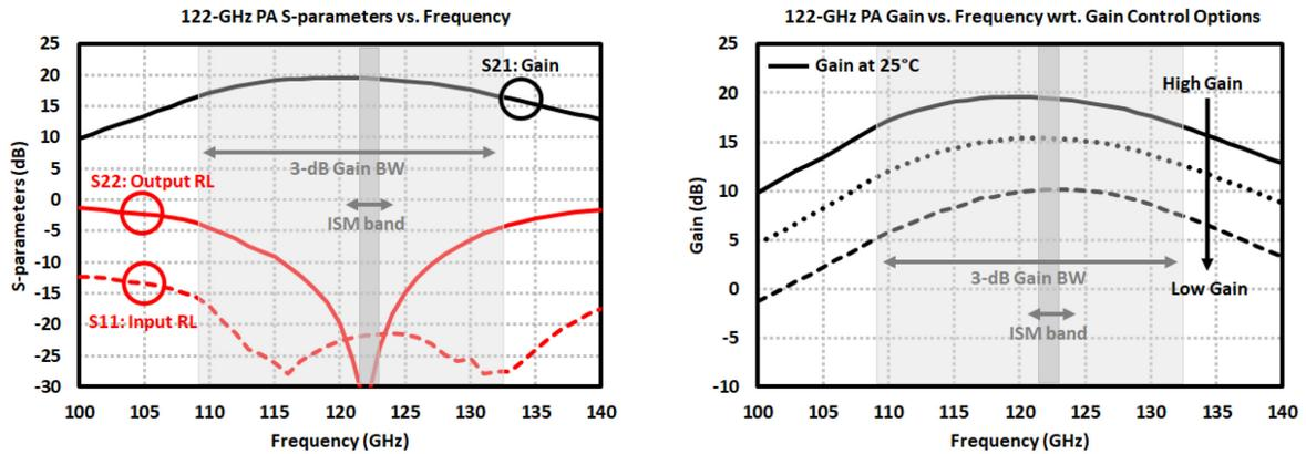
Figure 3.29: Simulation results of 122-GHz PA: (left) S-parameters, (right) gain with respect to gain control options.
