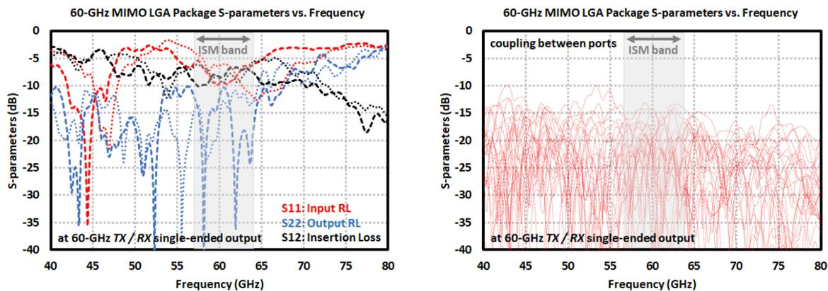
Figure 5.47: Return loss, insertion loss and port coupling of 60-GHz Tx / Rx outputs of 60-GHz MIMO LGA package.
