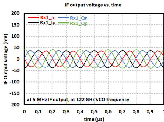
Figure 4.17: Measurement results of the 122-GHz TR2 TRx: 5-MHz IF output voltages at 122 GHz.
