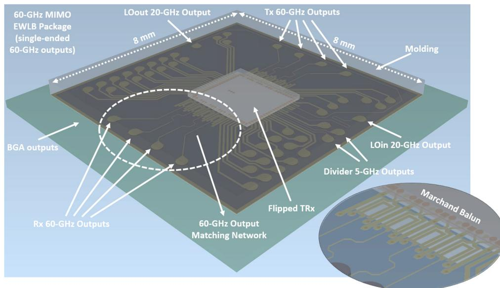
Figure 5.54: Simulated 60-GHz MIMO  $8 \times 8 \text{ mm}^2$  EWL B package structure with single-ended 60-GHz outputs.
