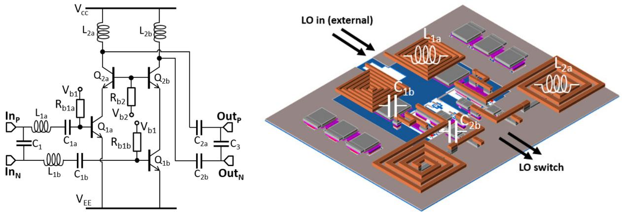
Figure 3.55: Schematic and layout of 20-GHz single-stage cascode PA.
