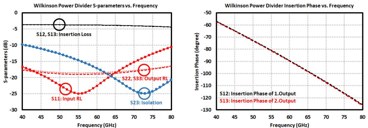
Figure 3.10: Simulation results of 60 GHz differential LC Wilkinson Power Divider: (left) S-parameters, (right) insertion phase at the divider outputs.
