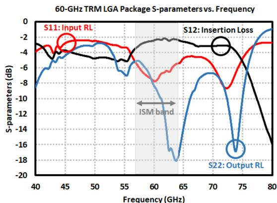
Figure 5.40: Return loss and insertion loss of 60-GHz TRM LGA package.
