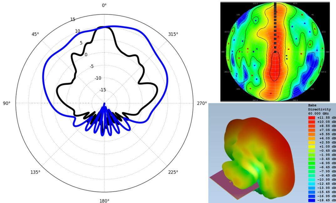
Figure 5.10: Simulation results of PCB antenna (1 x 5 patch array) of 60-GHz TR2 chip.
