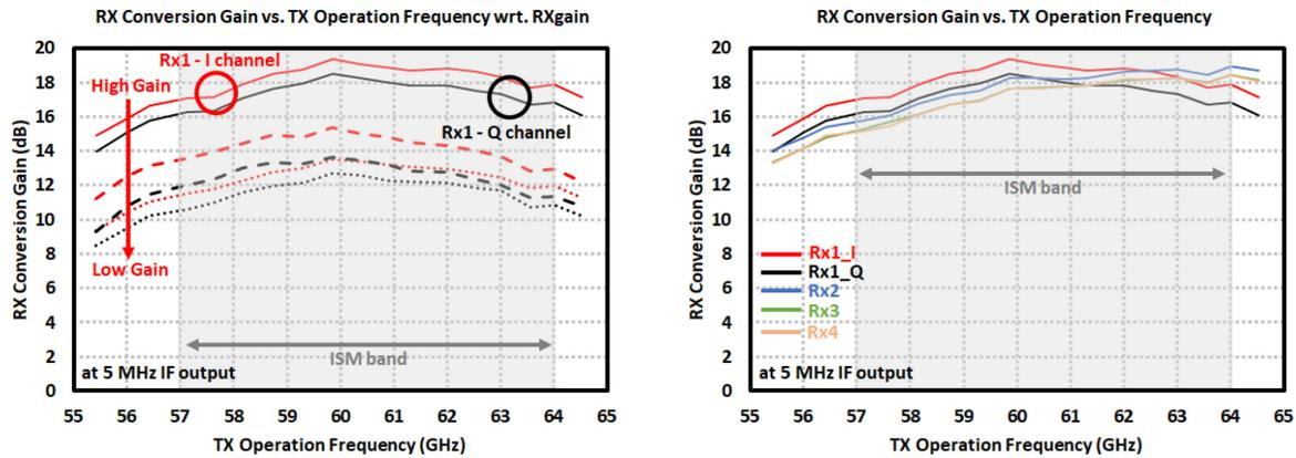
Figure 4.35: Measurement results of the 60-GHz MIMO TR<sub>x</sub> in *master* mode where internal VCO is enabled: (left) Rx channel 1 conv. gain vs. freq. with respect to Rx gain control voltages, and (right) Rx channel conv. gain vs. freq.
