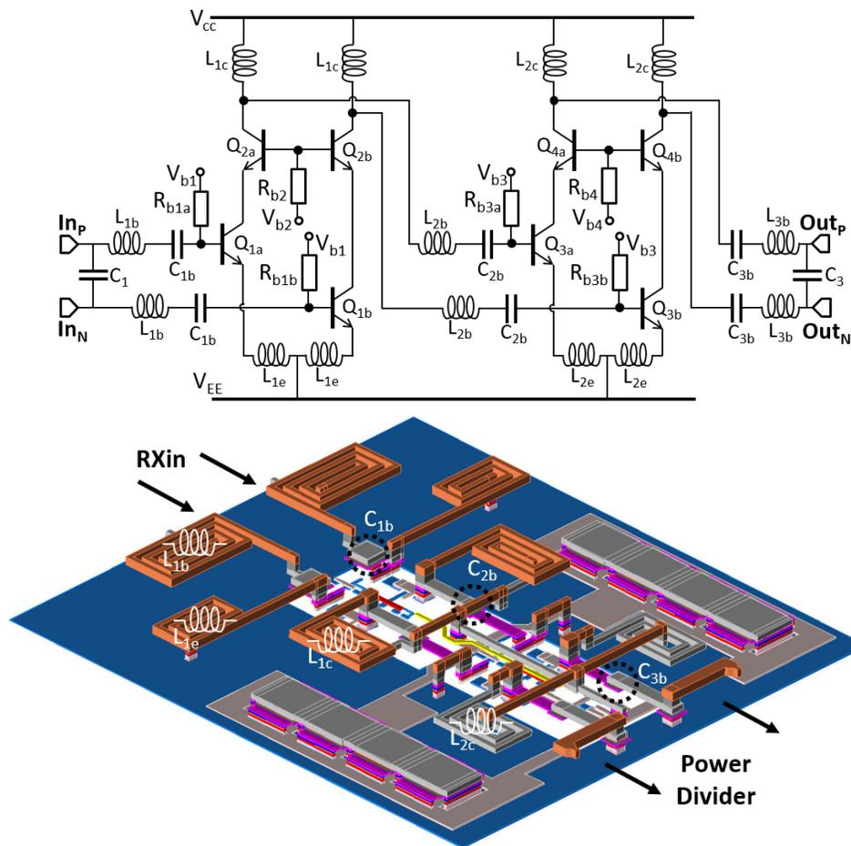
Figure 3.6: Schematic and layout of 60 GHz differential two-stage cascode LNA circuit.
