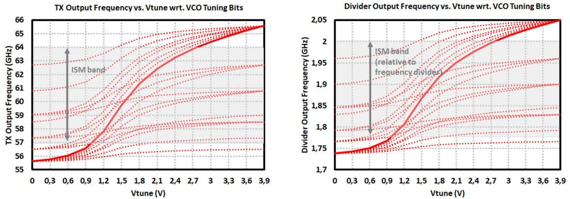
Figure 4.19: Measurement results of the 60-GHz TRM TRx: (left) Tx output frequency and (right) Frequency Divider output frequency vs. VCO tuning voltages with respect to VCO tuning bits.
