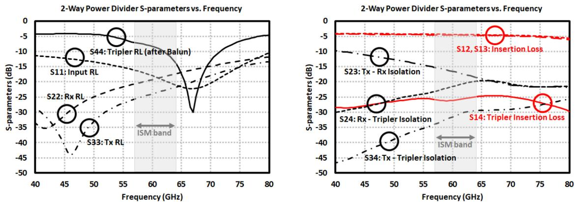
Figure 3.59: Simulation results of 60-GHz two-way power divider with a coupled output for frequency tripler.
