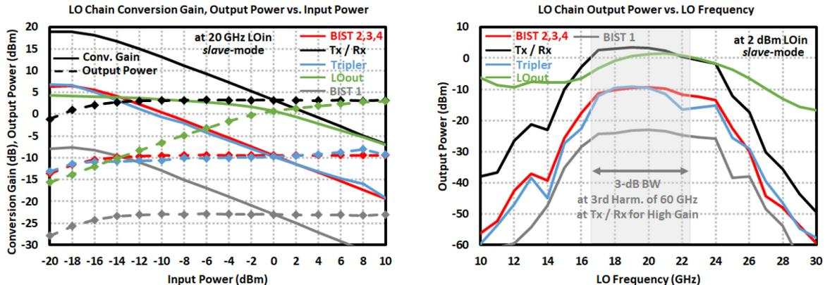
Figure 3.69: Simulation results of the complete LO chain in 60-GHz MIMO TRx in *slave* mode where internal VCO is disabled: (*left*) conversion gain and output power vs. input power at 20 GHz external LO input, (*right*) output power vs. LO input frequency at 2 dBm external LO input.
