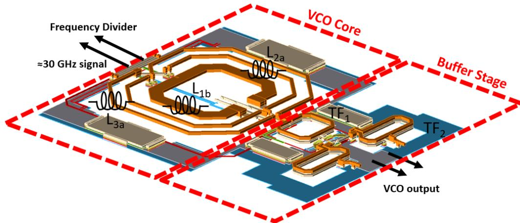
Figure 3.37: Layout of 60 GHz VCO integrated to the single-stage buffer PA.
