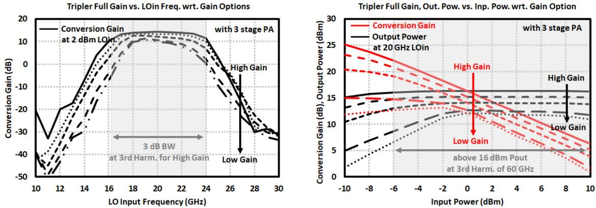
Figure 3.54: Simulation results of frequency tripler including the three-stage PA. Conversion gain and output power with respect to input power for the 3<sup>rd</sup> harmonic of 20 GHz LO input at different temperatures.
