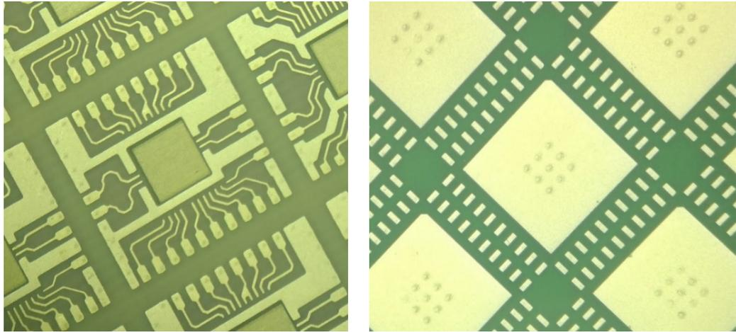
Figure 5.36: 60-GHz TRM 6 x 6 mm<sup>2</sup> LGA package, top (RF and DC connections) and bottom (lead frame).
