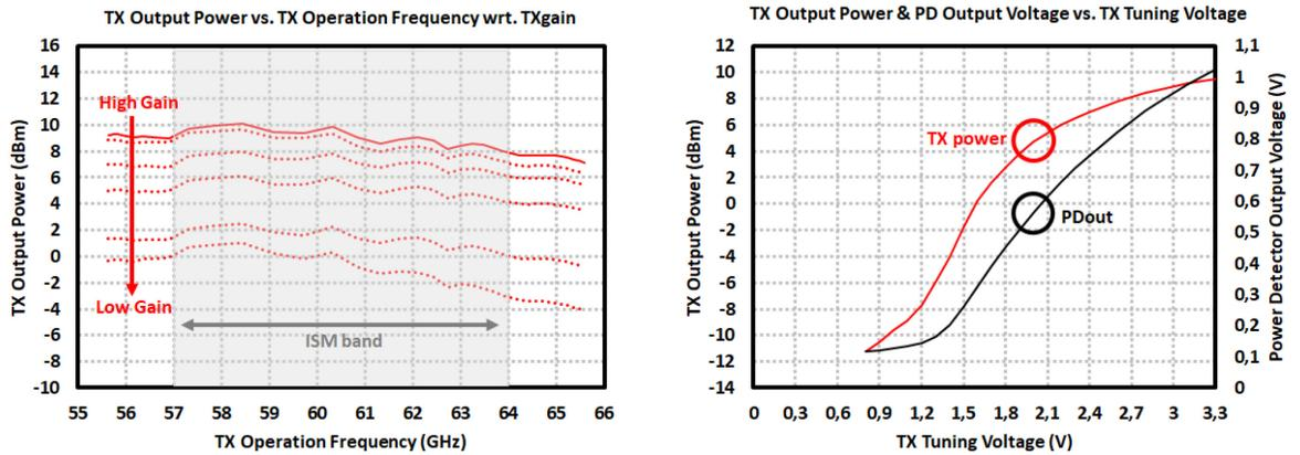
Figure 4.24: Measurement results of the 60-GHz TRM TRx: (left) Tx output power vs. frequency with respect to Tx gain control voltages 0 V – 3.3 V, (right) Tx output power and Power Detector voltage vs. Tx gain tuning voltages.
