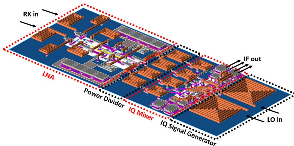
Figure 3.17: Layout of 60 GHz Rx channel highlighting the sub-blocks ( $450 \mu\text{m} \times 250 \mu\text{m}$ ).
