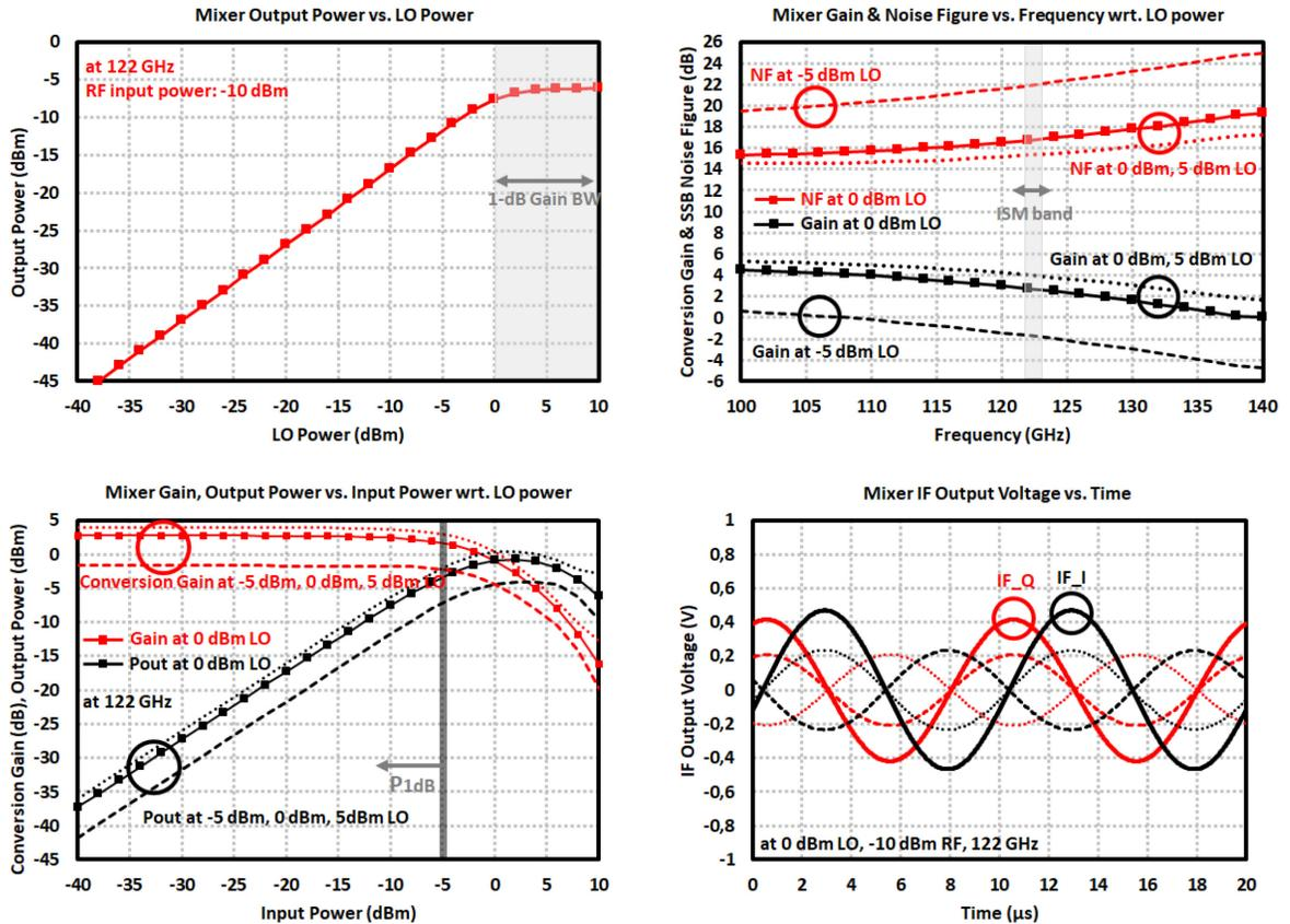
Figure 3.16: Simulation results of 122 GHz Mixer chain: (*top left*) output power vs. LO power, (*top right*) conversion gain and noise figure with respect to LO power, (*bottom left*) conversion gain and output power with respect to LO power, (*bottom right*) IF output voltages in time domain.
