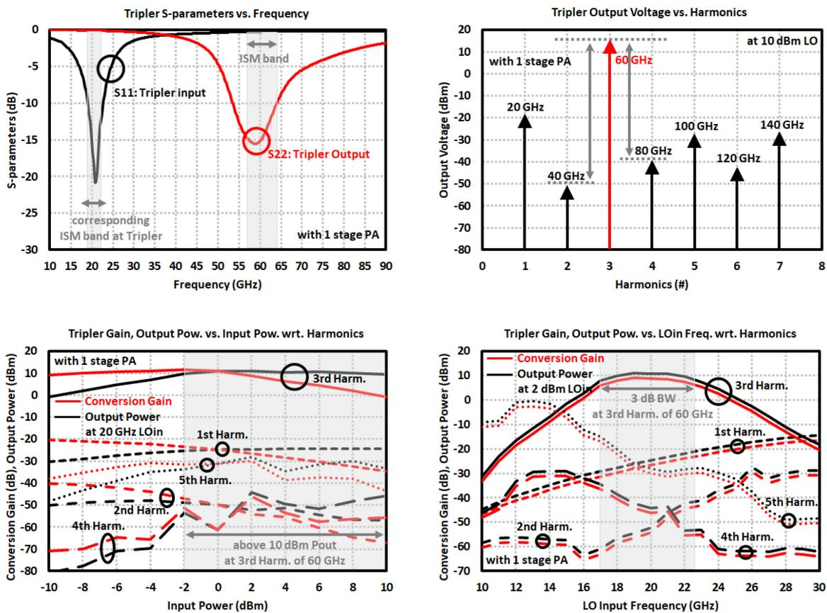
Figure 3.51: Simulation results of frequency tripler including a single-stage PA. (top left) S-parameters, (top right) harmonics at 10 dBm LO input at 20 GHz, (bottom left) conversion gain and output power with respect to input power for harmonics of 20 GHz LO input, (bottom right) conversion gain and output power with respect to LO input frequency for harmonics of 2 dBm 20 GHz LO input.
