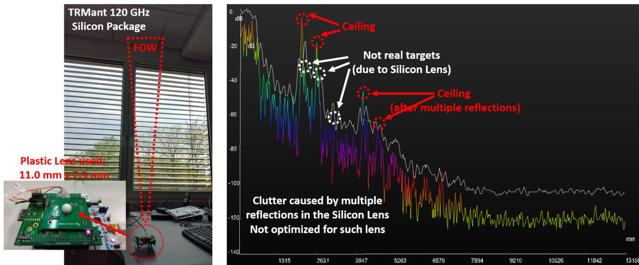
Figure 5.29: Simple indoor measurement using the radar board of 122-GHz TRMant Silicon package including the Plastic lens having 11.0 mm x 7.5 mm size directed towards the office ceiling.
