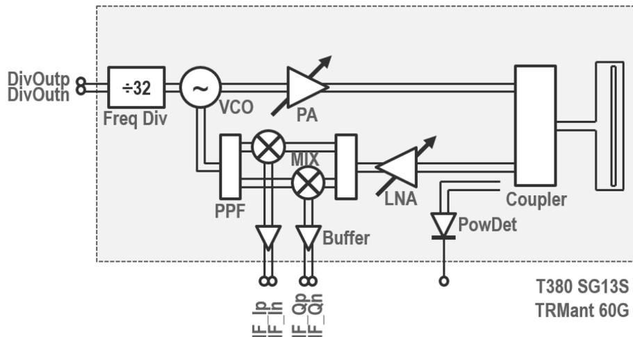
Figure 2.4: Block diagram of the single-channel monostatic 60-GHz TRx with integrated dipole antenna.
