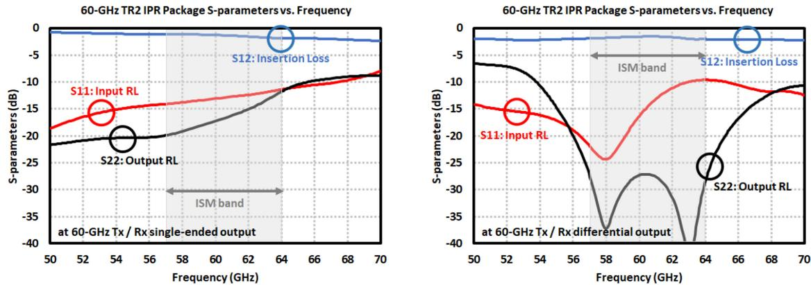
Figure 5.62: S-parameter results of 60-GHz outputs in (*left*) single-ended and (*right*) differential IPR package versions.
