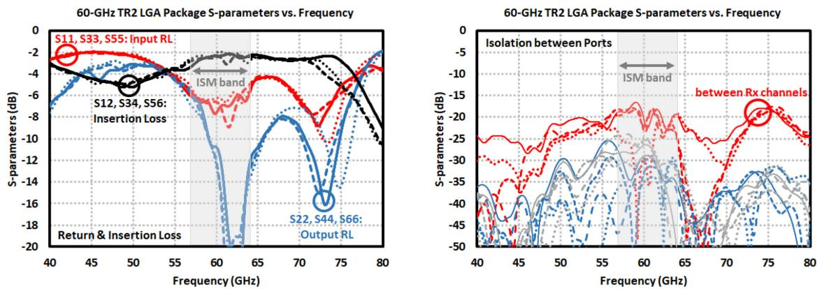
Figure 5.42: Return loss, insertion loss and port isolation of 60-GHz TR2 LGA package.
