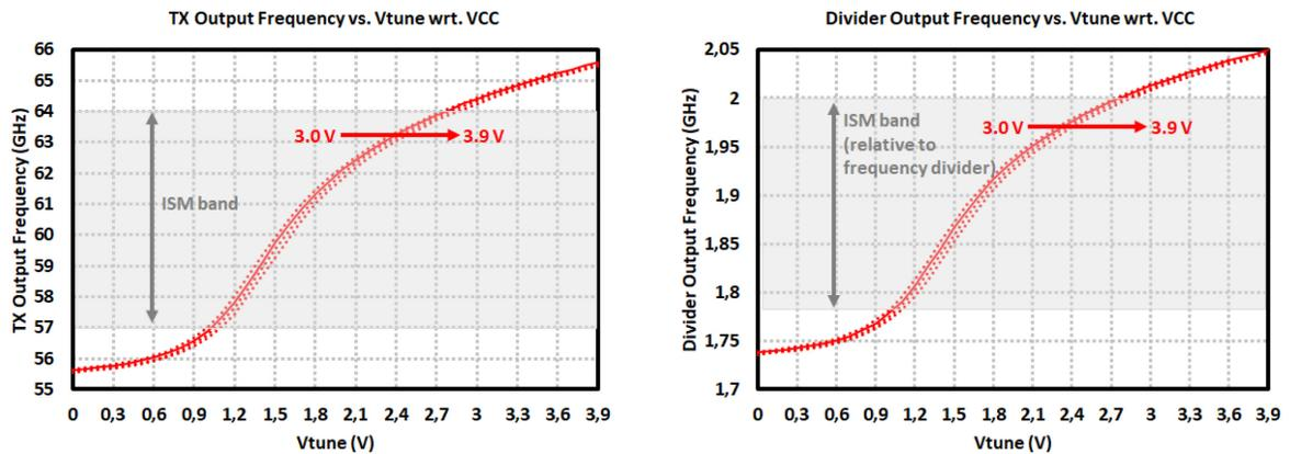
Figure 4.20: Measurement results of the 60-GHz TRM TRx: (left) Tx output frequency and (right) Frequency Divider output frequency vs. VCO tuning voltages with respect to changing supply voltages between 3.0 V – 3.9 V.
