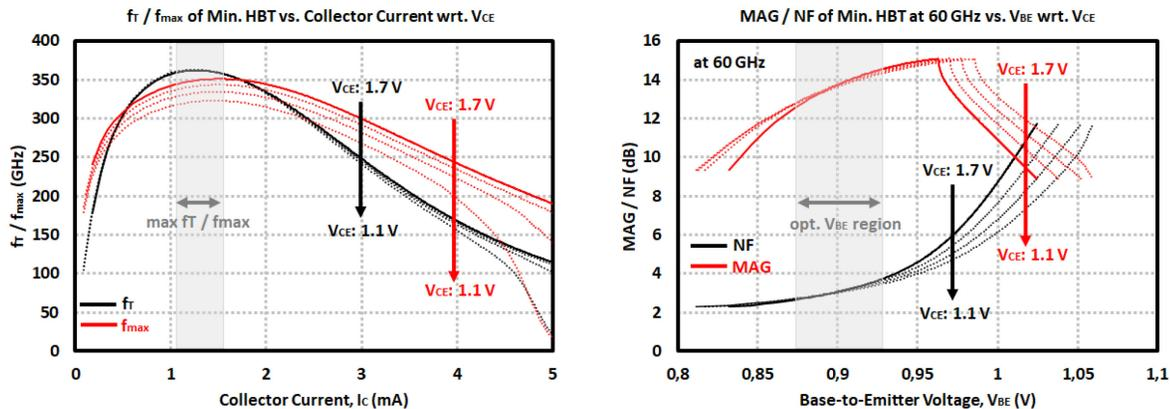
Figure 3.2: (Left) Minimum-length HBT transistor  $f_T / f_{max}$  and (right) corresponding maximum available gain and noise figure with respect to base-to-emitter voltage at 60-GHz.
