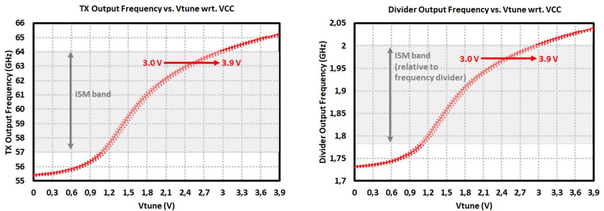
Figure 4.3: Measurement results of the 60-GHz TR2 TRx: (left) Tx output frequency and (right) Frequency Divider output frequency vs. VCO tuning voltages with respect to changing supply voltages between 3.0 V – 3.9 V.
