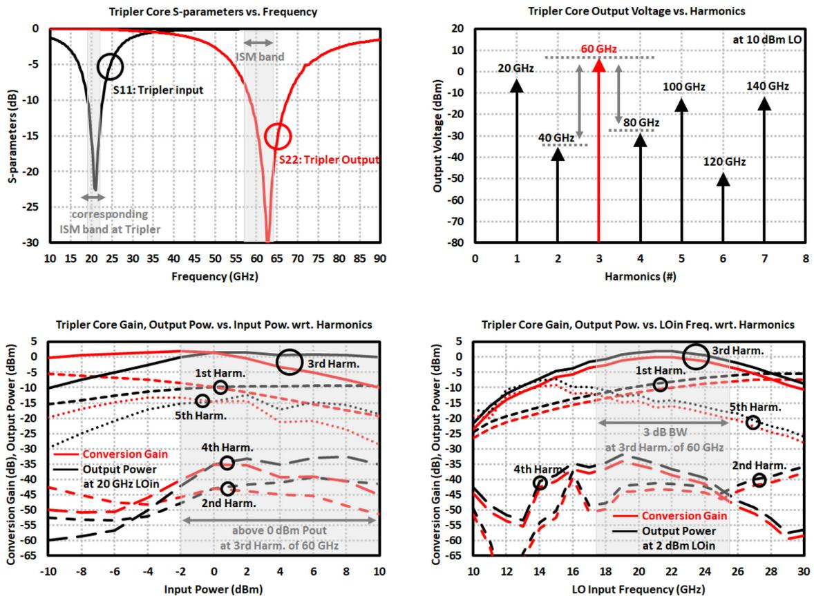
Figure 3.50: Simulation results of frequency tripler core. (*top left*) S-parameters, (*top right*) harmonics at 10 dBm LO input at 20 GHz, (*bottom left*) conversion gain and output power with respect to input power for harmonics of 20 GHz LO input, (*bottom right*) conversion gain and output power with respect to LO input frequency for harmonics of 2 dBm 20 GHz LO input.
