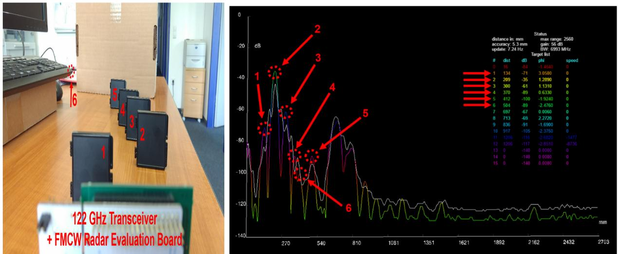
Figure 6.10: Simple indoor measurement using the radar board of 122-GHz TRM including the lens to detect closely spaced targets [15].
