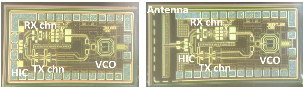
Figure 4.18: Photo of the fabricated 60-GHz TRM and TRMant transceiver chips occupying  $1.42 \text{ mm} \times 0.84 \text{ mm}$  and  $1.64 \text{ mm} \times 0.84 \text{ mm}$  area.
