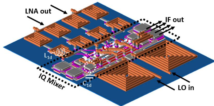
Figure 3.14: Layout of 60 GHz double-balanced Gilbert-cell based quadrature mixer.
