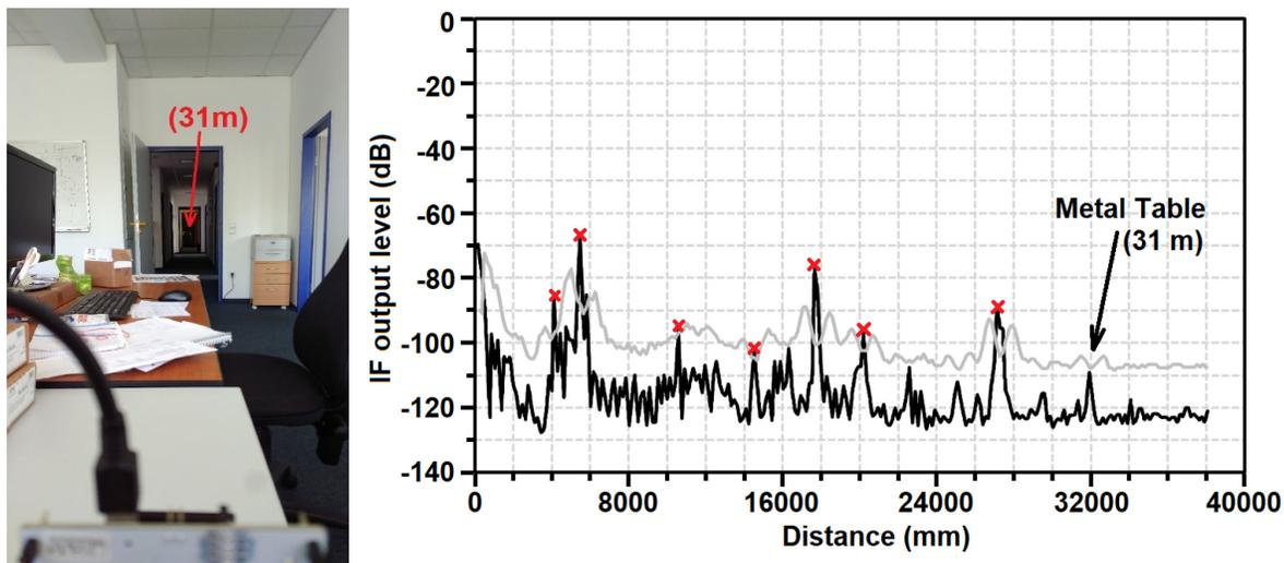
Figure 6.6: Complex indoor measurement using the radar board of 60-GHz TRM excluding the lens with the farthest available target being the metallic table at 31 m (below the detection threshold, needs threshold adjustment) [18].
