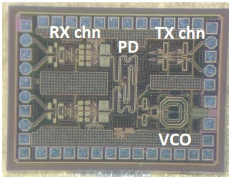
Figure 4.1: Photo of the fabricated 60-GHz TR2 transceiver chip occupying  $1.46 \text{ mm} \times 1.06 \text{ mm}$  area.
