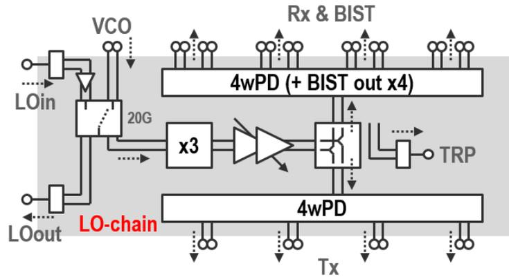
Figure 3.66: Schematic of the complete LO chain in 60-GHz MIMO TRx.
