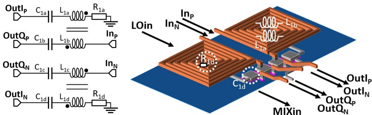
Figure 3.11: Schematic and layout of 60 GHz differential I/Q signal generator.
