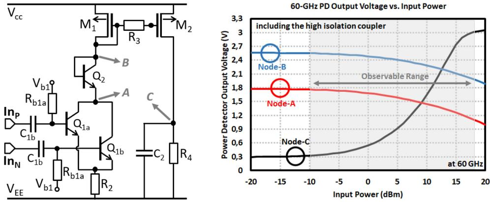
Figure 3.33: Schematic and simulation results of power detector together with high isolation coupler in 60-GHz TRM.
