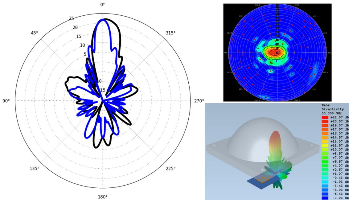
Figure 5.7: Simulation results of PCB antenna of 60-GHz TRM chip including HDPE plastic lens at 1.5 cm.
