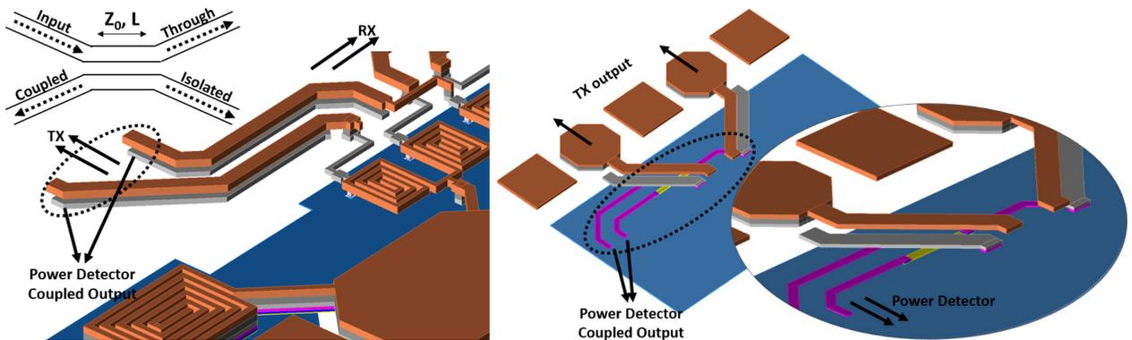
Figure 3.32: Layout of power detector coupler mechanism integrated to (left) high isolation coupler in mono-static TRxs and (right) Tx output pads in 60-GHz MIMO TRx.
