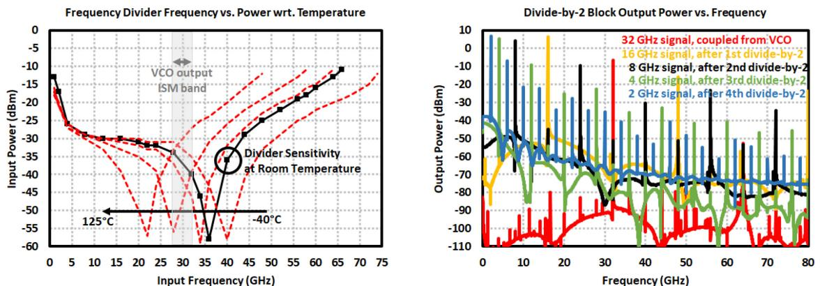
Figure 3.45: (*Left*) Divide-by-16 frequency divider sensitivity measure with respect to temperature, (*Right*) Divide-by-2 frequency divider block output power spectrum at each division stage.
