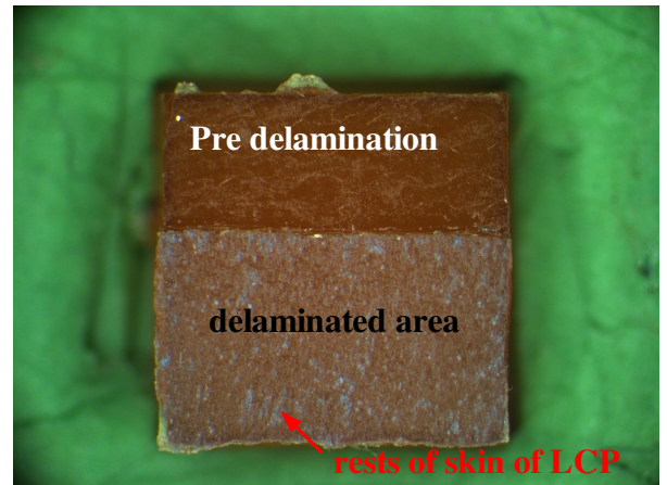
(b) Button with rests of skin of LCP substrated on delaminated area
