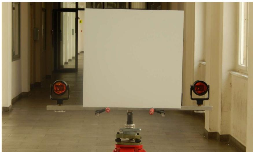
**Figure 4.** Mount with planar sample.
